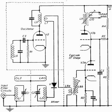
Fig. 1.—Circuit diagram of the converter.
