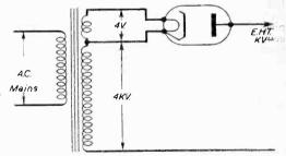
Fig. 29.-Mains driven EHT (negative supply).
