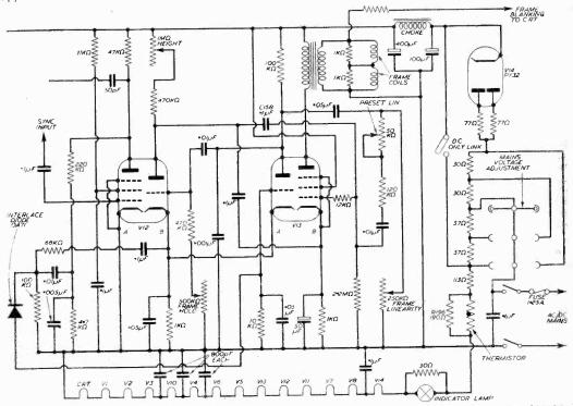
Fig. 2.—Mains, H.T. and frame timebase circuit. Thermistor is a Brimistor CZ8A or a Varite VA1026.
