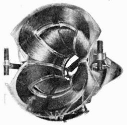
This 110° scanning coil assembly by Elac incorporates a new Ferroxcube core enabling a "pull-back" of 4mm, to be achieved without loss of sensitivity.
