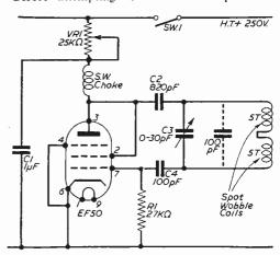
Fig. 3.—Circuit of the oscillator using an EF50.
