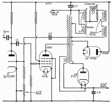
Fig. 26.—Circuit for line flyback EHT.
