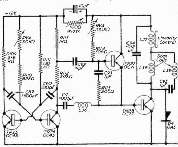
Fig. 24.—The line timebase.
