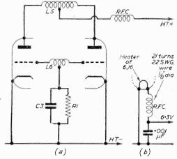
Fig. 2(a) (Left)-Tuned-anode, tuned-grid oscillator circuit.
