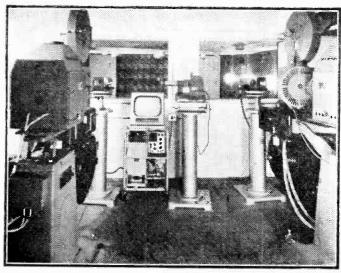
The projection room of L.P.E. Television Ltd., with two Marconi BD871 television cameras mounted on pedestals for televine work. (See "Closed Circuit Television".)
