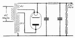
Fig. 28.—Mains driven EHT (positive supply).
