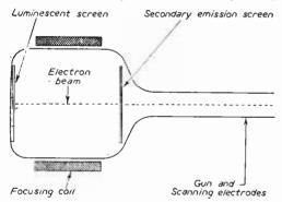
The secondary emission cathode ray tube.
