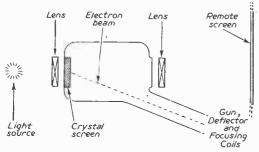
Basic details of a light relay C.R. tube.
