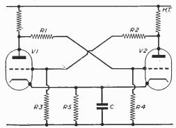
Fig. 1.-Stable multivibrator circuit.
