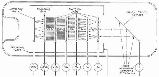
A pictorial representation of a grid cell multiplier.
