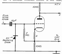
Fig. 2.—Cathode follower for use with grid modulation of C.R.T.
