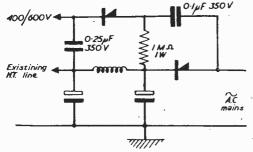
Picture tube substitution. A voltage additive arrangement,
