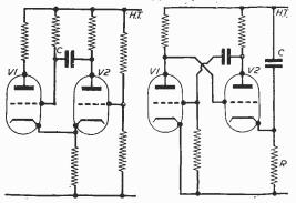
Fig. 2.—(Left) The "flip-flop" circuit.
