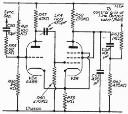
Fig. 2.—Circuit diagram of the line timebase generator.
