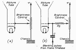
Fig. 3.—In most older receivers the brightness control is arranged as in circuit (a), but where frame-flyback suppression is featured, in more recent models, the circuit in (b) is often used.
