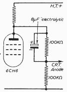
Fig. 1.—Reducing the D.C. voltage on the C.R.T. cathode.
