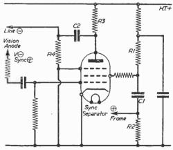
Fig. 18.—Taking off the frame pulses from the screen
