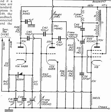
Fig. 1.—Circuit diagram of the frame timebase and interlace filter of the Cossor 927 series.
