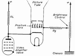
Fig. 2.—A diagram showing the biasing elements of a picture tube. In a "soft" tube the positive ions will be attracted to and collect on the grid as shown, and the positive charge on the grid will draw grid current through Rg, which will then act as a load resistor.
