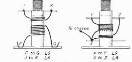
The supplementary coil data for the R.F. 26 converter.
