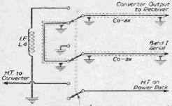
Bandswitch (In Converter Off position)
