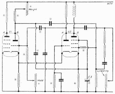
Fig. 4.—Multivibrator using two triode pentodes, two triodes as multivibrators, one pentode as sync. valve, one pentode frame output valve.
