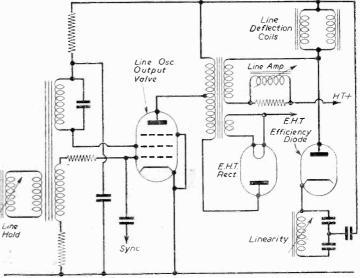
Fig. 8 .- A line timebase stage utilising a self-oscillating output stage.
