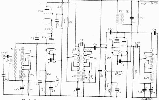
Fig. 1.-The tuner section of the completed receiver. This is the heart of the set.
