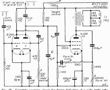
Fig. 23.—Complete scanning circuit for frame deflection of a wide-angle tube. Resistors are  $\frac{1}{2}$  w. unless stated otherwise.
