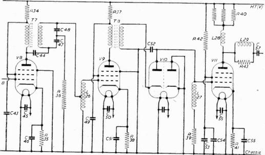
Fig. 3.-The vision I.F. section of the receiver.
