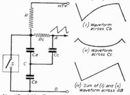
Figs. 17 and 18 .- Sawtooth linearising circuit and waveforms found in it.
