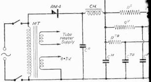
Fig. 4.-The power pack section.
