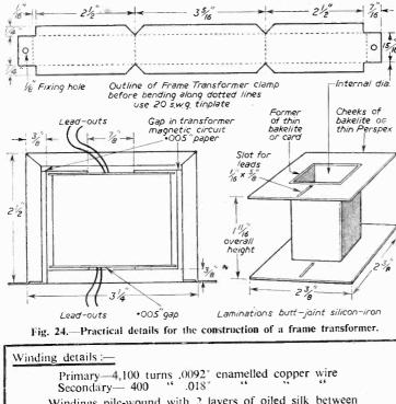
Windings pile-wound with 2 layers of oiled silk between prim. & sec. and also over completed winding
