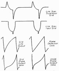
Fig. 4 .- Some typical waveforms from the timebases.
