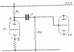
Fig 2 -- Testing at the valveholder in a receiver.
