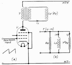
Fig. 19.-Simplified circuit of frame scanner, and its equivalent circuit.
