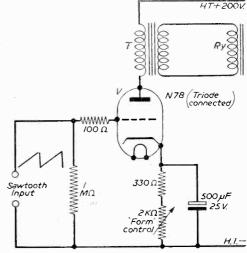
Fig. 21 .- Practical circuit of valve curvature linearity correction.
