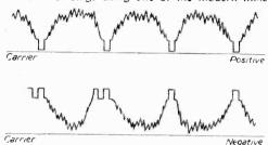
Fig. 3.—Positive and negative modulation.
