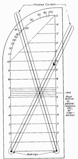
Fig. 5,-The finished calculator.
