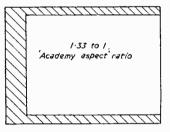
Fig. 1,-Shaded area indicates section of old silent film frame which is not reproduced on television. "Academy" area is fully reproduced.
