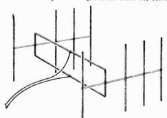
Fig. 18.-A Yagi array with slot aerial.
