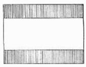
Fig. 2.—Shape of CinemaScope 2.35 to 1 picture on TV screen, reproducing full width, but masking top and bottom.
