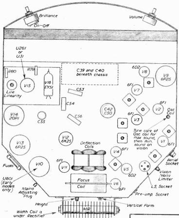
Fig. 3.—Top of chassis view.
