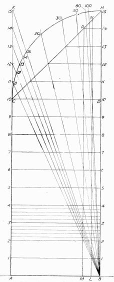
Fig. 4.—Laying out the basic scale.
