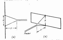
Fig. 17.—On the left a delta match, and on the right a delta applied to a slot.
