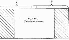
ped off with black Fig. 3.—When reproduced to the full height of the TV screen, each side of CinemaScope picture is cropped (in section shaded above). This restricts the choice of CinemaScope film sequences for TV to those with main action in the centre. A.-TV's new scanning system permits a panoramic shift from "A" to "B" to follow the main action.
