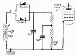
Fig. 6.—A switched detector stage.
