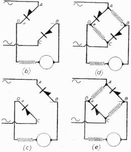
Fig 1 (b) to (e). How the hridge rectifier works.
