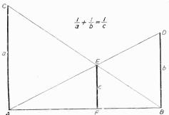
Fig. 1.—The basic principle of the calculator. See also Note 1 (page 309).
