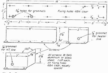
Fig .5.—Common chassis side drilling, and details of underchassis screens.
