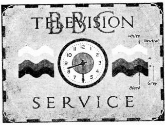
Fig. 3.—Details of the tuning signal.
