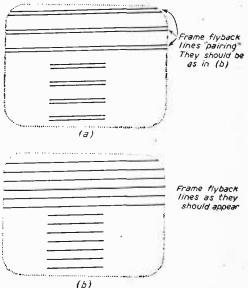
Note: (a) and (b) are the conditions obtained when the brilliance control is advanced while receiving a picture
