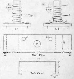
Figs. 2 and 3.-Coil-winding details and chassis data.
