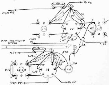
Fig. 9.—Layout of V2 and V8 stages. This gives the general layout of all vision stages.
