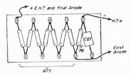
Fig. 10.—Bleeder and first anode boost resistance panel details.
