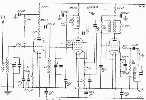
Fig. 10.—Circuit of a superhet converter.
