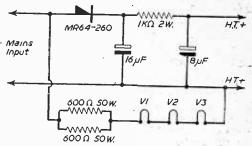
Fig. 12.—Modified circuit for A.C./D.C. use.
