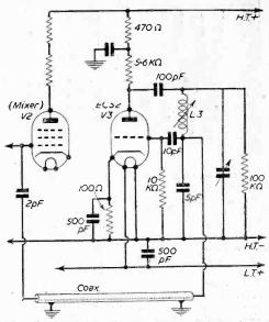
Fig. 13.-Modified oscillator stage. 5 turns 22 s.w.g. on §in. former with iron slug for channels 1 and 2; no slug for channel 3 and brass slug for channels 4 and 5.
