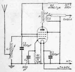
Fig. 1.—Theoretical circuit of the Pre-amplifier.
