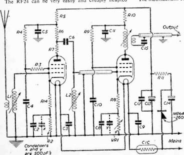
Fig. 8.—Circuit of the two-stage pre-amplifier.
