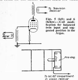
If the bandwidth is found insufficient it can be broadened by connecting a 4.7  $K\Omega$  resistor across L1 and another across the primary of L2.
