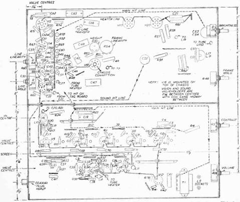
Fig. 6.—Underchassis layout of valves and components, showing run of heaters and H.T. lines. This layout applies to the transitron frame oscillator. The principal measurements are given, but small changes are permissible to suit alternative components, etc.
