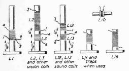
Fig. 8.-Coil winding details.
