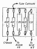
Fig. 11.—Line output transformer wiring.
