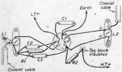
Fig. 4.—Wiring details.
