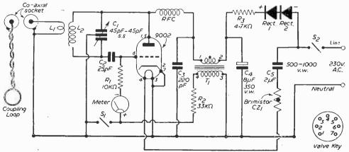
Circuit of the Grid-dip Meter and Bar Generator.
