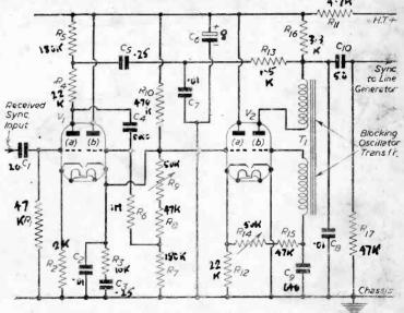
Fig. 5.—This English Electric circuit utilises two double triodes. Essential values are:
