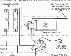
Fig. 6.—Wiring of the mains side.
