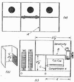
Fig. 3.—Details of the chassis modification and layout.
