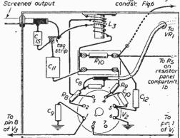
Figs. 4 and 5.—Above and below chassis wiring details.
