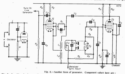
Fig. 3.—In this circuit capacitative or inductive effects are given by the relative positions of C and R.
