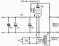
Fig. 7.—Modification when using the unit for A.C. operation only.
