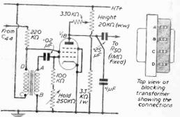
Fig. 4.—Alternative frame oscillator stage. When this circuit is used, the bias resistor of V19 is 1602.
