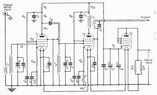
Fig. 1.-Circuit of the first A.C./D.C. Pre-amplifier.
