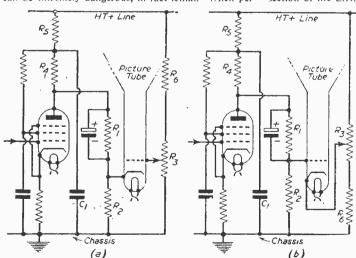
Fig. 1.—Methods of modulating the picture tube: (a) cathode modulation and (b) grid modulation.
