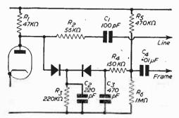
Fig. 5.—New Pye arrangement in which two rectifiers are used in place of the double diode seen in former circuits.
