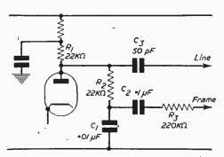
Fig. 2.—A practical interpretation of the Fig. 1 arrangement. This is the arrangement used in certain Ferguson receivers.
