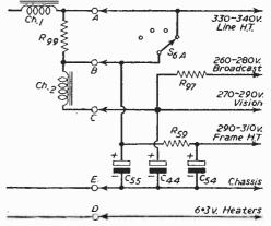
Fig. 4.—The voltage divider circuits
