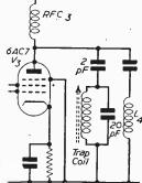
edge of this hole are filed Fig. 5.—"Sucker" trap cirfor the four mounting cuit to remove sound from bolts. The 4-volt heater the vision channel.
