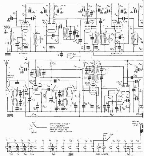
Fig. 1.-Theoretical circuit of the combined receivery exe
