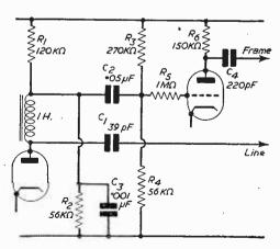
Fig. 6.—This arrangement, recommended by Mullard, uses a triode, and an iron-cored choke in place of the resistor for the anode load on line.
