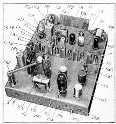
Fig. 2.—Chassis layout with essential component references.
