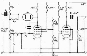
Fig. 2.—The Miller-Sanatron circuit.
