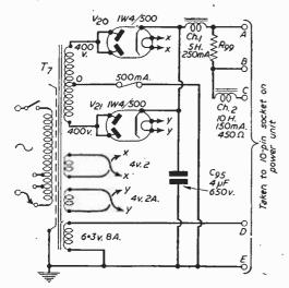
Fig. 3.-Theoretical circuit of the mains unit.
