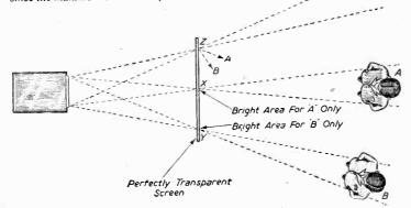
Fig. 19.-Diagram showing the function of a viewing screen.
