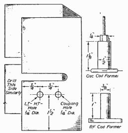
Drilling Of Inter-Compartment Screen
