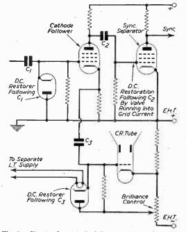
Fig. 5.—Circuit of a cathode follower video stage feeding the tube from the cathode and the sync separator from the anode.
