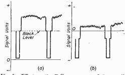
Fig. 3.—Effect on the D.C. component of the coupling condenser (a) without condenser, and (b) with condenser
