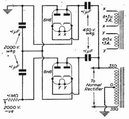
Fig. 5.-A high voltage quadrupler circuit.
