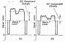
Fig. 2.-Video signal, D.C. component, and sync pulses.
