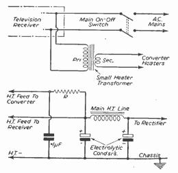
Fig. 2 (Top).—Use of additional heater transformer, and Fig. 3 (Bottom)—a decoupled H.T. feed for the converter,
