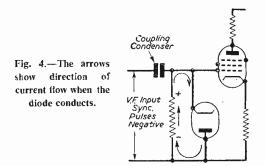
diode in each position, but it is quite possible to use a Westector type WX 6 in front of the tube grid and this dispenses with the necessity of a separate heater winding for the diode.
