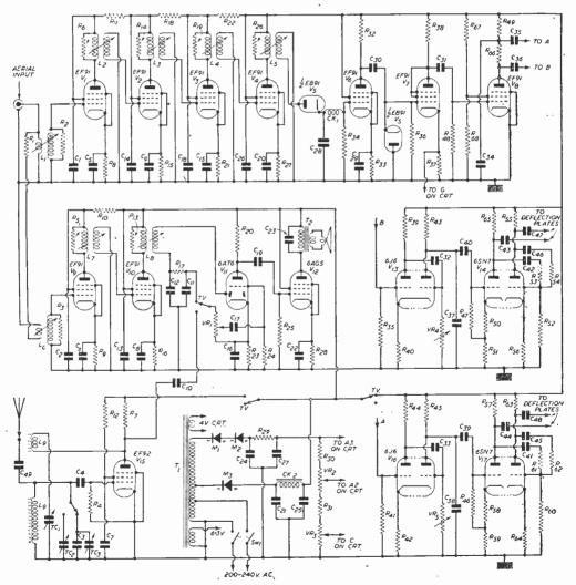
Circuit of the Completed Midget Television-radio Receiver built by the Author and illustrated on page 399. A full list of the components used in the original model will be found on page 395.
