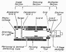
Fig. 2.-Schematic arrangement of the Image Orthicon.
