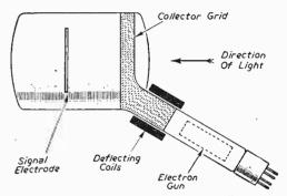
Fig. 1.--Schematic arrangement of the Iconoscope.
