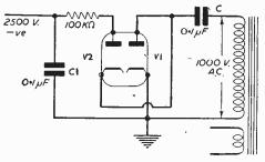
Fig. 3.-A simple doubler circuit.
