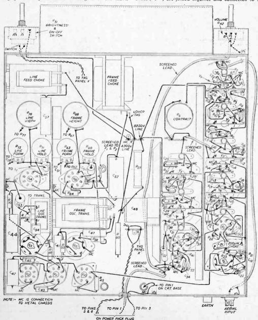
Fig. 6.-Main chassis wiring details.
