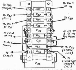
Fig. 5.—Tag board No. 4, which feeds the frame time-
