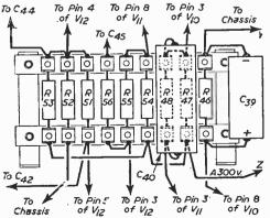
Fig. 3.—Tag board No. 2, which feeds the sync-circuits.
