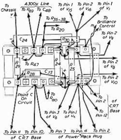
Fig. 2.—Tag board No. 1, which is the main power distribution point.
