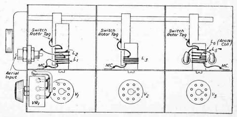
Fig. 4.—Top view, showing coil connections. The trimmers and fixed condenser have been omitted for clarity.
