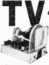
Model TV 20 inc. 12° Tube and 21 valve circuit operating on 200-250 volt A.C. mains with two main controls and SIX pre-set adjusters, completely en closed E.H.T. unit and separate 10" loudspeaker.
