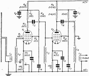
Fig. 2.—The circuit of the unit after conversion.
