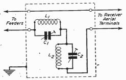
Fig. 1.—Circuit of the Wavetrap.
