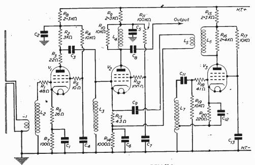
Fig. 1,-Original circuit of the RF24 Unit.
