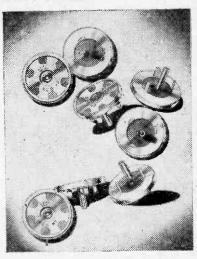
Type CM 30 Cap. in  $\mu$ F: 0.0002, 0.0003, 0.0005 Cap. Tolerance (a) -0 + 50%(b)  $\pm 20\%$ Max. D.C. Wkg. Volts 350 at 71°C.
