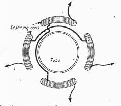
Fig. 10.—Arrangement of the scanning coils around the dissector tube.
