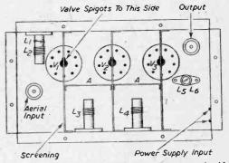
Fig. 3.-Layout of the main components-underside view.
