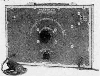
For accurate adjustments of a modern television receiver a pattern generator such as this Windsor model is invaluable. It checks raster linearity, vision receiver frequency and bandwidth, sound channel frequency, frame frequency and linearity.
