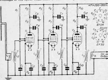
Fig. 1.-Theoretical circuit of the pre-amplifier. A list of components will be found on the next page.
