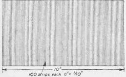
Fig. 8.—Diagram showing how the picture area is built up by the system shown in Fig. 7 (last month's issue).
