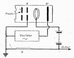
Fig. 12.-Arrangement of the electron multiplier.
