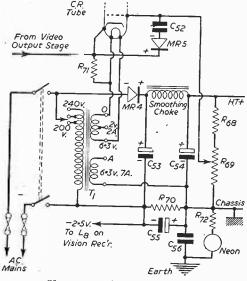
The power unit and tube supply.
