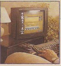
The alternative, TV PC approach to JR Smart home control. The TV set becomes a PC with an infra-red remote-control keyboard. In addition to home network operation, this gives access to the internet with the TV screen for display.
