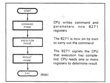
Fig. 3.6. Sequence of operations for an 8271 floppy disc controller. The CPU initiates action by sending a sequence of commands to the 8271; the 8271 then carries out the action independently, and returns the result to the CPU
