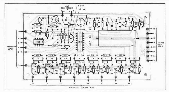
Fig. 13. Type B receiver board constructional details
