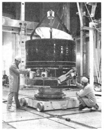
Giotto under laboratory conditions at the British Aerospace facility at Bristol. The probe is almost 3 metres high and is 1.84 metres in diameter
