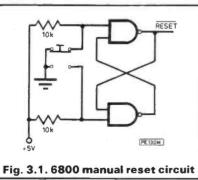
ual reset circuit for a 6800 system is shown in Fig. 3.1.
