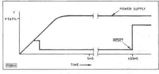
Fig. 3.3. Timing for power-on reset
