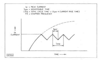
Fig. 3. Current waveform: Constant current chopper mode
