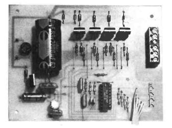
The values specified should work with most small motors, the ideal values for a particular set up can be found by experiment. It is worth noting that a stepping motor running at full power will run very hot. This is quite normal, the manufacturer's specifications allow a maximum operating temperature of 120°C.
