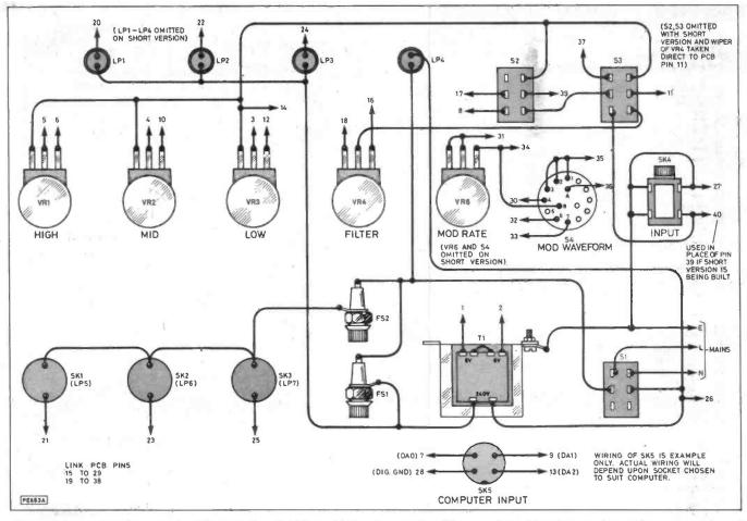
Fig. 2.3. Complete interwiring diagram for the Disco Lights Controller. The numbered lead-out wires relate to numbered lines on the main p.c.b., published in Part One, and to the optional "chaser" board. If the simplest version of this project is being built, many components can be omitted, as noted above, and the input taken direct from line 40 to the main p.c.b. In the full version, line 40 is omitted, and the input taken from line 39
