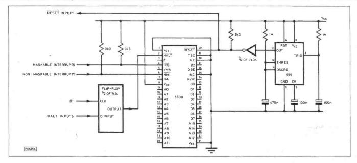
Fig. 3.2. Practical power-on reset circuit, ensuring that the micro starts up in a known state
