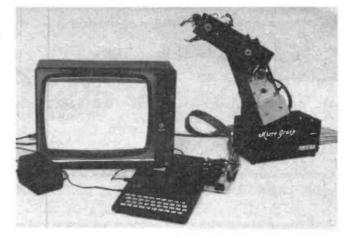
The Micrograsp robot with interface and ZX81—a very popular low-cost system introduced in Dec '82
