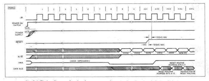
Fig. 3.4. Timing diagram showing the sequence of events after the micro is first switched on
