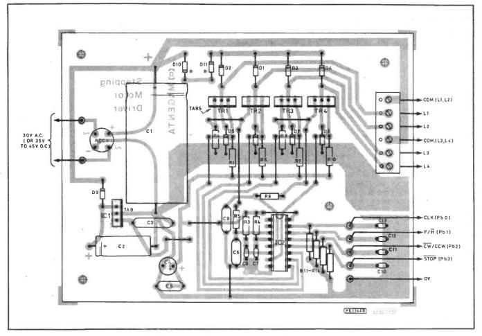
Fig. 5. Component layout of the Stepping Motor Driver
