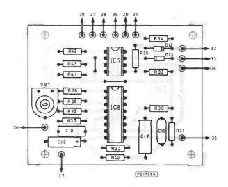
Fig. 2.2. Component layout and p.c.b. design. The offboard numbered lines refer to numbered lines on the main board, and on the interwiring diagram
