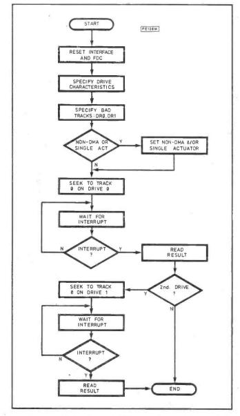
Fig. 3.7. Initialisation includes a reset to the interface hardware between FDC and CPU, and indication of whether or not this is a Direct Memory Access (DMA). The DMA facility allows the CPU to continue with other tasks while the FDC is finding the required data
