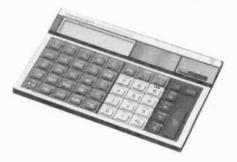
58C/59 family of calculators. The constant memory feature retains data and program information even when the calculator is turned off.
