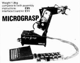
A real programmable robot for under £300! Micrograsp has an articulated arm jointed at shoulder, elbow and wrist positions. The entire arm rotates about its base and there is a motor driver gripper. All five axes are motor driven and four of these are serve controlled giving positive positioning. The robot can be controlled by any microcomputer with an expansion bus – the Sinclair ZX81 being particularly suitable.
