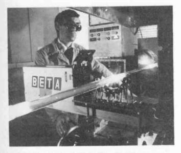
By passing the chemical ingredients through a vacuum in the hollow centre of a super-heated tube of coarse glass, thin layers of the purest optical fibre glass are gradually built up
