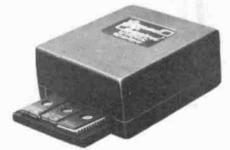
measures  $90mm \times 80mm \times 40mm$ . A fibre optic indicator is used to show that the unit is in operation. EPROMs are simply loaded onto the conductive foam supplied and inserted into the unit. The 'Uvipac' costs £21.45 as a standard unit or £24.95 with a built-in (15 min) timer. From Ground Control, Alfreda Avenue, Hullbridge, Essex SS5 6LT (0702 230324).
