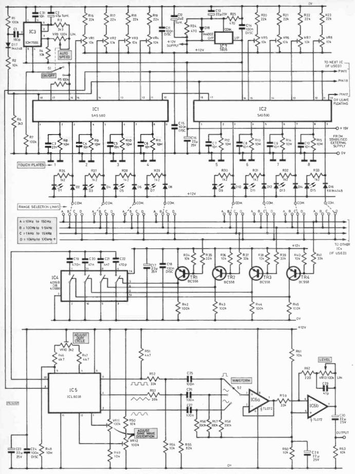
Fig. 3. Circuit diagram of the Spot Frequency Oscillator
