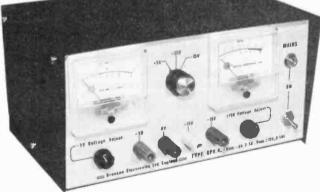
**Grenson BPU-4** bench power supply has three variable outputs: +3 to +8V (@ 2.5A +8 to +16V (@ 500mA and -8 to -16V (@ 500mA. Outputs are highly stabilised and fully protected against long term overload, short circuits and the injection of an external voltage. Voltage and current are independently monitored. Price £59 kit (£98 assembled). Available from **Grenson Electronics Ltd.**, High March, Daventry, Northants N11 4HQ. (0327 705521)
