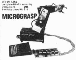
A real programmable robot for under £300! Micrograsp has an articulated arm jointed at shoulder, elbow and wrist positions. The entire arm rotates about its base and there is a motor driven gripper. All five axes are motor driven and four of these are servo controlled giving positive positioning. The robot can be controlled by any microcomputer with an expansion bus -the Sinclair ZX81 being particularly suitable.
