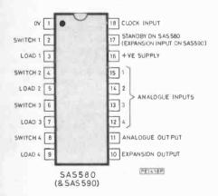
complex extra facilities are provided. Full interlocking is arranged such that only one input is switched to the output at any one time, except when two control inputs are deliberately turned on together as a momentary action. The control inputs themselves (switch 1, switch 2, switch 3, and switch 4) have been made touch sensitive, so that either nonmoving touch plates or conventional switches may be used as the switch input device.
