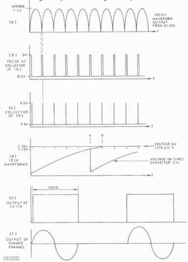
ply, in common with its three counterparts IC20-22, via TR1. TR1 is switched off by operation of the Strobe switch, thus disabling the output stage, and extinguishing all lights except the strobes. For an output from channel 1, both inputs of the NAND gate must be high. One input derives from the dimming circuitry and the other from the signal path.
