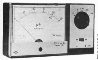
The **Chinaglia CP570** capacitance meter can accurately identify any capacitor within its range. An up to date meter suspension system is incorporated along with a shockproof ABS case. Both the test probes and the sockets in which they engage are designed to reduce contact resistance and wear. Five ranges can be set from 0 to  $0.5\mu$ F, accuracy is within 3% of reading. The CP570 is priced at £51 and is available from **Alcon Instruments Ltd.**, 19 Mulberry Walk, London SW3 6DZ (01-352 1897).
