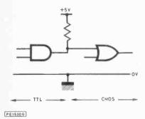
Fig. 9. Driving CMOS from TTL
