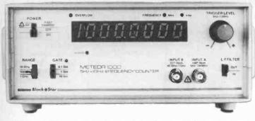
**Meteor 1000X** 5Hz to 1GHz precision frequency counter has temperature compensated crystal. Sensitivity is <50mV at 1GHz. Stability is  $\pm 0.5$  p.p.m. at  $-10^{\circ}$ C to  $40^{\circ}$ C with aging at  $\pm 1$  p.p.m. per year, and stability of  $\pm 0.2$  p.p.m. Battery or mains powered. Trigger level control. Three gate times: 0.1 sec, 1 sec and 10 sec. Price £258.75. Available from **Black Star Ltd.**, 9A Crown St., St. Ives, Huntingdon, Cambs PE17 4EB. (0480 62440)
