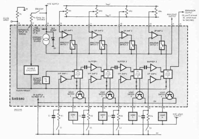
Fig. 2. Block diagram of the SAS 580 and 590
