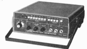
**Levell TG302** function generator can generate triangle, square, sine, pulse and ramp waveforms from 0.02Hz to 2MHz in 7 ranges. It provides 20V p.p. from a 50 $\Omega$  source with variable offset. TTL output. External sweep over three decades. Built-in frequency counter to 10MHz. Price £155.25, Available from **Levell Electronics Ltd.**, Moxon St., Barnet, Herts EN5 5SD. (01-440 8686)
