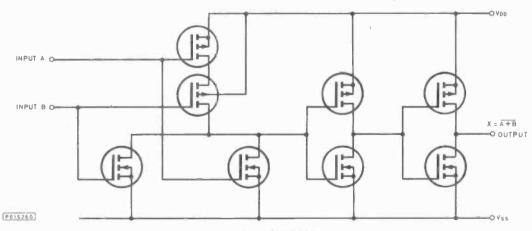
Fig. 5. B-series CMOS NOR gate
