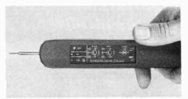
The **4500** transistor tester simplifies and speeds up the task of checking the p.n. junctions of discrete semiconductors, in or out of circuit. This lightweight hand held device features a series of l.e.d.s, which indicate the junction status. PNP or NPN transistors, diodes and open or short circuit junctions can be identified with parallel circuit values as high as 270 ohms or 33 microfarads. Price £18.40 from **Osborne Electronics**, Binstead Road, Ryde, Isle of Wight (0983 63622).
