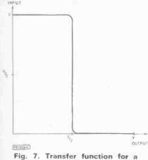
Fig. 7. Transfer function for a CMOS inverter
