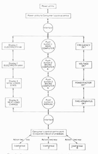
Fig. 3. Basic elements of an industrial consumer's interactive load control unit
