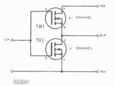
Fig. 1. Internal circuit of a CMOS inverter
