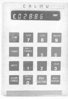
Credit and Load Management Unit (CALMU). This microprocessor controlled consumer unit will interact with the electricity board, optimising tariff rates and replacing the old meter system
