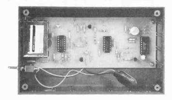
to the interlacing this gives two scans per horizontal line. The values in the pulse shaper have been chosen to give vertical lines of approximately the same width. If desired broader lines can be obtained by raising the values of R15 and R19.
