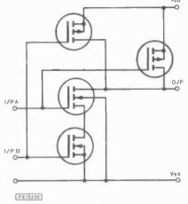
Fig. 2. CMOS NAND gate circuit
