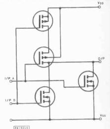
Fig. 3. CMOS NOR gate circuit
