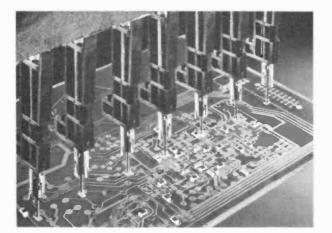
The unique pipettes of the Philips MCM range of automatic SMD placement machines
