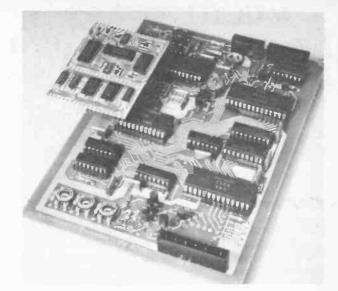
These boards fulfil identical functions. Generally, SMDs require only a third of the board space needed by conventional components. Photograph courtesy of Mullard Ltd. P.c.b. drilling is entirely eliminated
