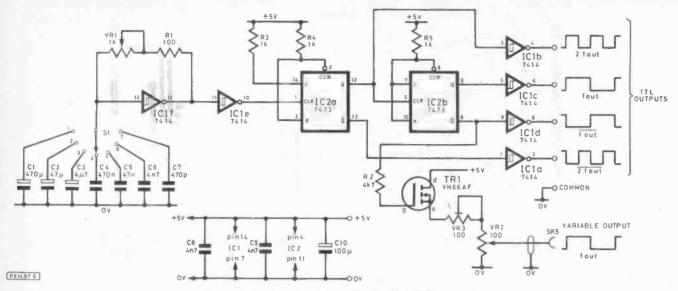
Fig. 1. Circuit diagram of the Logic Signal Generator
