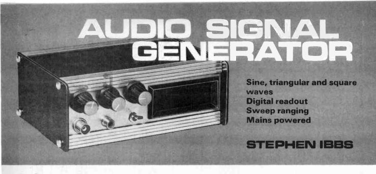
THIS design provides gain control of sine, triangle and square waves via an op-amp buffer. It has a TTL output for logic applications, and gives digital readout accurate to  $\pm 1$ Hz. No switched ranges are used, the potentiometer giving a 1000:1 sweep range, and for this reason a multiturn pot is specified to enable accurate settings to be made easily. The unit is mains-powered, giving  $\pm 12$ V and  $\pm 5$ V.
