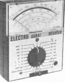
Model: Miselco Electro Super. Ranges: Voltage a.c./d.c. 100mV-1000V (9 ranges). Current a.c./d.c. 100µA-6A (8 ranges). Resistance 0-1MΩ (3 ranges). Special Features: dB scale. Price: £56-00. Supplier: Alcon Instruments Ltd., 19 Mulberry Walk, London SW3 6DZ. (01-352 1897).
