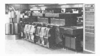
MCM III is a hardware-automatic placement machine accommodating up to 12 placement heads. A typical handling capacity is 200,000 component placements per hour. Photograph courtesy of Mullard Ltd.
