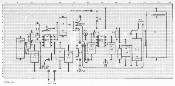
Fig. 5. Veroboard layout for the Baby Alarm
