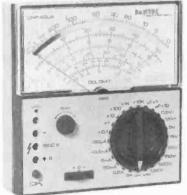
Model: Pantec Dolomiti. Ranges: Voltage d.c. 150mV-1.5kV (9 ranges). Voltage a.c. 5V-1.5V (6 ranges). Current d.c.  $50\mu$ A-5A (6 ranges). Current a.c. 5mA-5A (4 ranges). Resistance  $500\Omega$ - $50M\Omega$  (6 ranges). Decibels (6 ranges). Special Features: Universal signal injector. Price: £57.61. Supplier: Alcon Instruments Ltd., 19 Mulberry Walk, London SW3 6DZ (01-352 1897).
