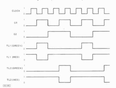
Fig. 8.4. Timing diagram for the traffic light simulator
