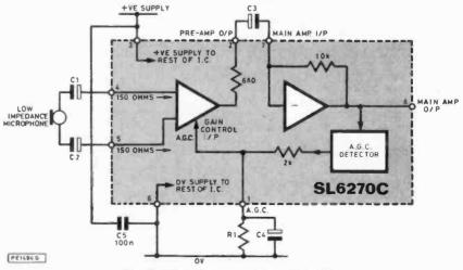
Fig. 2. Block diagram of the SL6270C
