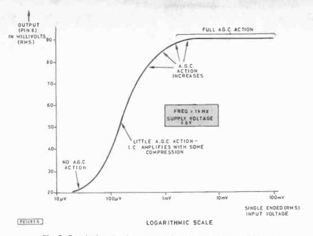
Fig. 3. Graph showing input against output (unbalanced input)
