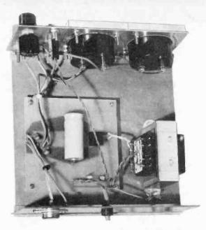
Fig. 4 and use thicker than normal wire for the output connections to avoid unnecessary voltage drops caused by lead resistance. Take care with the mains connections, particularly those to the neon as these can be easily touched inadvertently. After a final check the case can be bolted together and a useful piece of equipment added to the workbench.
