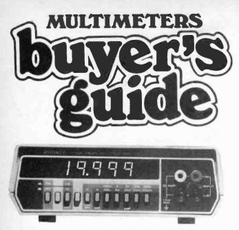
Model: Keithley 179A. Ranges: Voltage d.c. 200mV-1200V (5 ranges). Voltage a.c. 200mV-1000V (5 ranges). Current a.c./d.c. 200µA-20A (6 ranges). Resistance 0-20MΩ (5 ranges). Special Features: Hi-lo range option, over-range indication. Price: £385. Supplier: Keithley Instruments Ltd, 1 Boulton Road, Reading, Berks RG2 ONL. (0734 861287).
