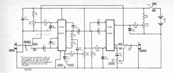
"fuzz" effect. The attack and decay times of the circuit need to be short, due to the rapid changes in the dynamic level of the input signal, but smoothing capacitors C6 and C11 must not be made too small or distortion performance suffers. It is, therefore, a matter of choosing values which give a good compromise between response time and distortion levels.
