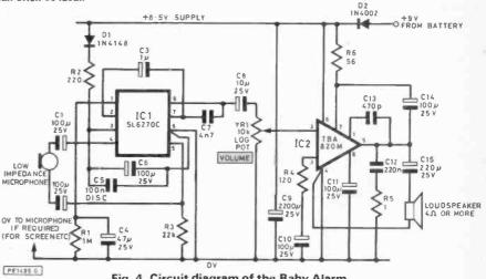
Fig. 4. Circuit diagram of the Baby Alarm
