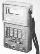
Model: ALT/AI KD305. Ranges: Voltage d.c. 0-1000V (4 ranges). Voltage a.c. 0-750V (2 ranges). Current d.c. 0-10A (4 ranges). Resistance 0-2MΩ (4 ranges). Price: £32.20. Supplier: Semiconductor Supplies International Ltd., Dawson House, 128/130 Carshalton Road, Sutton, Surrey SM1 4RS. (01-643 1126).
