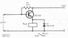
whereupon conduction will cease. Nothing more is therefore required to produce a comprehensive and reliable system than this elementary circuit, together with a continuous loop shorting the base to ground, which would cause the unit to operate if it is broken at any point.
