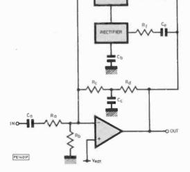
Fig. 1a. The normal NE571 compressor configuration
