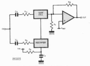
Fig. 1c. The NE571 as an expander
