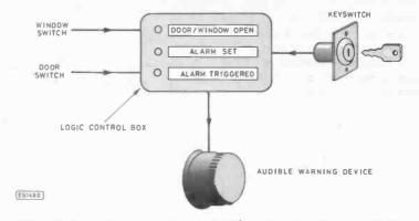
Fig. 8.6. Essential components of the intruder alarm for the electronic shop
