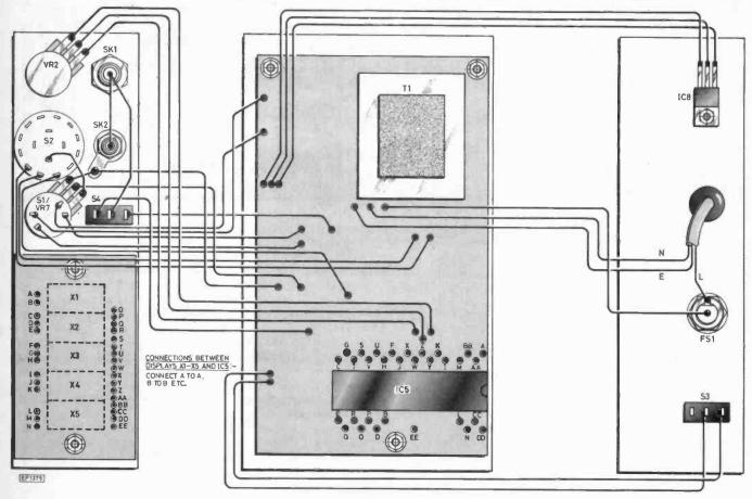
Fig. 5. Interwiring details of generator
