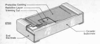
Structure of a SMD, laser trimmed resistor
