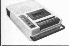
'cue and review' mode is incorporated: This allows fast-forward or rewind to be done with the 'play' button depressed so that playback begins immediately the wanted section of the tape has been found.
