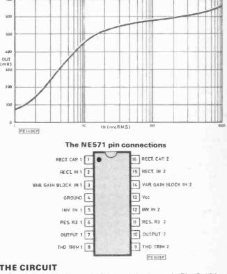
Fig. 2. Typical input/output characteristic of the sustain unit
