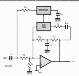
Fig. 1b. The compressor arrangement used in this design
