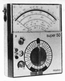
Model: Miselco 'Super' 50. Ranges: Voltage d.c. 150mV-1000V (8 ranges). Voltage a.c. 0-1000V (5 ranges). Current d.c. 20µA-3A (10 ranges). Current a.c. 3mA-3A (6 ranges). Resistance 0-50MQ (5 ranges). Decibels -10 to +61 (5 ranges). Special Features: Diode test facility. Price: £50. Supplier: Alcon Instruments Ltd., 19 Mulberry Walk, London SW3 6DZ. (01-352 1897).
