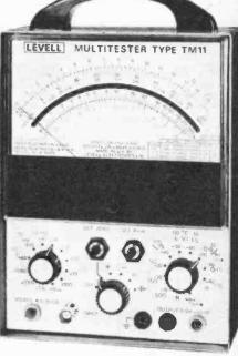
Model: Levell TM11. Ranges: Voltage d.c. 150µV-50kV (18 ranges). Voltage a.c. 50µV-50kV (19 ranges). Current d.c. 150pA-50A (24 ranges). Current a.c. 50pA-50A (25 ranges). Resistance 0-10GQ (7 ranges). Decibels -90 to +50 (15 ranges). Special Features: Diode test, temp. sensor (7 ranges), amp output. Price: £189-75. Supplier: Levell Electronics Ltd., Moxon St., Barnet, Herts. EN5 5SD (01-440 8686).
