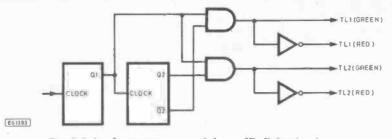
Fig. 8.2. Logic arrangement of the traffic light simulator
