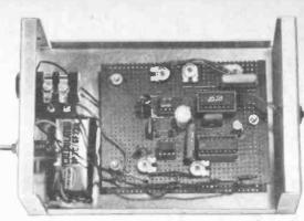
The separate tone generator with phototransistor on right panel
