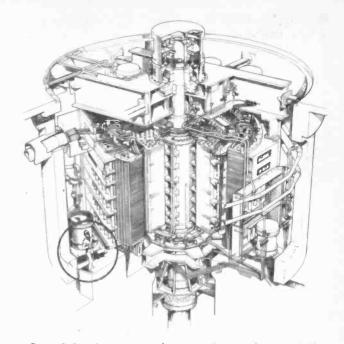
One of the six generator/motors, the rotating parts of which weigh 484 tonnes
