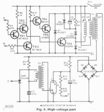
low. This pulse briefly turns on TR9, firing CSR1 and hence the tube. The recharge cycle begins, with IC1 output going high, and when C6 is fully charged, going low again. TR7 collector goes from low to high, and if S3 wiper is still connected, this transition initiates the triggering, and so the cycle repeats until S3 is opened.
