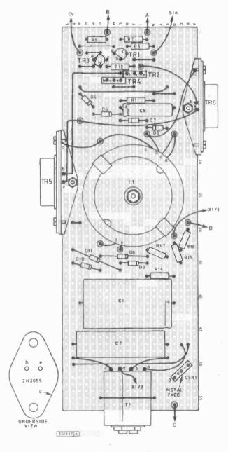
Fig, 5. High voltage gun board
