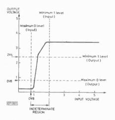
Fig. 3.18. TTL buffer transfer characteristics
