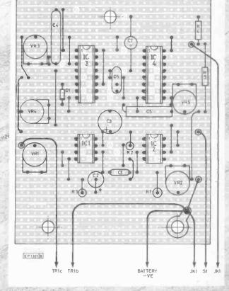
Fig. 2. Veroboard assembly of tone generator
