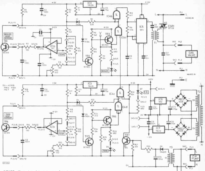
BC109, silicon transistors are used as temperature sensors. Although each circuit could have monitored the voltage generated across a silicon junction diode, transistors were chosen because in a three-terminal mode they offer gain at the sensors themselves.
