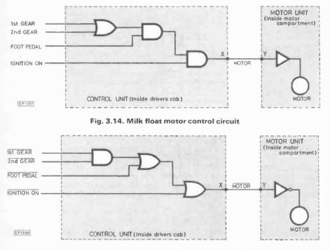
Fig. 3.15. Motor control circuit using negative logic
