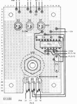
Fig. 9. Potentiometer board layout
