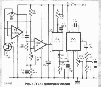
to minimum and VR3 and VR5 to mid position. A jack plug should be connected to a suitable power amplifier and loudspeaker and inserted at JK1.
