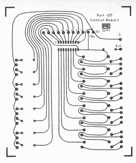
Fig. 3.4. Low voltage output control board printed circuit layout (actual size)
