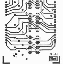
Fig. 5.3. Track side p.c.b. layout of CMOS input option board (actual size)
