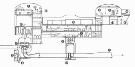
Section through station. Electricity generated in the machine hall at 18kV is conducted via aluminium bus-bars to the transformer hall, then at 400kV to the national grid system through a 6 mile underground tunnel
