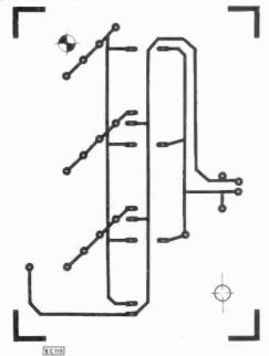
Fig. 5.4. Component-side p.c.b. layout of CMOS input option board (actual size)
