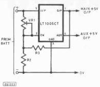
Fig. 3. 'Battery saver' circuit
