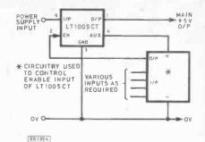
Fig. 4. Using both the 'Enable' and 'Aux' facilities
