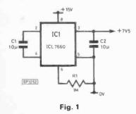
converter in a similar manner. The circuit configuration is shown in Fig. 1:
