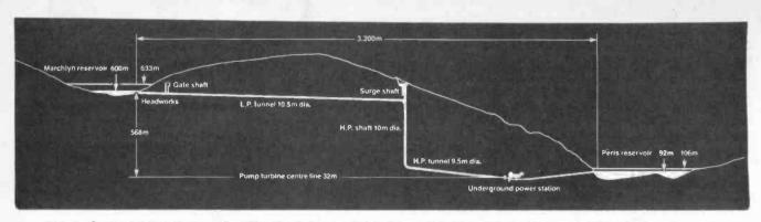
Fig. 1. Cross-sectional view showing the basic layout at Dinorwig. The overall distance between the upper and lower reservoirs is around 3.2 kilometres. The high-pressure and surge shafts together form a vertical shaft 1 kilometre deep-nine times the height of Nelson's Column
