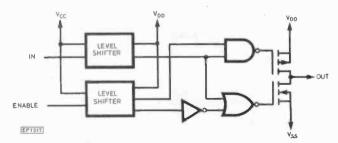
Fig. 5.1. Logic diagram of a single translator in the CD40109B
