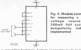
Fig. 4. Module connections for measuring a floating source with 200mV full scale and indication
