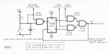
Fig. 1. 1MHz to 2MHz dynamic changeover for UK101
