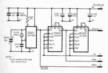
Fig. 4.6. Internal Clock option circuit diagram
