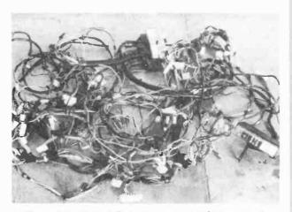
Wire, wires, wires! Enough to stretch  $\frac{1}{2}$ km were ripped out of the conventional Delta to be replaced with 75 metres of wire and fibre-optic cable
