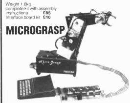
A real, programmable robot for under £200! Micrograsp has an articulated arm jointed at shoulder, elbow and wrist positions. The entire arm rotates about its base and there is a motor driven gripper. All five axes are motor driven and servo controlled, giving positive positioning. The robot can be controlled by any microcomputer with an expansion bus – the Sinclair ZX81 being particularly suitable.
