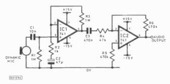
Fig 1.1. Preamplifier circuit
