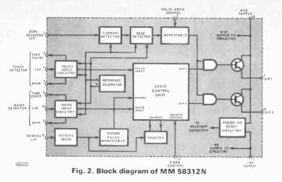
the 'two minute' timer facility is to be used. (Because this delay period is frequency dependent, it will be only 103 seconds if 60Hz mains is used). The timer is enabled by connecting pin 11 to the positive supply while using output 2 (pin 13) of the i.c. to trigger the triac, and is disabled by connecting pin 11 to the negative supply, and using output 1 (pin 1) of the i.c. to trigger the triac.
