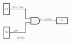
Fig. 2.7. The shop light control circuit
