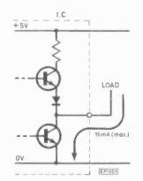
Fig. 2.14a. Current flow in the logic 0 state
