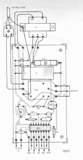
suitably accurate thirty second switch-on time. When used to provide longer switch-on times the error is multiplied by the division ratio used in the counter circuit, and slight readjustment of VR1 may be needed when the unit is programmed for normal use if a high degree of accuracy is required.
