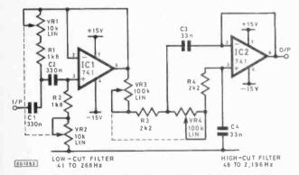
Fig. 1.3. Audio amplifier incorporating bass and treble controls
