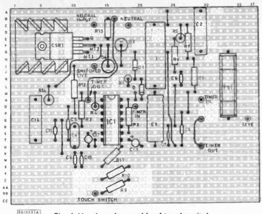
Fig. 4. Veroboard assembly of touch switch
