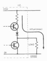
Fig. 2.14b. Current flow in the logic 1 state
