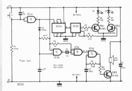
THIS circuit allows each player a maximum of ten seconds to make his move and push the switch or the buzzer will sound and he will have lost the game. The l.e.d.'s indicate which player has lost when the buzzer sounds.
