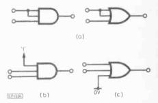
Fig. 2.16 a, b and c. Dealing with unused gate inputs
