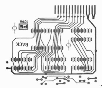
Fig. 4.3 (above). Z-Mod option p.c.b. layout (track-side) Fig. 4.4 (above right). Z-Mod option p.c.b. layout (componentside)
