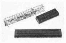
The bargraphs have a wide viewing angle of  $\pm 30^{\circ}$  with very low cross-talk between segments. The units are designed generally for solid state indication in all forms of linear analogue display. One major application area is in VU meters used in Hi-Fi equipment, and one type (D634P) has been constructed with 7 green and 3 red segments specifically for this purpose. Further information from Brian Penks, AEG-Telefunken (0753 872101).
