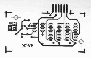
Fig. 4.7. Clock option p.c.b. layout (track-side)
