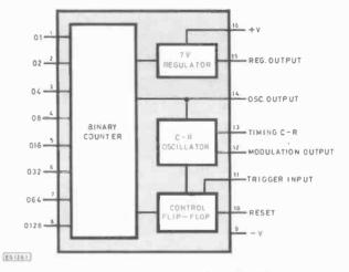
Fig. 1. Block diagram of the UA2240
