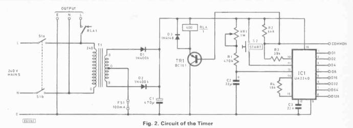
duration of each oscillator cycle is a convenient 1CR, and the timing resistor should be between 1k and 10M. The timing
