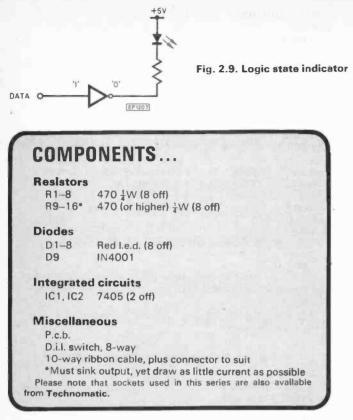
The simple, low cost board (approx. £5 on a completely d.i.y. basis) described here allows the computer to simulate being used to turn on and off devices such as small motors or model railway circuits and signals and the functioning of safety devices such as 'limit' switches to prevent over-running.
