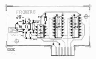
Fig. 4.9. Clock option component layout (actual size)
