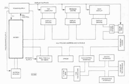
Fig. 1. Block diagram of the Driver Information System. The trip computer and message centre each uses a twenty character alpha-numeric display. All displays are vacuum fluorescent, which will remain the preferred technology until l.c.d.s are developed further
