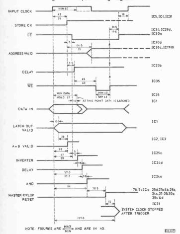
Fig. 1.1. Analyser timing diagram
