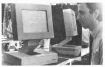
As a VDU, the display may be driven entirely digitally, each pixel being addressable on a row-and-column basis. Pulse durations determine illumination levels, thereby allowing a full greyscale. But there is nothing grey about the future of this development, which is quite capable of invading the television market in due course.
