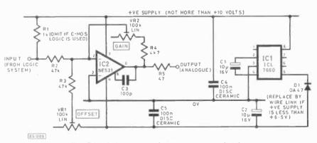
Fig. 8 Logic level to analogue converter circuit
