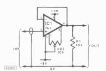
OR measuring voltages in circuits where currents are very small and resistances large, an ordinary multimeter is unsuitable because it draws an appreciable current from the circuit and therefore gives erroneous readings. It may also upset the operation of the circuit. This very simple impedance converter makes it possible to get true readings with even the most ordinary meter.
