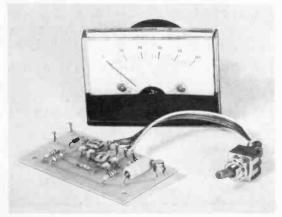
and with the unit adjusted in this way a low reading on the meter will indicate that watering is needed. Always make sure that the probes are pushed right down into the soil and are making good contact with it.
