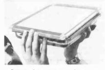
Because plasma acts as an electron source, as opposed to the hot cathode in a conventional c.r.t., this display requires a mere 4kVfor its acceleration electrode (c.r.t. requires 20kV), and so it produces virtually no X-rays. This is a nice feature since the display will first begin to appear in VDU applications; and
