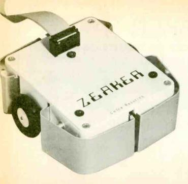
ZEAKER is a small, low cost computer controlled robot vehicle designed to have all the normal functions of a "turtle" i.e. steering, lights, pen, horn and bump sensors but it is also capable of being expanded using photosensors for eyes to seek out or avoid light or to follow white lines etc; with a complex sound generator for special noises à la R2D2, and with computer speech.
