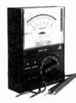
18 ranges, 3'' meter, DC Volts: 0-1000, AC Volts: 0-1000. Current: 0-50  $\mu$ A, 0-250mA, DC. Resistance: Rx1, Rx10, Rx1000 (24 ohms, centre scale). dB: -20 to +62 in four ranges. Accuracy: ± 3 DC, ± 4 AC.
