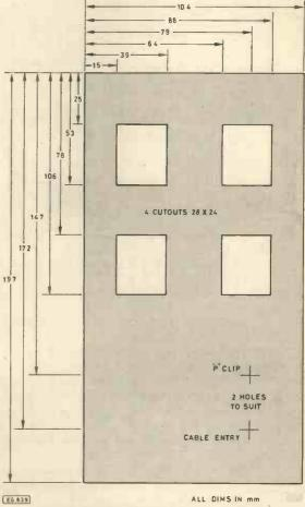
Fig. 10. Cutting details for the rear panel
