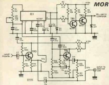
THE accompanying design has been used by the writer to detect the morse code tones found on the amateur bands. It takes its input from the audio output socket of a communications receiver or other radio, at line level, i.e. about 200mV peak to peak. It produces a single bit TTL compatible output, which can be fed directly into a computer port.
