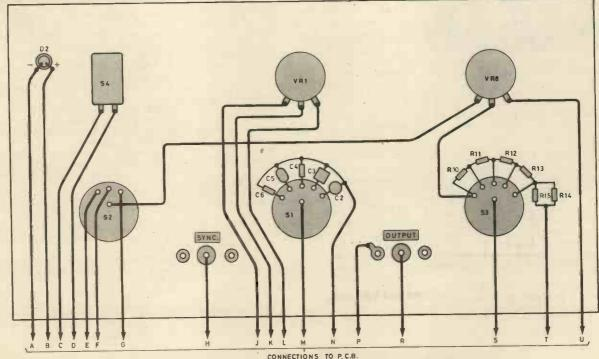
EGBIB Practical Electronics May 1982 Fig. 6. Control panel assembly showing leads connecting to Fig. 4
