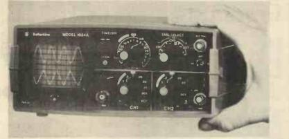
The new Ballantine 1024A mini oscilloscope, available from PPM Limited, has been designed to suit the needs of the field engineer, and light weight and small size have been achieved without reduction in instrument performance. The 1024A's specification is equal to laboratory bench scopes two or three times larger and heavier; it is shock and weather proof and will operate in harsh environments. The 1024A weighs 2.1 kilos and measures 87mm × 203mm × 220mm.
