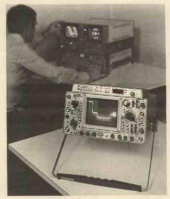
Tektronix 468 digital storage oscilloscope
