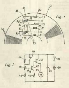
enables it to change running speed automatically and continuously as it tracks in across the disc and so keep the playing speed constant at around  $33\frac{1}{3}$ rpm. This modification is described in US patent 4 232 202.
