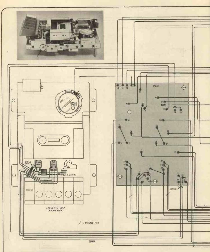
Fig. 3. Wiring diagram for the Quasar. Note the arrowed screw in the photograph should be shorter than the other bracket screws
