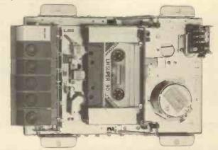
Photograph showing the top of the cassette mechanism. After the cassette mechanism has been mounted into the case and screwed into position the Perspex cover should be glued onto the two aluminium brackets mounted either side of the cassette compartment. Finally the offcut from the fascia panel legend should be trimmed and glued onto the cover.
