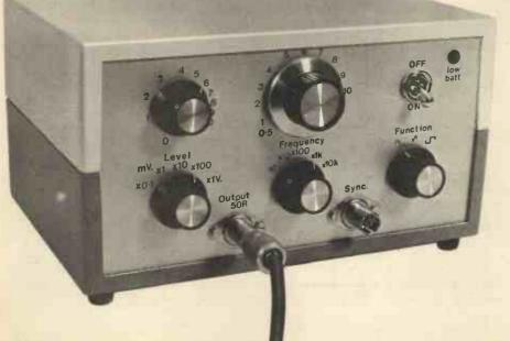
Provides sine, square and triangular output waveforms
