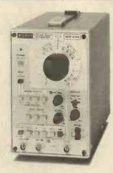
Up to five frequency decades can be covered in a single sweep with automatic sweep times being internally selected from 0.1 to 100 seconds both continuous and single to match the application. The single sweep mode can also be controlled manually from the front panel or sweep speeds determined by external signals. Automatic sweep speed compensating has been provided to maintain a constant sweep time period for any arbitrarily set width.
