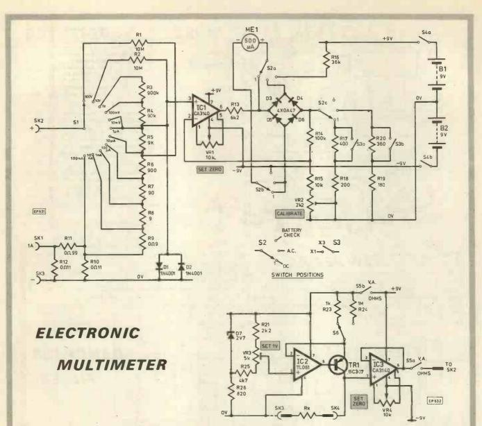
THIS multimeter design has an input impedance of  $1M\Omega/V$  or  $333k\Omega/V$ depending on whether one is reading in decade multiples of 1 or  $3V/mV/A/mA/\muA$ . The f.s.d. ranges are 10mV to 300V,  $1\muA$  to 3A a.c. or d.c. Protection is by D1, 2 and by R13.
