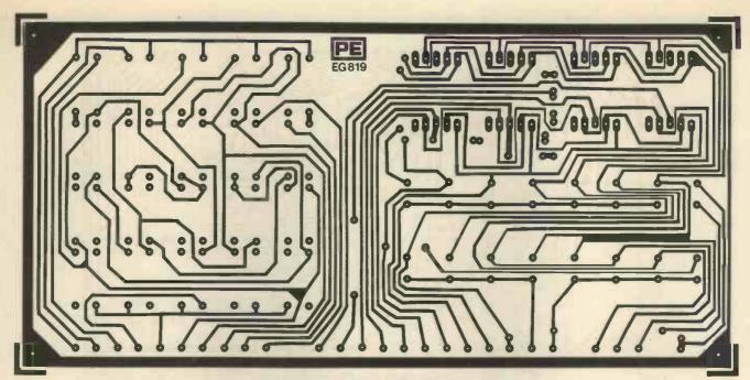
Fig. 3. P.c.b. design for the display keyboard
