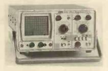
The 3131 features 5mV/div sensitivity with full X-Y operation plus the extra feature of algebraic addition and subtraction. The timebase is fully constructed from 200ns to 0.2s/div with a versatile trigger circuit which operates to at least 35MHz and includes TV Field and line frequency modes.
