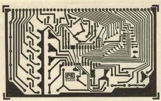
Fig. 5. P.c.b. design for the logic driver board
