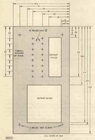
Fig. 9. Cutting details for the front panel
