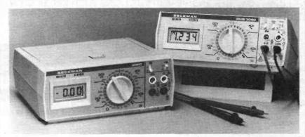
Following the success of their hand-held digital multimeter family, Beckman have introduced two portable bench-top models. The instruments require no external power supply and will operate continuously for 12,000 hours from standard alkaline batteries.
