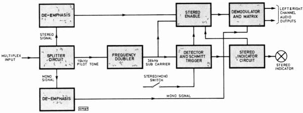
Fig. 2. Block diagram of the LP1401 stereo decoder
