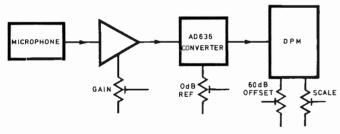
Fig. 2. Block diagram.
