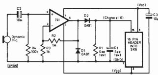
Fig. 7.10. Audio Detection using the A/D converter
