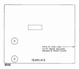
Fig. 6. Template for front panel drillings
