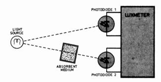
Fig. 9. Making absorbence measurement
