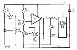
Fig. 7.8. Temperature Sensor with voltage amplifier
