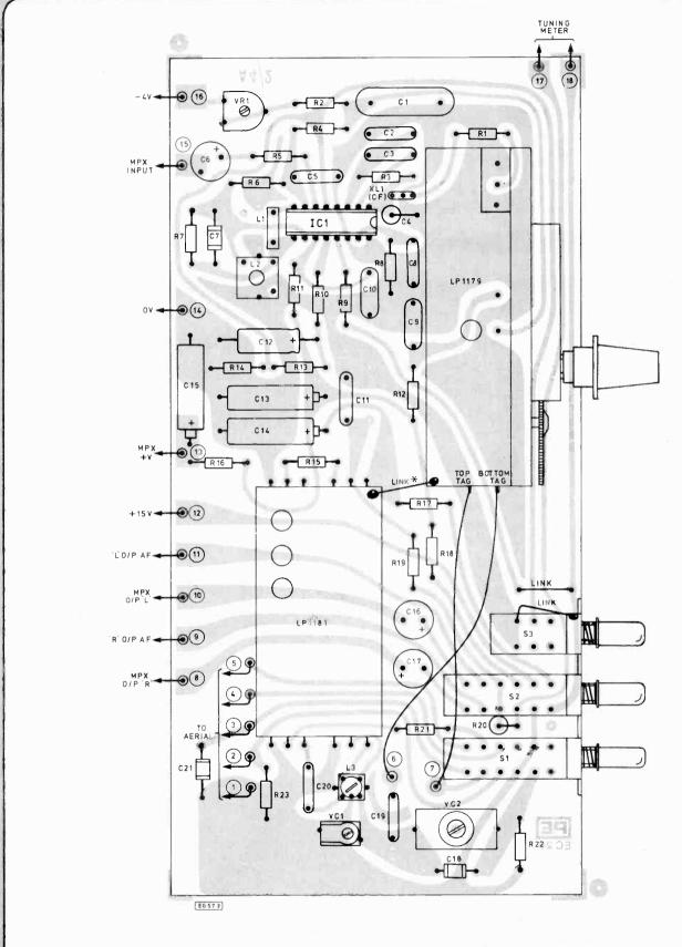
Fig. 5. Component layout for the main board. \*Note this link is soldered to the case of each module
