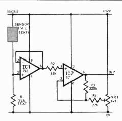
The circuit shown is a linear reading pressure sensor. The voltage at the output of the potential divider formed by the sensor and R1 (which rises with increased pressure) is buffered by IC1 and fed to the amplification stage IC2—the resulting out-
