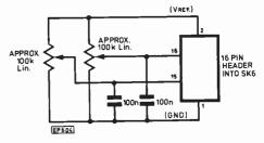
Fig. 7.5. Connection of 2 axis joystick to A/D converter
