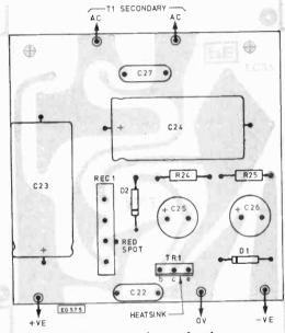
Fig. 9. Component layout for the p.s.u.
