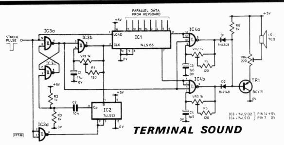
NTENDED as an addition to microprocessor or VDU keyboards, this produces a different pattern of high and low tones for each key on the keyboard. Although it is not necessary to learn these different patterns, after some use the tone generator becomes a real aid to accurate typing.
