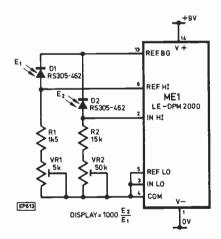
Fig. 7. Ratiometric method of measurement
