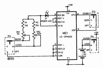
Fig. 3. Circuit of Lightmeter
