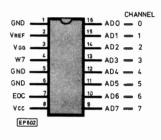
quad latch IC7. This is enabled by line W7 from the Decoding Module. The 8 channels are selected by POKEing the channel number (0-7) to address 61319. Thus the command POKE 61319, 6 will connect channel 6 (at pin 10 of SK6) to the input of the converter.
