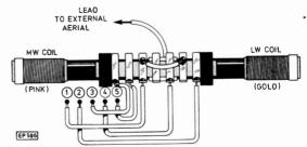
Fig. 7. Wiring details for the aerial assembly
