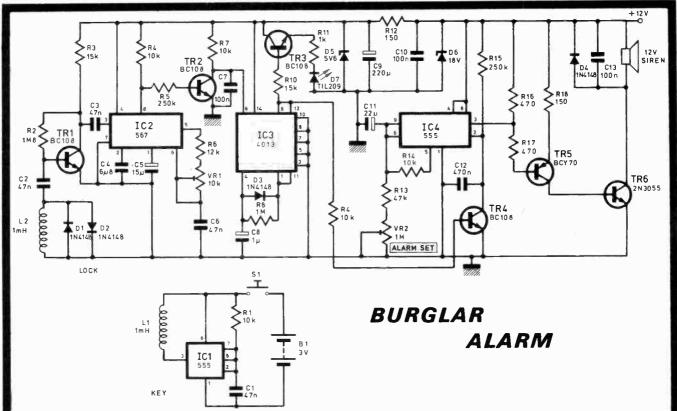
THIS consists of an astable multivibrator used as a key, and a lock circuit. This operates at a frequency of 3.2kHz and uses a 1mH choke as the load which acts as a primary of a transformer, when brought into close proximity to the lock.
