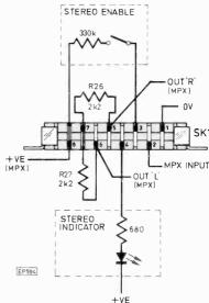
Fig. 10. Connection diagram for SK1
