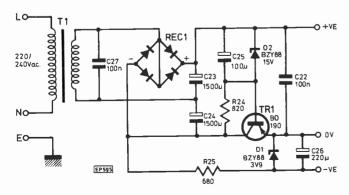
Fig. 3. Circuit diagram of the power supply unit
