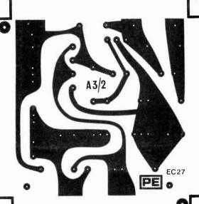
Fig. 8. P.c.b. design for the p.s.u.
