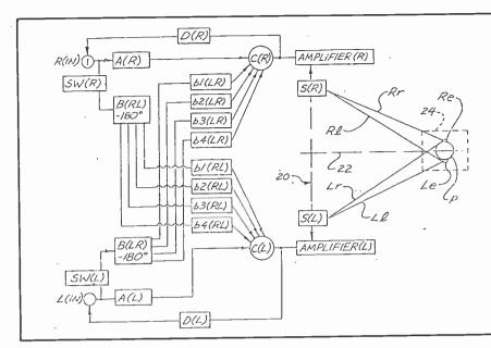
loudspeakers in the following manner. The listener's left ear first hears a sound direct from speaker LS along path Le. At the slightly later time when the listener's right ear would hear the same sound from loudspeaker LS along slightly longer path Lr, it also receives the delayed replica of that signal in anti-phase from speaker RS. There is thus cancellation at the right ear so the left ear hears only the left speaker.
