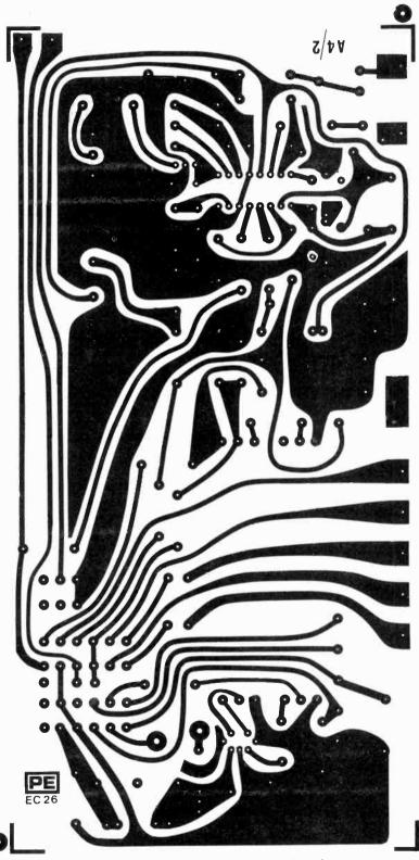
Fig. 4. P.c.b. design for the main board
