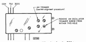
Fig. 6. AM oscillator modification for the FM tuner
