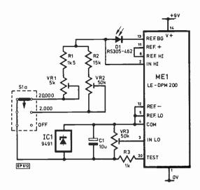
Fig. 6. Method of incorporating offset adjustment
