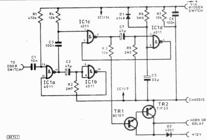
alarm will sound for about 2 minutes and you'll have about 20 seconds to turn the unit off after entering the car. These times can be changed by altering the RC-networks. If the diode D2 is connected
