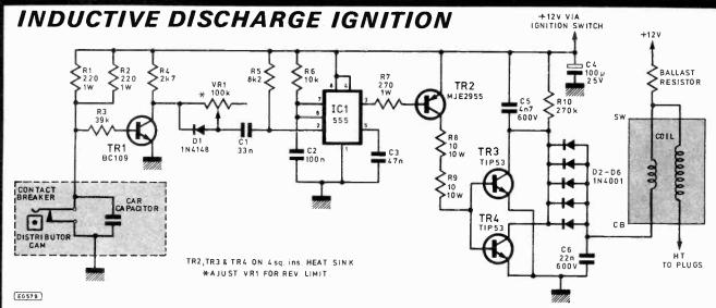
WITHOUT going into the controversy about the advantages of capacitor or inductive discharge ignition versus normal ignition, a circuit for inductive discharge ignition is presented here. It is a points assisted unit in which the coil load of 3.5 amps is removed to a switching transistor. Other features in the circuit are: rev limit, points bounce control, long dwell time, lower RFI than a CDI system.
