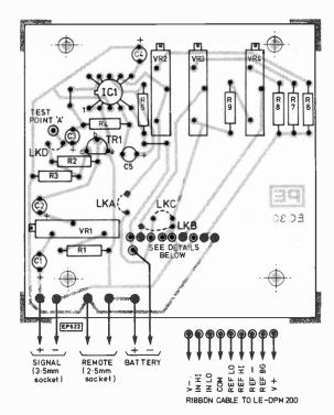
against another calibrated meter, VR1 should be adjusted to provide the correct reading for the particular microphone used.
