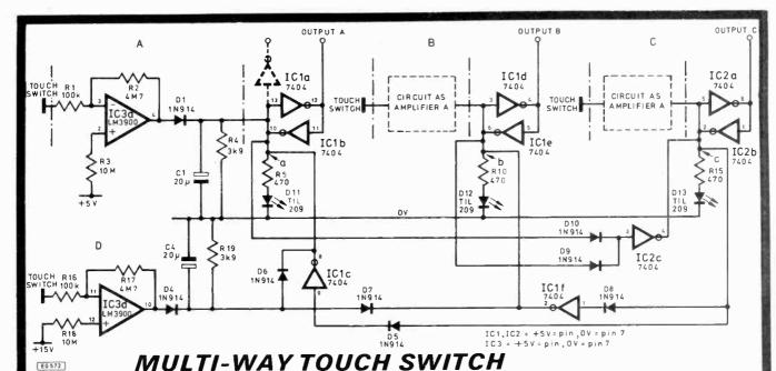
THIS circuit has been developed to eliminate the possibility of activating the wrong combination of switches. Switch C can never be switched 'on' when either switches A or B or both are 'on'. Circuit D enables switches A and B to be switched 'on' simultaneously.
