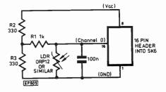
Fig. 7.6. Connection of light sensor to A/D converter
