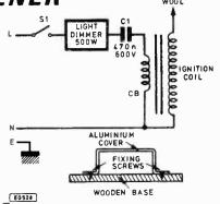
The capacitor in our circuit passes this rapid switching charge through to the ignition coil at 100 times per second for 50Hz mains, rather like the contact breaker on the car opening 100 times per second, while at the same time isolating the mains from being directly connected to the ignition coil. Therefore 100 high voltage pulses are produced per second, the amplitude of which are controlled by the dimmer setting.
