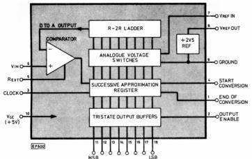
Fig. 7.1. ZN427 Block Diagram
