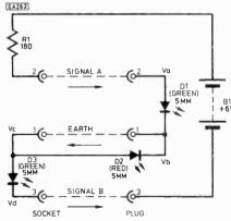
LEDS SHOULD BE OF THE SAME TYPE AND MANUFACTURE
