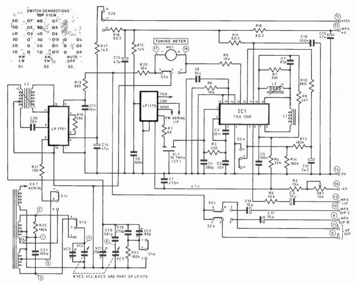
Fig. 1. Main circuit diagram of the PE Quasar
