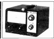
AG203 Low Distortion Oscillator — 10Hz to 1MHz in 5 ranges < 0.1% distortion — very flat O/P to 7V r.m.s. sinewave from 600 ohms, squarewave 10V pp — Ext. Sync. — > 60dB's of variable output attenuation
