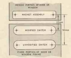
Fig. 2.8. Switch mounting details
