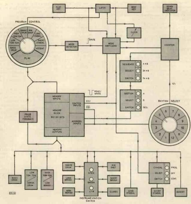
Fig. 2. Schematic of Master Rhythm
