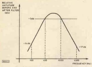
Fig. 2.3. Bandpass filter characteristics
