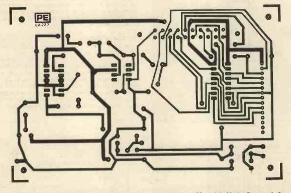
Fig. 2.6. P.c.b. design and component layout for the interface board (Copyright Modus Systems Ltd)
