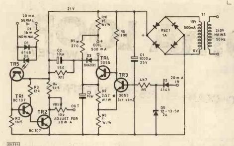
Fig. 1. Circuit diagram of opto-coupled 20mA loop. When in optoisolated mode, the OUT from VR1 is connected to IN at D2 (as on p.c.b.) The input at D2 can be used as a non-isolated RS232 input
