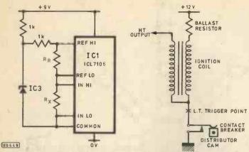
Fig. 2. Ratiometric resistance Fig. 4. Ignition system triggering measurement
