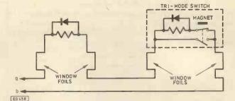
Fig. 2.10. Tamper-proof system for window foils.
