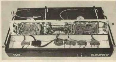
turntables, gooseneck arms and other exposed metalwork via 16/0.2 wire to the chassis earth commoning point.
