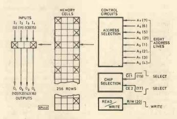
Fig. 1. Showing simplified operation of a 5101
