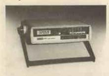
Thirty measuring ranges are provided covering the five basic functions of d.c. and a.c. voltage, d.c. and a.c. current, and resistance. In addition, diode test and frequency measurement functions are included. Frequency measurement is achieved via a crystal controlled timebase, and is particularly useful for monitoring oscillators or checking microprocessor clock frequencies, etc. Maximum reading is 3999-9kHz with overflow to 7MHz.
