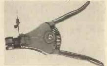
A single squeeze operation strips the insulation from single and stranded wires without damage. Its wide jaws permit fast and accurate stripping without any nicking or scraping of the wire and a gauge is supplied to ensure consistent lengths of stripping during fast production work. Five diameters of wire can be used on this tool, which has the following size cutter: 1.0, 1.6, 2.0, 2.6 and 3.2mm. Of an all metal construction, it is available ex stock priced £10.50.
