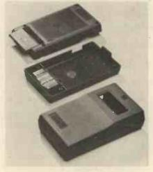
part body by the use of four self-tapping screws, whilst the bottom section will house a board of  $56 \times 105$  mm. The two sections snap together and are secured by four screws through the base. There is an integral battery compartment which will accept a **PP3** or a nickel cadmium stack of  $25 \times 45$  mm, it has a slide-off cover which allows easy access.
