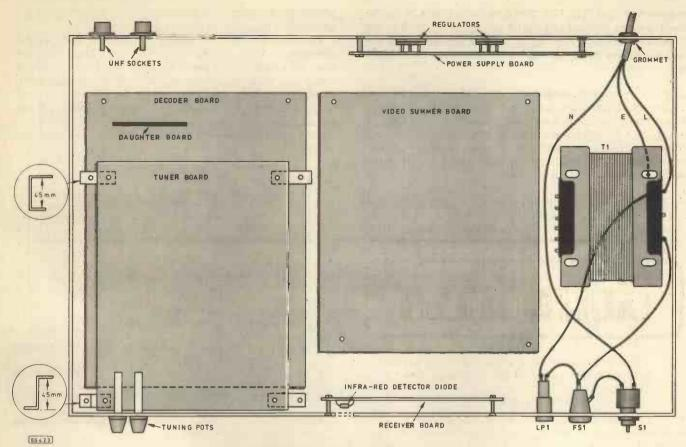
Fig. 4.2. Internal layout of the case
