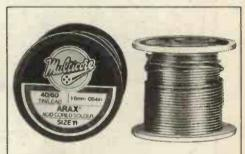
Metal Soldering. Arax Multicore 4-acid-core solder for metal fabrication (not aluminium) and repairs. 40/60 tin/lead 1.6mm dia. Size 11. £3.91 per reel.
