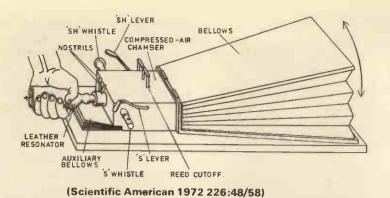
Fig. 1. Sir Charles Wheatstone's reconstruction of Van Kempelen's speaking machine. A bellows fed air into a reed which excited the hand controlled resonator. Four separate restricted passages were included for the consonants and nasals.
