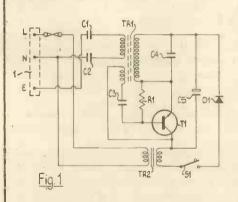
Figure 1 shows a sender or control unit which plugs into a mains socket Transistor T1, resistor R1, capacitors C3, C4 and transformer TR1 function as a feedback oscillator connected to the neutral and earth pins of a standard size mains plug 1. Capacitors C1, C2 block DC and the oscillator is powered by step down transformer TR2, rectifier diode D1 and smoothing capacitor C5. When control switch S1 is closed the plug impresses an oscillation on the house mains wiring.
