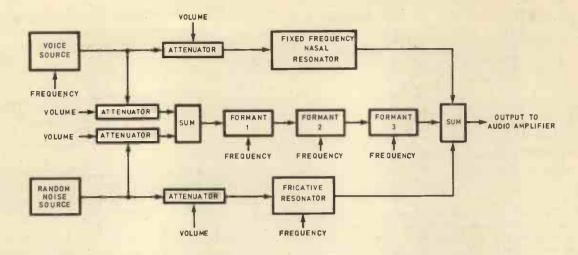
Fig. 4. This "classical" voice synthesis unit requires just nine parameters to specify a single sound (four "volumes" and five frequencies). The "frame" of nine parameters is updated (typically) fifty times a second during the production of a word.
