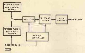
Fig. 5. The Texas Instruments Linear Predictive Coding System codes words into the coefficients of a ten-stage digital filter. A maximum of 2400 bits of data per second of speech are required to adjust the filter coefficients, type of excitation and pitch and frequency as a word is produced.
