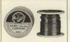
Aluminium Soldering. Alu-Sol Multicore 4-core solder for soldering most types of aluminium. No extra flux needed. 1.6mm dia. Size 4. £11.50 per reel.
