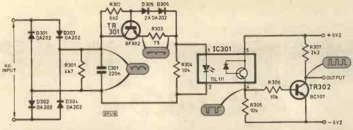
Fig. 2 Circuit diagram of new phase reference pulse generator
