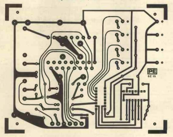
Fig. 4.4. Corrected p.c.b. design for the Tuner board
