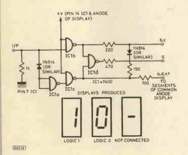
HIS circuit for yet another logic tester differs from others by instead of lighting one l.e.d. for logic 1 and another for logic 0, actually displaying a 1 or an 0 on a common anode seven-segment display:
