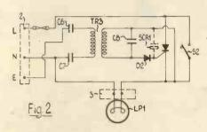
the live pin of mains output socket 3. The potentially confusing effect of spurious mains signals can be minimized by an extra capacitor downstream of diode D2 to slow down response of the thyristor to oscillation in the circuit TR3, C8.
