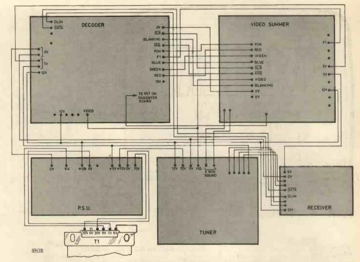
Fig. 4.1. Wiring diagram for the complete system. Note the annotation of plug PL3 on the decoder board was shown incorrectly in Fig. 2.4 (F1 was omitted)
