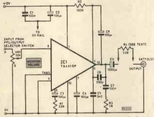
Fig. 11. Monitor Amplifier circuit with p.c.b. below and layout right
