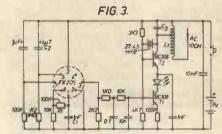
Coil L1 is a step up transformer which matches the low output impedance of T2 to the high impedance presented by the short aerial AE. The inventor advocates the use of this step up transformer to obtain correct electrical matching because in more conventional transmitters the output has a higher impedance than the aerial, whereas the reverse is the case in his arrangement. To keep dimensions of the transformer small, one transformer winding is made concentric to the other.
