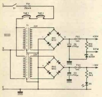
Fig. 7. Power supply circuit
