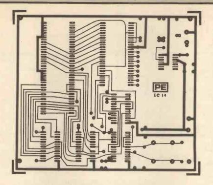
Fig. 6. Printed Circuit layout (actual size)
