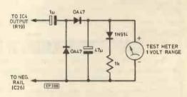
Fig. 10. Circuit for setting up search coils
