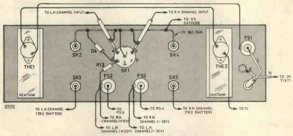
Fig. 12. Wiring diagram for the rear panel.
