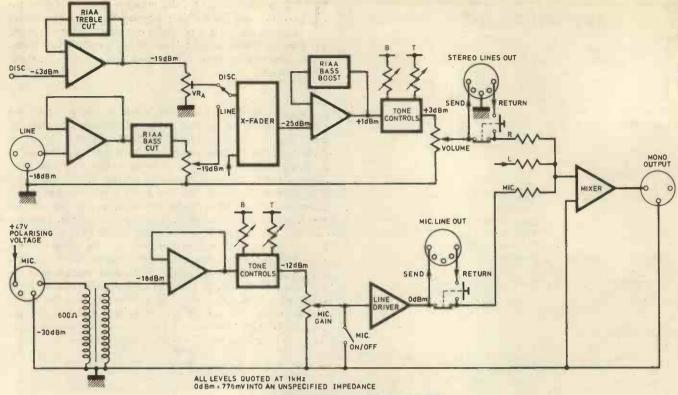
Fig. 1. Block diagram of main circuitry
