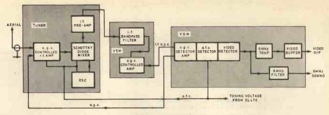
Fig. 2.1. Block diagram of the Tuner
