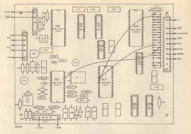
Fig. 2.6. Component layout of the Decoder Board. Note C32 is not used on the supplied board
