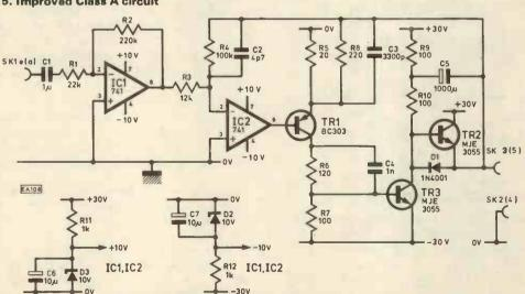
Fig. 8. Circuit diagram of one channel of the Class A emplfier. (Connections for R.H. channel shown in brackets.)
