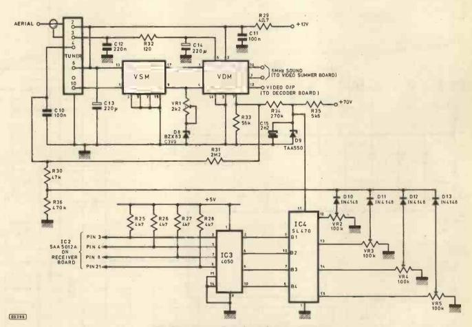
Fig. 2.2. Circuit diagram of the Tuner Circuit
