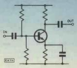
Fig. 1. Conventional R.C. coupled stage
