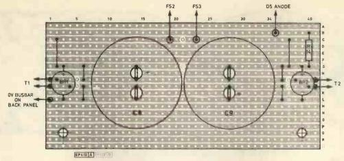
Fig. 11. Veroboard layout of the p.s u
