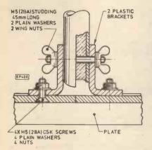
Fig. 6 (left). Search plate mounting assembly
