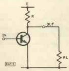
Fig. 2. Simple Class A circuit
