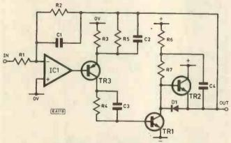
Fig. 5. Improved Class A circuit
