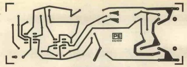
Fig. 8. P.c.b. design for one channel of the amplifier.
