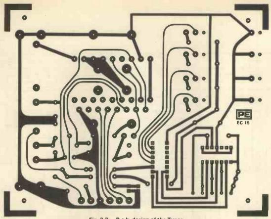
Fig. 2.3. P.c.b. design of the Tuner
