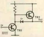
Fig. 4, Basic Class A stage with an emitter follower
