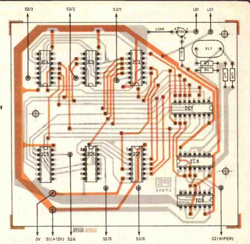
Fig. 4. Component overlay of p.c.b.
