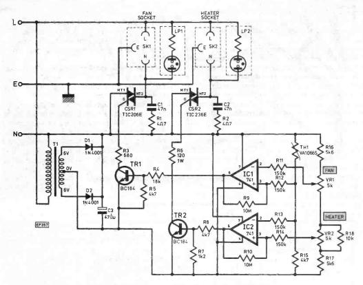
Fig. 1. Circuit diagram of the Temperature Controller
