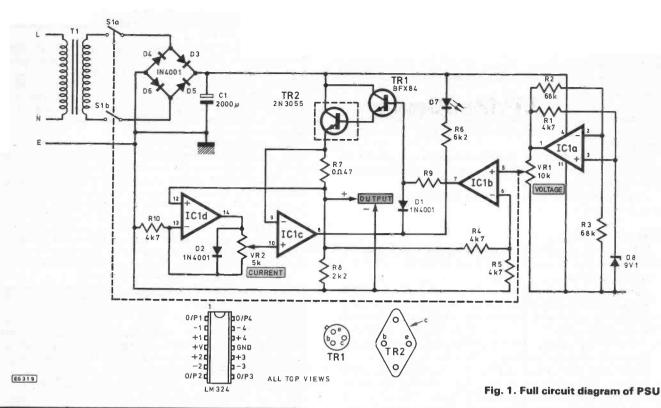
Since the voltage drop across R7 is directly proportional to the current being taken by the load, and since the pot track is linear, it follows that this can easily be calibrated.
