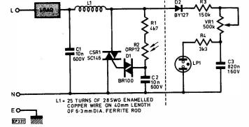
The remainder of the circuit is a basic neon oscillator where D2 rectifies the a.c. and VR1 controls the rate at which the neon flashes.
