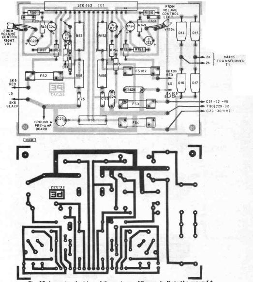
Fig. 15. Layout and wiring of the main amplifier p.c.b. Note the ground A link to the pre-amp board and the wire link from G to G
