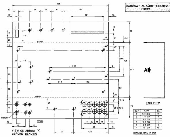
Fig. 16. Drilling and bending diagram for the chassis. It is suggested that mounting holes for the p.c.b.s are marked through the board fixing holes with the boards in place to ensure accurate alignment. If the holes are marked out after bending 1.5mm should be added to all dimensions taken from the bends, all measurements to be made on the outside of the chassis
