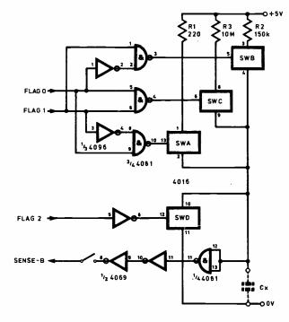
Fig. 1. Auto-ranging digital capacitance meter interface circuit
