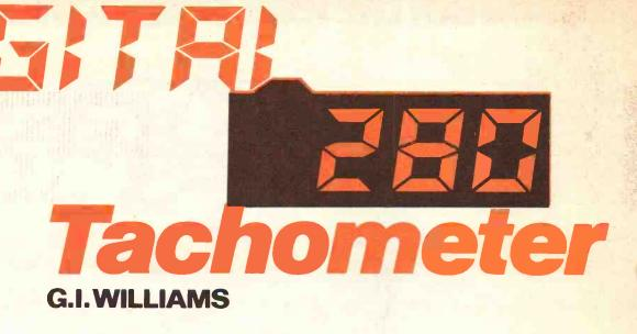
THIS instrument was designed as a general purpose tachometer for measuring shaft speeds of rotating devices between 0 and 10,000 r.p.m. and has proved useful both in the laboratory and workshop.
