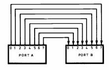
Fig. 7. Connection between two 8-bit ports to implement a 'reverse' instruction
