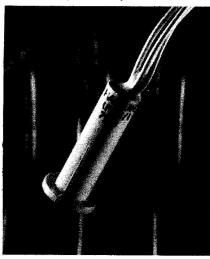
The switch measures 28mm in length  $\times$  7.62mm in diameter, and is supplied with two pairs of leads; one pair can be looped back into the circuit. Four reed-switch options are available: low-cost Form A (normally open); standard Form A; high-power Form A; and standard Form C (single-pole/double-throw).
