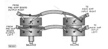
Fig. 13. Wiring of the volume and balance controls
