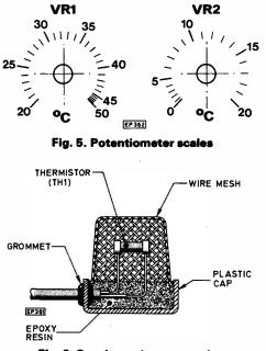
Fig. 6. Sensing unit construction
