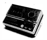
In use the capacitor leads are simply inserted into a pair of slots and the capacitance is indicated on the clear 4-digit l.e.d. display. A flashing display provides over-range indication. Provision is also made for using jack plugs when measuring in-circuit capacitances.
