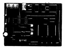
Circuit Mount prototype boards are available in a range of sizes from small modules designed to hold a single i.c. up to 1020 point panel-mounted boards complete with binding posts. All separated modules are interlocking and also feature screw holes for permanent mounting.
