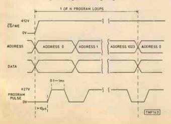
It should be noted that the machine described here is *not* suited to the *single supply* 2716, nor types of EPROM other than 2704, 2708 and the multi-supply 2716. The reason for this is that the cycle-timing diagram requirements are quite unique to this family.
