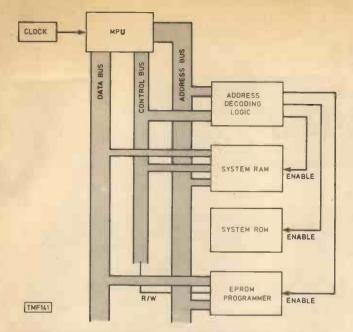
Fig. 1. Minimal system containing EPROM Programmer
