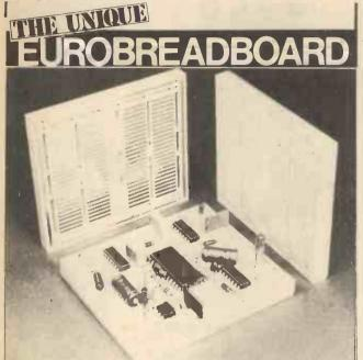
Logically laid out to accept both 0.3" and 0.6" pitch DIL packages as well as Capacitors, Resistors, LED's, Transistors and components with leads up to .85mm dia.
