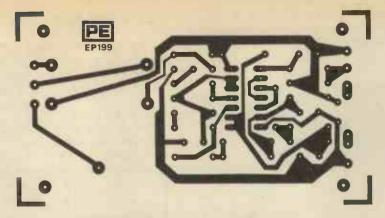
Fig. 5. P.c.b. design for the Control Unit
