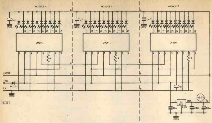
Fig. 4. Extended Bar mode display
