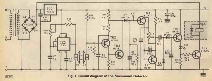
picked up by the receiver X2 and amplified by TR2 and TR3 with resistor R14 providing 100 per cent feedback making this stage very stable. The a.c. gain of the stage is determined by C8 which shunts the high frequency signals in the feedback path therefore increasing the gain of the stage( 50 times the input voltage at 40kHz).
