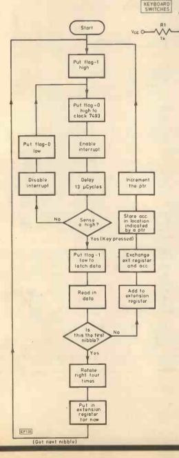
THIS circuit is for an experimental hexadecimal keyboard for use with National Semiconductor's SC/MP microprocessor. Using four popular TTL i.c.s it represents an interesting example of the hardware/software trade-off in MPU systems. If built with one of the surplus calculator-style keyboards advertised regularly in *P.E.*, total cost should be under £5. Use of 74LS series TTL is recommended.
