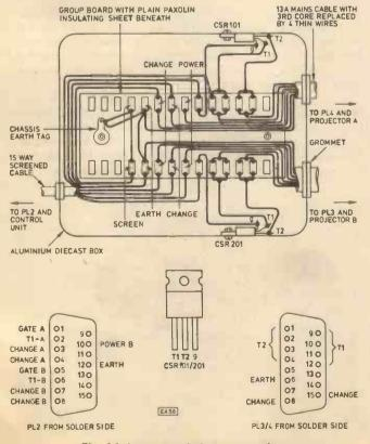
Fig. 14. Layout and plug connection
