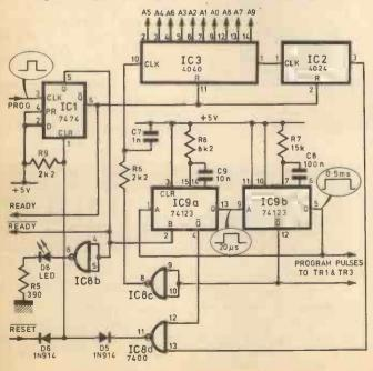
The 27 volt pulse, in particular, must *never* be applied unless the others are present exactly as required in the timing diagram, and certainly should never be applied for more than 1ms continuously.
