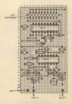
Fig. 5. Alternative stripboard layout
