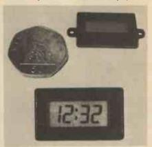
day and date. The unit is quartz controlled, has a back light, and an alarm function to drive a bleeper or other indicator. Running consumption is  $6\mu$ A, accuracy is within  $\pm 2.5$ minutes per year, and height of the characters is up to 0.5in. The display shown has a character height of 0.25in. Price is £10.60 inc. VAT and p&p.
