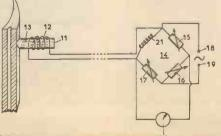
frequency of around 5kHz. The signal is applied via resistor R1 and thermistor T1 to compensate for any small change in the value of capacitor C1 caused by temperature. Because a relatively low frequency sine signal is used, oscillator 15 can be placed up to 500 feet from sensor electrode 11 without significant loss.
