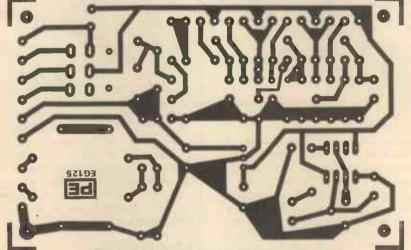
Fig. 3. P.c.b. design for the Movement Detector
