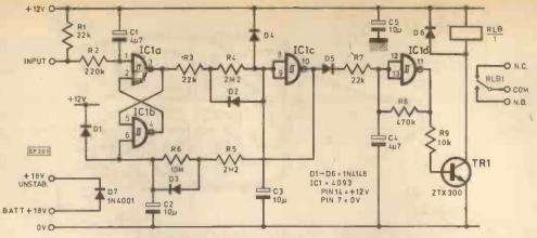
Fig. 2. Circuit diagram of the Control Unit
