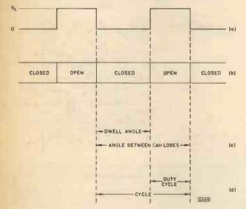
Large dwell angles will result in overloading of the capacitor and burning of the contact breaker points at low speeds. Too large a dwell angle is usually due to the gap of the contact breaker being set too small.
