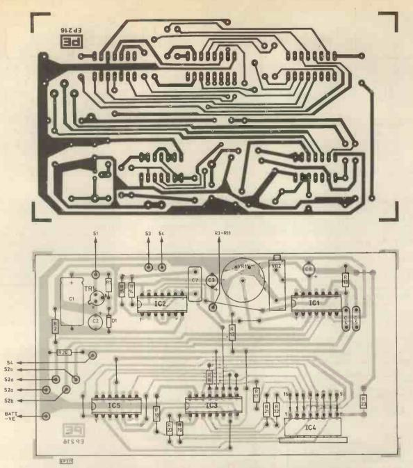
Figs. 3 and 4. P.c.b. and component layout. Arrows refer to display pin connections. For these see circuit
