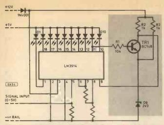
Fig. 1. Circuit to provide Dot-to-Bar mode changeover triggered by I.e.d. 8
