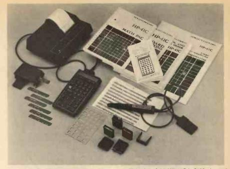
only to execute the program and not allow alterations. The thermal printer can print numbers, letters (upper and lower case), special characters, graphics and produce high resolution plots from data of programs.
