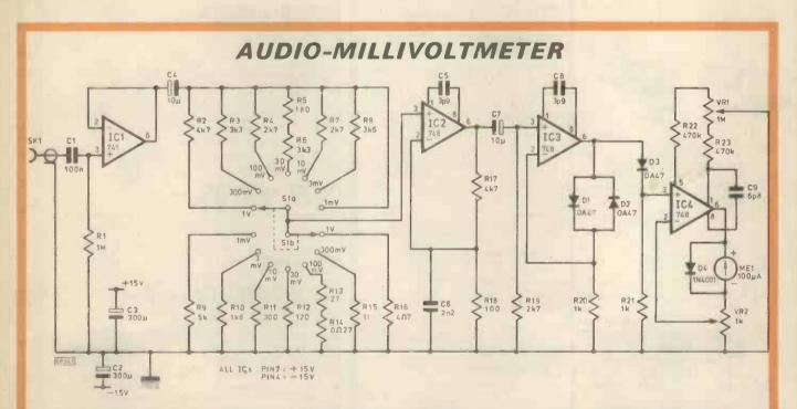
AVING constructed the audio-millivoltmeter featured in the June '76 edition of *PE*, I discovered that circuit noise and main's hum caused a permanent deflection on the meter that was unacceptably large on the lowest range. To cure this I devised this circuit.
