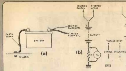
Fig. 1. (a) Conventional car battery connections; (b) Equivalent circuit of the battery earth strap
