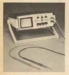
The Tracker uses a scope display, two nonpolarised leads and three impedance ranges. The scope display show the condition of the device under test indicating "shorts", "opens" and "leaks". Both the forward and reverse response of the component can be displayed on the scope screen.
