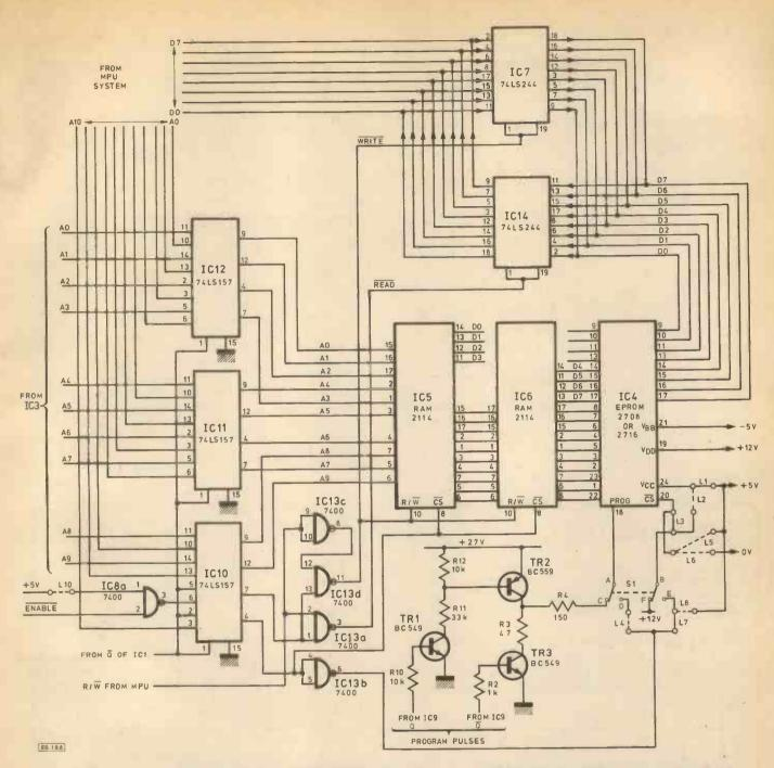
Fig. 5. Memory and switching of the Programmer. S1 is in the "Program" position. Links are shown connected for 2708
