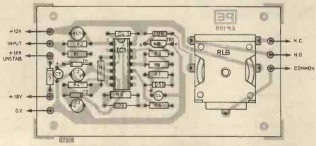
Fig. 6. Component layout of the Control Unit
