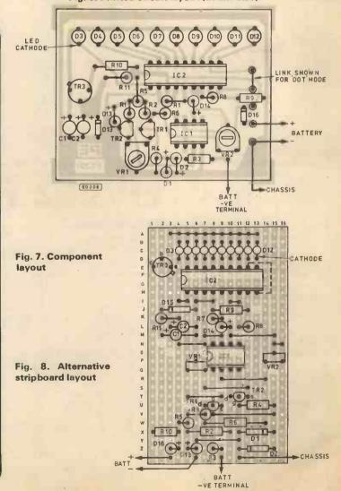
that the circuit functions correctly before wiring to the vehicle. With the 1k variable resistor set to mid-position, VR1 should be adjusted so that D7 just extinguishes and D8 just becomes illuminated. Moving the variable in one direction should cause the green l.e.d.s (D8 to D12) to illuminate successively and in the other direction the red l.e.d.s (D3 to D7) should illuminate successively. VR2 should be adjusted so that the whole range is covered.
