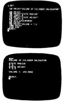
The listing for program one and its execution is shown above. If your machine has  $\pi$  in memory, only the actual symbol need be included. As the sign for raise to the power is  $\Lambda$ , statement 70 can be reduced to  $\pi \circ \mathbb{R} \Lambda 2 \circ \mathbb{H}$ .
