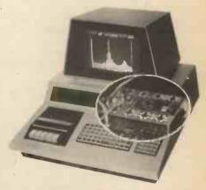
The manufacturers suggest that the plug in board can be used for measuring sound and noise levels, for optimising the equalisation of a hi-fi or public address system, for checking the frequency response of audio components, and for speech and sound pattern recognition.
