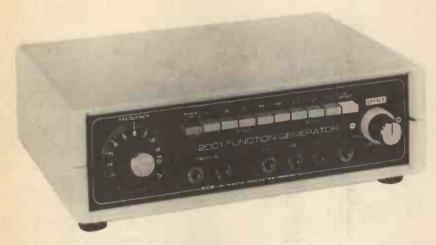
The variable d.c. offset amplitude control, once set, holds the output signal to within ±0.5dB over the entire frequency range.
