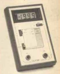
The instrument has 15 different ranges and can resolve voltage to 0.1 mV, current to  $0.1 \mu\text{A}$  and resistance to  $0.1 \Omega$ . Auto-polarity and auto-zero are standard. Inputs are via 4mm terminals and are protected against overloads and transients.
