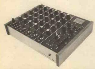
(Above) Prototype control panel layout. In the modified design the limiter switch is excluded. (Below) Headphone outlet is on the front panel with inputs to the rear
