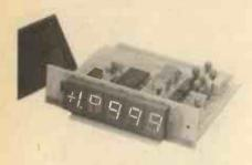
Accuracy is guaranteed to  $\pm 1$  count over the entire range, giving a resolution of up to  $10\mu V$ . Auto-polarity, auto-zero, b.c.d. outputs, digital hold and programmable decimal points are standard features.
