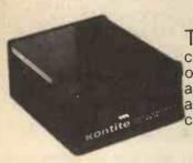
The Receiver: contains input and output cables which are connected to the appliance to be controlled.
