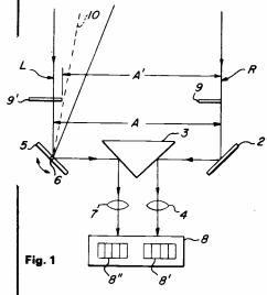
As shown in Fig. 1, two mirrors 5,2 are spaced apart on the camera front and thereby "see" slightly different images of the scene to be photographed.
