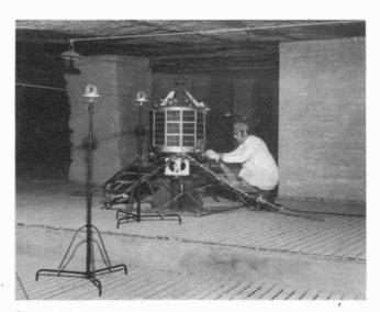
The Ariel 4 satellite being tested prior to launch. The receiving aeriels of some of the experiments are visible. (By courtesy of British Aerospace)
