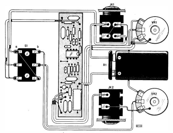
Fig. 5. External assembly to board
