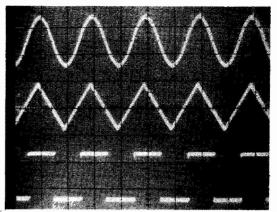
Sine, triangular and square wave outputs at 1kHz. Vertical scale: 2V/cm; Horizontal scale: 500µs/cm
