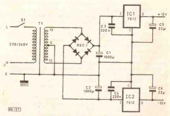
Fig. 1. Circuit diagram of the power supply
