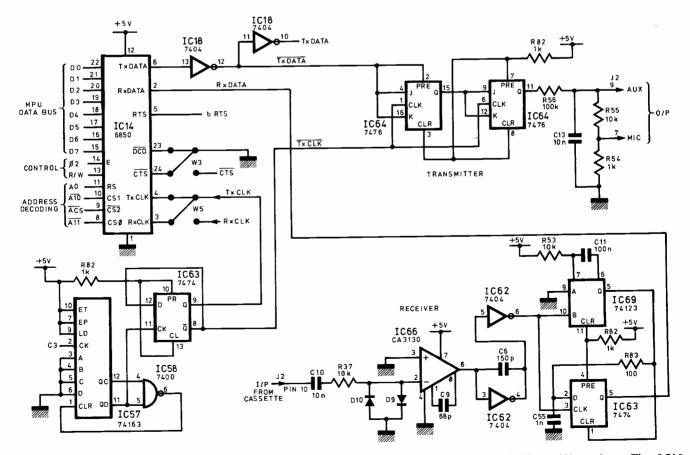
Fig. 2.3. Cassette Interface. 7400 series devices are LS types. Printed circuit ''patch-panels'' have W numbers. The ACIA signals \$2 and R/W go to expansion socket pins 31 and 32 respectively
