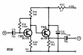
Fig. 4 Output and echo send amplifiers (3 required)
