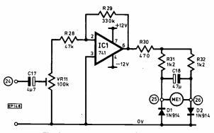
Fig. 6 VU meter amplifier (2 required)
