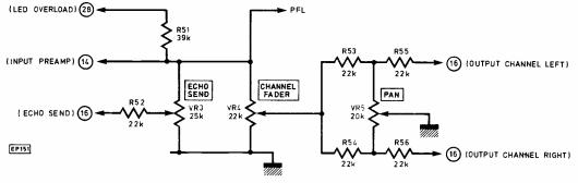
Fig 3 Pan pot and mixing network
