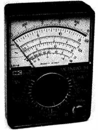
Despite the simplicity of it's design the meter offers no less than 36 ranges with a  $20k\Omega/V$  sensitivity, at just £22.00 plus VAT & Carr.
