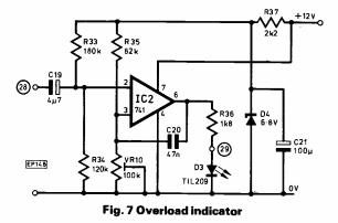
A reference voltage is provided in the circuit by R37 and D4 and decoupled by C21. C20 provides positive feedback at high frequencies causing the op amp to switch more rapidly. The preset pot VR10 adjusts the switching level and hence the level of input signal which illuminates D3.
