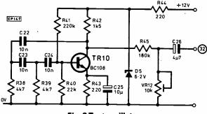
Fig. 8 Test oscillator
