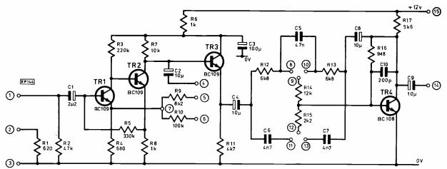
Fig. 2 Preamplifier and tone controls (6 required)
