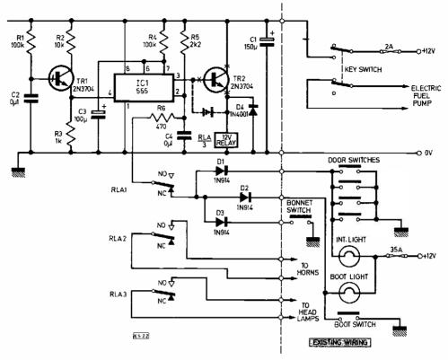
THE circuit will give both visual and audible warning of unlawful entry into your motor car, which should deter the car thief. If your car is fitted with an electric fuel pump, then this may be immobilised when the alarm unit is switched on. The alarm is essentially an electronic version of the more common mechanical alarms, based on a relay latch, in conjunction with a thermal delay switch, and costing over double the outlay for this unit.
