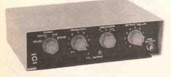
and fine frequency control is achieved by varying the d.c. potential at pin 8 of the 8038. Two pre-set resistors, VR2 and VR3, are used to set the maximum and minimum frequencies respectively at each end of VR1. Adjustment of the purity of the sine wave output is provided by VR4 and VR5. The desired output waveform is selected by S2 and fixed resistors, R4, R5 and R6, are included to provide equal peak-peak outputs with all three waveforms.
