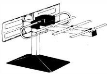
Although called a set-top aerial, it can be mounted outside with perhaps a little weatherproofing around the junction box where the co-ax joins the array.
