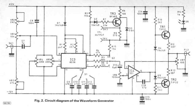
and TR2 is provided by forward biased silicon diodes, D4 and D5.
