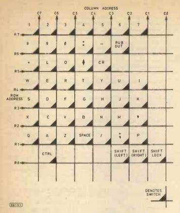
Fig. 3. Above: Keyboard switching matrix
