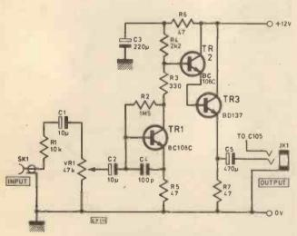
Fig. 1 Single channel of amplifier
