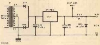
Fig. 4. Power supply circuit diagram
