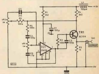
Fig. 1. Circuit of Generator
