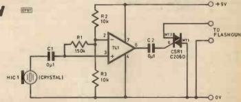
When a sound is made near the microphone, the output of IC1 swings between the supply rails at the frequency of the input. On the first negative going excursion, the triac switches on firing the flashgun.
