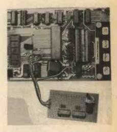
Fig. 7. The Single-Cycler circuit described in the text attached to an MK14 microprocessor kit
