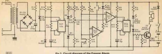
Fig 1. Circuit diagram of the Freezer Alarm.
