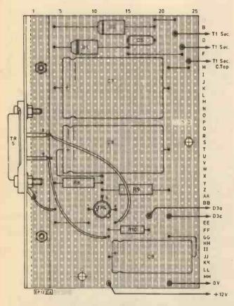
Fig. 4 Layout of p.s.u. board
