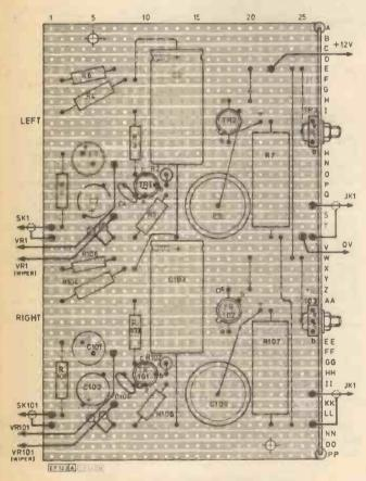
Fig. 3 Layout of stereo amplifier board
