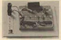
Measuring 11.5 × 14mm the unit is mounted on a baseboard which enables two power terminal connections to be fitted.
