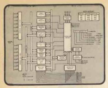
Fig. 1. 6502 internal architecture
