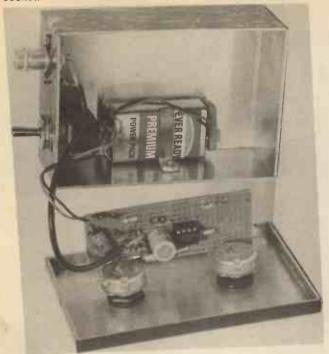
Although the prototype oscillated up to 7.5MHz, it was only calibrated up to 3MHz, because of the cramping of frequency above this. With a little thought, a fine tuning contol could be connected around VR1 to make these frequencies available.
