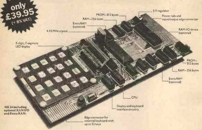
The MK 14 is a complete microcomputer with a keyboard, a display, 8 x 512-byte preprogrammed PROMs, and a 256-byte RAM programmable through the keyboard.
