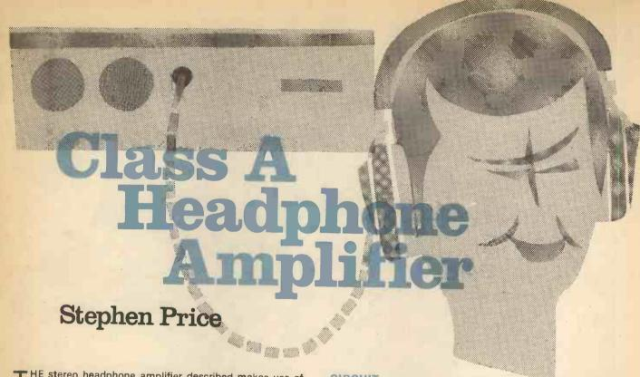
THE stereo headphone amplifier described makes use of a straightforward design specifically intended to drive dynamic headphones with impedances as low as 50 ohms per channel. It includes its own mains power supply and will accept a low level stereo input direct from a radio tuner or tape deck. However, as the basic amplifier does not provide facilities such as source switching, disc equalisation, tone control and filtering it is best suited for use in conjunction with a separate preamplifier.
