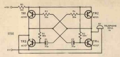
THE circuit shown is suitable for operating a polarised telephone bell from an 18V d.c. power supply (on no account should P.O. systems be interfered with).
