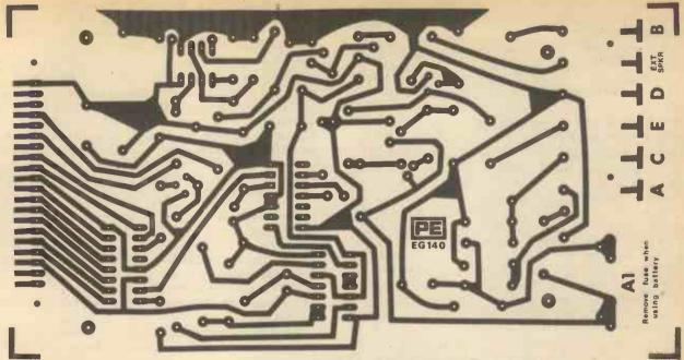
Fig. 3. P.c.b. layout for the Chimesonic
