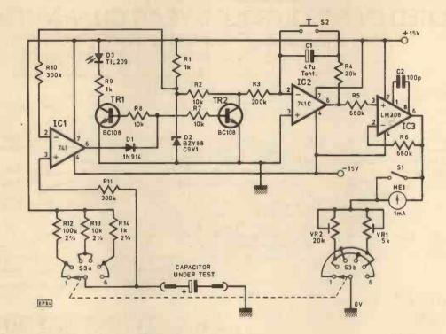
CAPACITORS of values up to 10,000µF can be measured with this instrument, and 6 ranges are available as follows:
