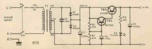
Fig. 2 Power supply circuit for both channels
