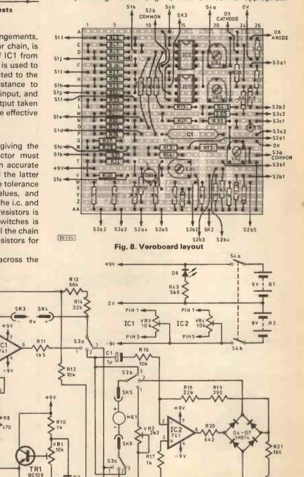
Fig. 6. Complete circuit diagram of the Metermate
