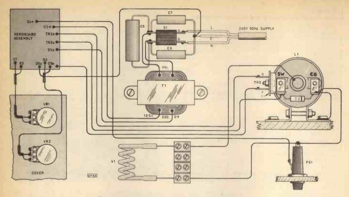
Fig. 4. Component layout and connections to Veroboard
