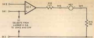
Fig. 7. Effective circuit of the Metermate EG 124
