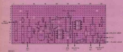
Fig. 3. Stripboard layout of Sound Triggered Flash
