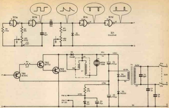
Fig. 1. Circuit of Stroboscope. The arrows on the potentiometers indicate clockwise rotation
