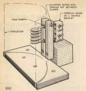
Fig. 7. Showing neon fixing. The centre of the helix forms the reflector focus
