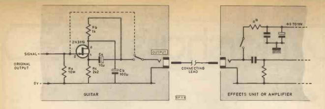
Fig. 7. Installation of a preamp in the guitar, without the need of an internal battery. No isolating capacitor is necessary at the preamp input. The only extra components required in the Treble Boost unit are the switch and 4k7 resistor R<sup>e</sup>
