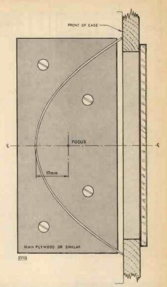
Fig. 6. Template for forming plywood parabolic profile in which reflector is placed. The lid has similarly shaped pieces attached
