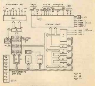
Fig. 1. 1802 architecture diagram
