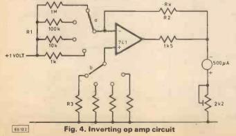
(as the gain is then 1) and is fed to the meter with a  $2 \cdot 2k\Omega$  resistor in series, as in Fig. 4. R3 is switched so that the impedance at both op amp inputs are approximately equal.
