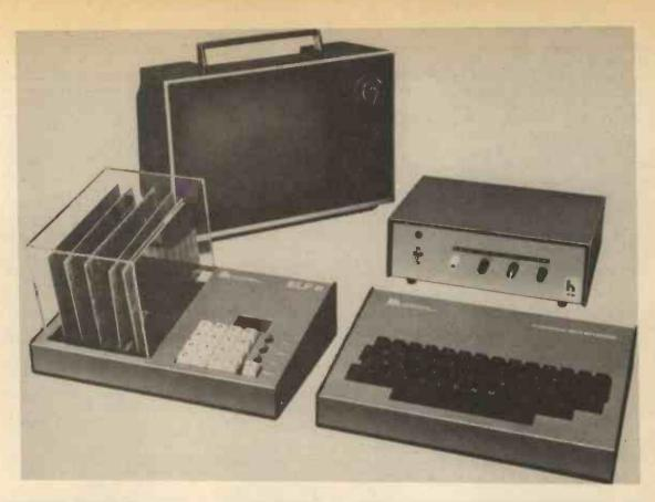
(Above) Elf II with 16K RAM on board, professional ASCII keyboard and power supply
