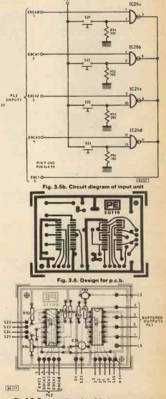
Fig. 3.7. Component overlay of the input-output unit
