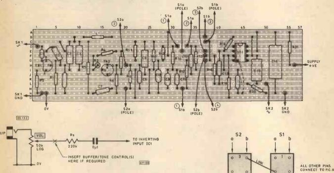
Fig. 4. Suggested arrangement for extra input
