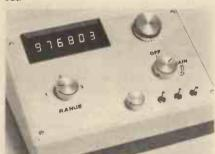
Designed to fit into a single rectangular cutout, the bezel is positioned in the cut-out by four removable location pegs, and firmly secured by two moulded in screwed studs which also secure the display mounting board on spacers provided.
