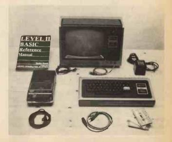
The complete system, showing Level II manual and all interconnection leads.
