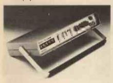
The units are powered from four C size cells and an optional a.c. adaptor is available where continuous use is required. Additional accessories include a rechargeable battery pack, 30kV high voltage probe and an "eveready" carrying case with a neck strap.
