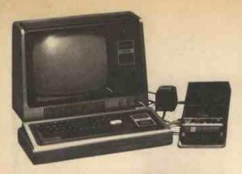
The Tandy TRS 80 which is supplied complete with a video monitor, mains transformer and cassette recorder
