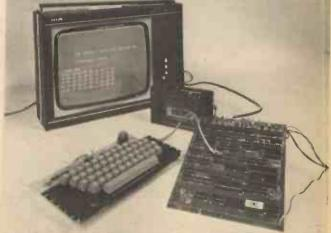
The Nascom I is supplied in kit form and requires a power supply and VDU for operation
