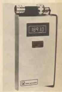
Being touchless, the tachometer can be used in places awkward to reach, and there is a 24in cord attached to the probe. The readout is quartz crystal controlled, with an accuracy of  $\pm$  1 digit up to 0.03 per cent. There is direct reading up to 30,000 r.p.m.
