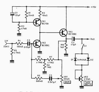
Fig. 3. Circuit of preamplifiers and fuzz
