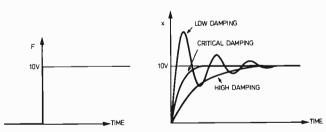
Fig. 4.4. Graph showing the effects of damping after a step function has been applied to Fig. 4.2.
