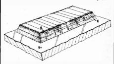
The RCA bipolar transistor is formed from a silicon layer of "n" type which consists of two separate strata which are both epitaxially deposited but differently doped. Using conventional photo, resist techniques the base region is formed by a double ion implantation of "p" type impurity, such as boron.
