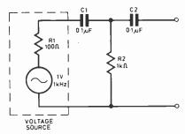
Fig. 9(a). Circuit to which Thevenin's theorem can be applied to get a simpler equivalent
