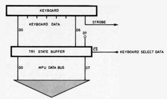
Fig. 5. Simple method of interfacing a keyboard το an ινιτυ system
