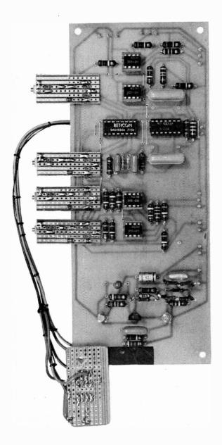
(Left) Main board. Here the cermet multiturn trimmers are mounted on small strips of Veroboard. The small Veroboard at the base is the meter driver circuit
