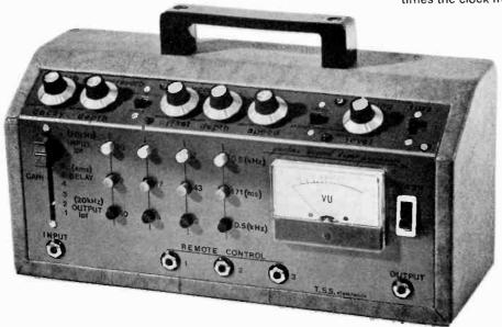
Prototype Sound Multiprocessor. Note the easy accessibility of all controls to the performer
