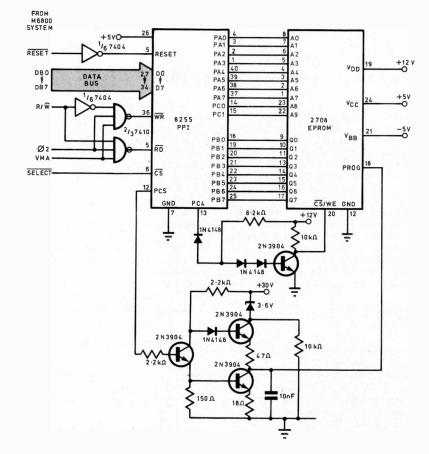
Fig. 2. Programmer for 2708-type ultra-violet arasable programmable read-only memories.
