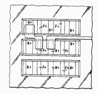
The emitter region is formed by "n"-type ion implanting. This implantation is through an elongated opening in the previously formed silicon dioxide layer. According to RCA this ion implantation technique and multi-strata foundation provides the missing link to reliability.
