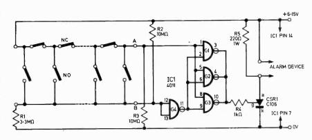
This circuit features high sensitivity with an extremely low current consumption—under 3µA at 12V. The circuit is so sensitive that a finger placed on each guard line will set the alarm off.
