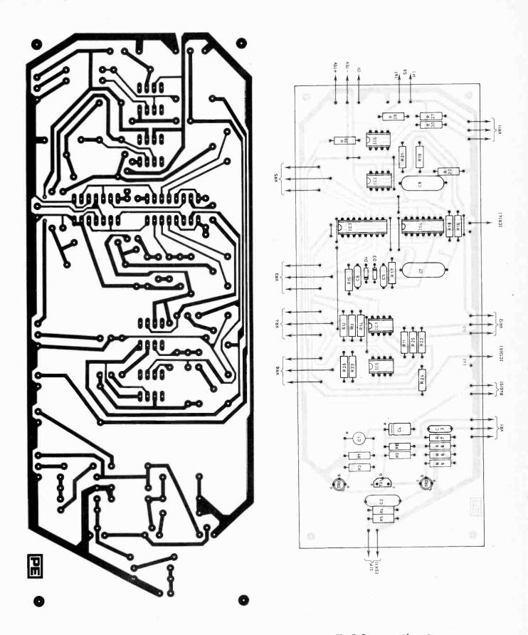
Fig. 4. Printed circuit of main board
