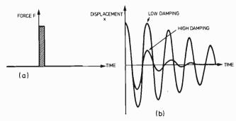
Fig. 4.3. The graphic representation of an impulse function is shown in (a). Graph (b) shows its effect on the circuit in Fig. 4.2.
