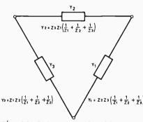
Fig. 14. Delta network with star to delta conversion formula
