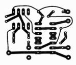
Fig. 2. Printed circuit layout (actual size)
