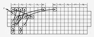
Fig. 4.2. Flow diagram and patch panel layout for investigating a damping system.
