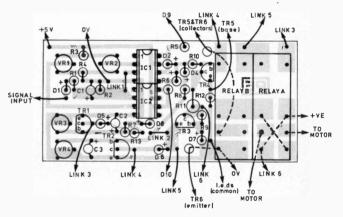
Fig. 3(a). Component layout. IC1 and IC2 may be plugged into a single d.i.l. socket
