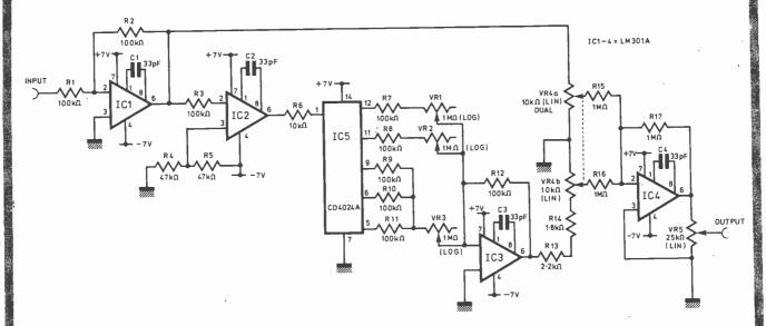
S HOWN is a circuit for a sub-octave generator, developed for use with a synthesiser. It functions as follows.
