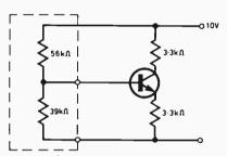
Fig. 10(a). Typical biasing stage
