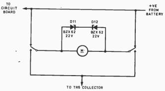
Fig. 5. Clamping diode circuit to suppress motor interference.
