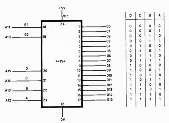
Fig. 1. Using a 74154 to decode the address lines thus generating the necessary  $\overline{\text{CS}}$  signals
