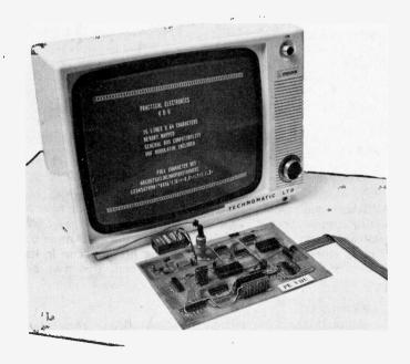
THE "PE VDU" is a complete output peripheral for MPU systems, and will interface easily to any data bus and address bus, including the 6800, Z80, 8080, and SC/MP systems such as the Science of Cambridge MK14.
