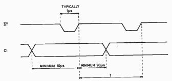
Fig. 2. Timing diagram for CO, C1, C2 and ST lines
