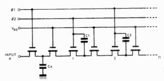
Fig. 1. Section of SAD 1024 equivalent
