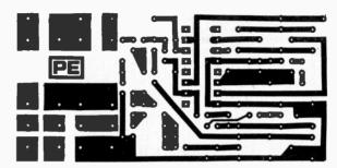
Fig. 2. Printed circuit layout shown at full size
