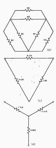
Fig. 15(a-d). All of these circuits are equivalent
