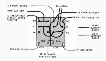
Fig. 4. Relay wiring arrangement for the standard configuration of two-pole change-over type relays.
