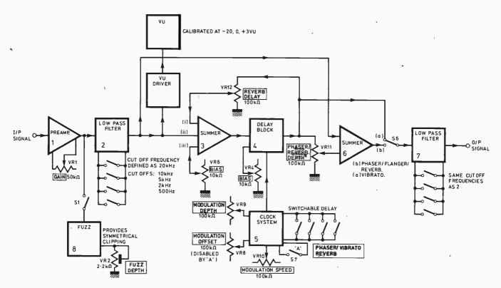
Fig. 2. Block diagram of the Sound Processor
