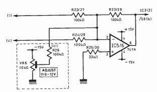
Fig. 7. Circuit of Summer 3. Summer 6 is identical apart from the exclusion of the boxed circuit
