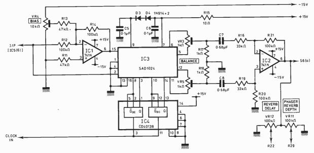
Fig. 6. Circuit of delay block
