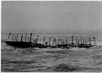
Above: One-tenth scale Wavepower Raft under test in the Solent
