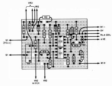
Fig. 2. Stripboard layout shown at full size. Note that C1 is not shown on this diagram
