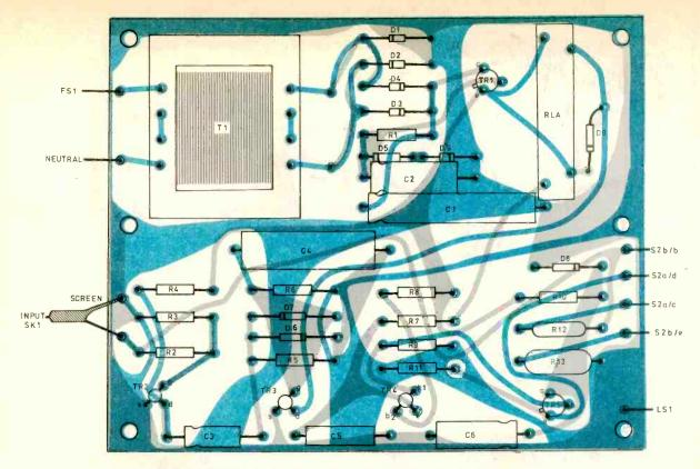
Fig. 5. Component assembly in double sided p.c.b.
