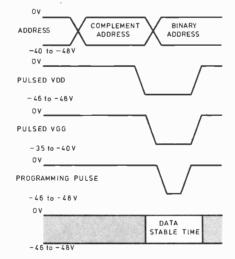
that the program pulse is a 3ms -47V pulse as required. As with many things in electronics, the secret lies in viewing the circuit. operation with one's feet firmly on the ground (or in this case, the ceiling!). If you check the other supplies with this new perspective, you will find that they are substantially as dictated in the data sheet.
