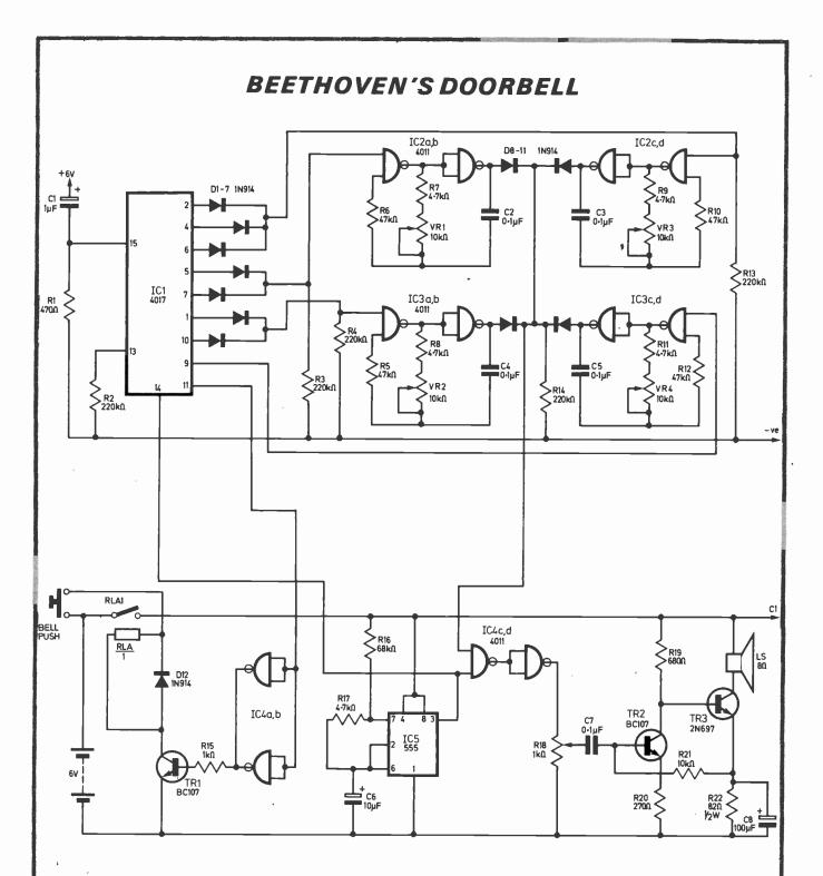
This circuit was developed from the doorbell published in *Practical Electronics* April 1975, using CMOS which were to hand, and plays the first eight notes of the Beethoven "Ode to Joy" theme. Clock pulses from IC5 are fed to the 4017 decimal counter IC1, which is reset by CI/RI at switch on. The "0" output is not used as the first clock pulse is
