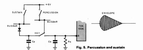
A combination of Percussion and Sustain is shown in Fig. 5. One capacitor now loads the other, so that staccato playing will produce a larger output than legato. Because the TDA 1008 gives an output voltage that is proportional to the input, we now have touch-sensitivity. The effect is similar to an acoustic piano with "loud" pedal in operation.
