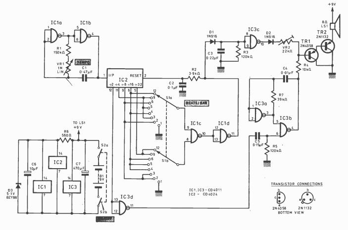
Fig. 1. Full circuit diagram of the Metronome
