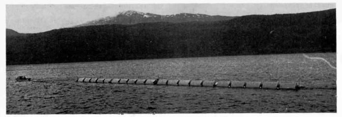
At Edinburgh University where the Salter Duck was originally developed, study is now concentrated on the theoretical and behavioural nature of the machine. On a more practical level at Lanchester Polytechnic (Coventry), Sea Energy Associates build scale models for testing. Shown above are one-fifteenth scale machines (50m string with 30 tonnes displacement) undergoing trials on Loch Ness. Illustrations courtesy of Lanchester Polytechnic
