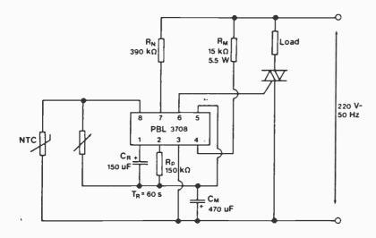
A typical design for control of room temperature with a heating element of 1,000W, 220V a.c. and a proportional band of 1°C.
