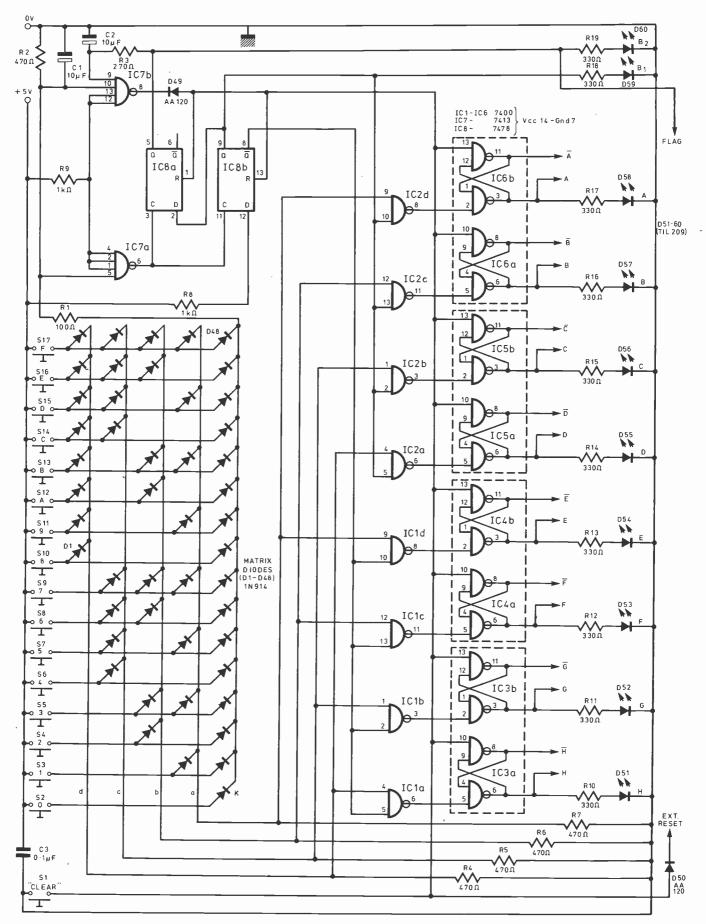
Fig. 1. Keyboard electronics
