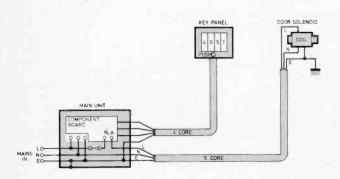
Fig. 3. Wiring diagram of solenoid circuit. Care should be taken when wiring up this mains portion of the system
