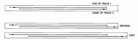
Fig. 1. Showing how copy tracks go out of sync
