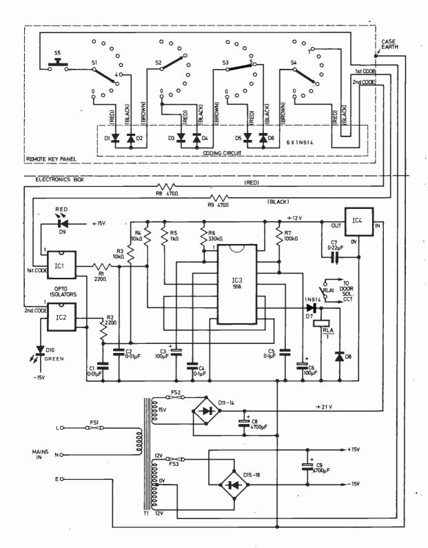
Fig. 1. Full circuit diagram including suggested power supply arrangement
