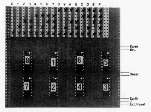
Fig. 3. Showing the connection of the matrix diodes and i.c.s
