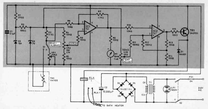
Fig. 1. Full circuit diagram, including suggested power supply circuit (shown outside shaded area)
