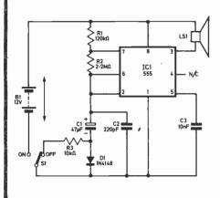
THE enclosed circuit utilises the timing capability of the 555, together with its capacity to directly drive a small audio transducer. It provides an economical arrangement to provide an audible alarm.
