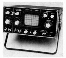
The black 4D10A dual trace scope, at £180, still retains the characteristics of the 4D10; stabilised power supplies in both the low voltage areas and e.h.t. allowing mains variation of as much as ten per cent. Accuracy on both time and voltage measurements is three per cent.
