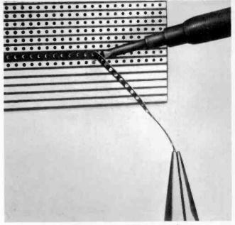
Lifting a copper strip with iron and pliers
