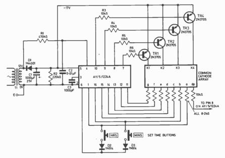
ABOUT 12 to 18 months ago I obtained a small quantity of gas-discharge and l.e.d. displays and purchased a clock chip type AY-5-1224A as it was the cheapest type. I designed a method of driving the gas type displays (normally chips suitable for this cost about £7).
