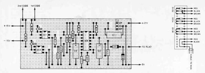
Fig. 2. Stripboard layout of the Combination Lock. The diodes D1 to D6 are mounted separately on a tag board which can be placed next to the code switches. The diode tag board is shown above right
