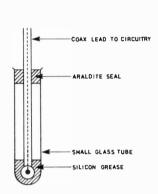
A temperature probe can be fabricated from a small test tube
