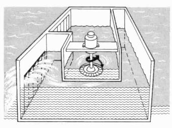
The Russell Rectifier is shown above in both states of flux. (left) The upper chamber fills as the wave rises. (right) The lower chamber empties during the trough of a wave. Courtesy of HRS
