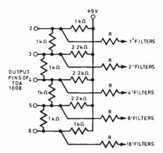
Fig. 8. A method for staircasing the output pitches as an alternative to square waves produced by the simple arrangement in Fig. 1
