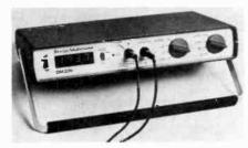
The unit is very light—less than  $1\frac{1}{2}$ lbs—and measures  $255 \times 148 \times 40$ mm. It is powered by four dry cell batteries and optional extras include a rechargeable battery pack, carrying case and a 30kV probe.
