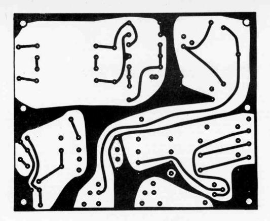
Fig. 3. P.c.b. layout for component side
