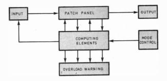
Fig. 1.9. Block diagram of the Analogue Computer
