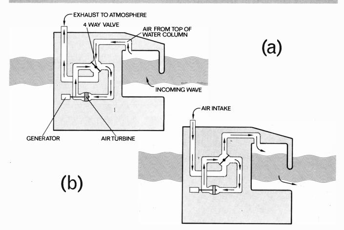
Rectification is achieved by the system shown above, which illustrates the simple OWC principle in its entirety. It employs a kind of pneumatic version of the familiar bridge rectifier circuit. A four-way valve is used to re-route the flow of air in each half cycle so that it always passes through the turbine blades in the same direction. (a) shows the airflow whilst the wave is rising, and (b) shows the situation as a wave trough develops.
