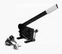
Shock and vibration have caused problems when the spindles of sensitive components have been sewn or cut on a lathe; but the Telpro Shaft Shear may be used to cut the spindles of even delicate helical potentiometers, since it does not transmit shock or vibration.
