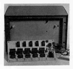
The original front panel is re-mounted internally in the box to provide a base on which to mount the p.c.b. A new front panel is them made of clear perspex and painted, leaving a display window.
