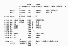
Fig. 2. Program for the M6800 which displays co-ordinate pairs from memory.
