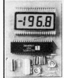
Based on the 7106 single IC 3½ digit D.V.M. the Kit contains a PCB, resistors, capacitors, pre-sets, I.C. and 0.5" liquid crystal display. Components are also included to enable the basic D.V.M. kit to be modified to a Digital Thermometer using a single transistor as the sensor.
