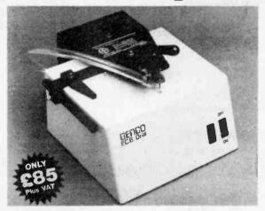
A Printed Circuit Board Drilling Machine, suitable for production or modification of circuit boards. The machine, by way of its kinetic design, is in fact a chuckless Drilling Machine, requiring no guide bushes for the turbo shank tungsten carbide drills.
