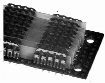
in Fig. 2, and the sharp edges are removed with a file. The socket strips are then inserted in the Veroboard.
