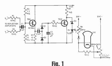
follower drives a voltage doubling rectifier whose output causes the other transistor to conduct should any signal sufficient to deflect the c.r.t. beam be present. If no signal is present the 8.2V Zener conducts and the l.e.d. lights up, its current being limited by the collector resistor of the second transistor.
