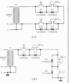
used as the bells will only be on for a very short time. In the same way the transformer voltage can be in excess of the rated value for the bells. In fact it is desirable to run the bells from a higher voltage transformer than recommended by the manufacturers as it is being run from a half wave rectified supply.
