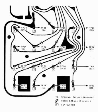
Fig. 5.7. Proprietary p.c.b. inside the Sinclair Cambridge, showing the keyboard end where track cuts are necessary
