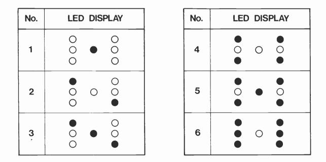
Fig. 2. Showing the I.e.d. display for a count up to six
