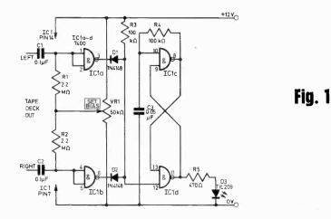
Schmitt triggers (Fig. 1). They have present a d.c. bias which sets the input level at which triggering occurs. Their outputs are fed to a monostable type circuit which lights the l.e.d. in a short pulse for each input peak.
