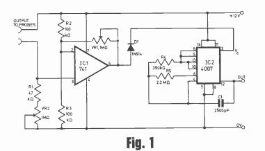
The circuit may be used to monitor changes in skin resistance under stress (or relaxation!) for biofeedback or other purposes. Supply rails down to 6V may be used without any real degradation in performance.
