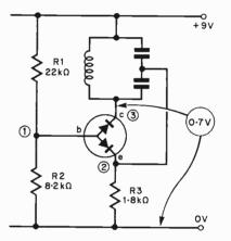
Fig. 1.2. Fault conditions for L1 open circuit
