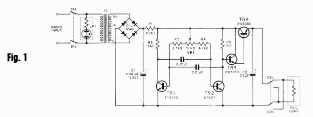
**T** HE main disadvantage with many model train controllers is that they do not give a linear control of train speed. The following circuit gives a linear control enabling the train's speed to be set anywhere between a very slow pace and full speed (Fig. 1).
