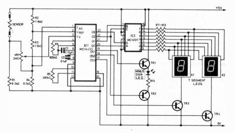
Fig. 1. Circuit diagram for a freezer thermometer using the MC14433
