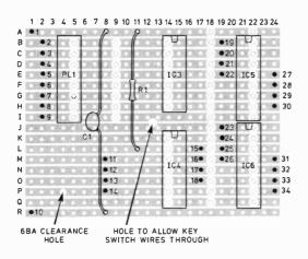
Fig. 5.8. Component layout for Veroboard to be mounted inside the calculator case
