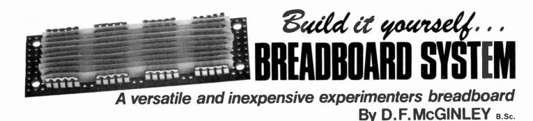
THIS breadboard system is designed to facilitate developing, or experimenting with circuits without the need for continual soldering and desoldering. It not only saves time, but also reduces the risk of burning components and/or fingers.
