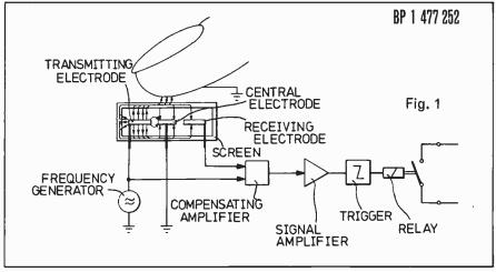
on a load such as a horn) open. When the tip of a finger is moved towards the surface of a metal screen covering the three electrodes, some of the field is diverted upwards by capacitive coupling and this attenuates the signal received. Accordingly, the difference between inputs to the compensating amplifier increases, as does the output. This triggers the changeover of the relay contacts.
