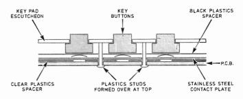
Fig. 5.3. A guide to the basic construction of the Sinclair 0801 keyboard assembly
