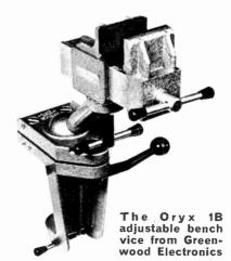
adjustable to rotate through 360 degrees and can be locked in any position. The vice is equipped with nylon jaw linings giving a firm grip with no damage to the work piece. Jaw linings are replaceable. The main components of the vice are cast in high tensile strength lightweight alloy and finished in stove enamelled green.
