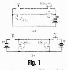
on d.c. so if your bell has terminals marked positive and negative, connect it up as shown. When both switches are pushed at the same time both bells will ring without damage to anything.
