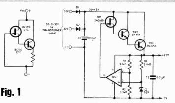
fed either from the crude d.c. at the reservoir capacitor or from a separately controlled supply. An f.e.t. driving the series element overcomes this disadvantage and enables a novel circuit (Fig. 1) to be constructed with both the gate and the reference diode fed from the output. The simple arrangement shown will provide 1A at an output impedance of 50 milliohms.
