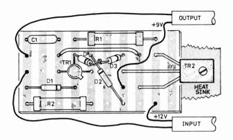
Fig. 2. Veroboard layout and track cutting details
