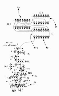
Fig. 8. Component layout of the main board (upper side). Print pattern shown is of the upper side with all underside connections shown with blobs
