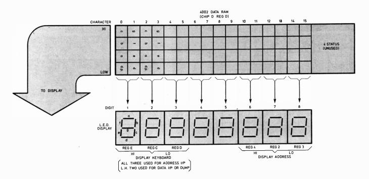
Fig. 5.1. Method of driving the display direct from RAM. A ''replica'' of the energised segments is stored, so that no decoding i.c.s. are necessary. Logic 1 in 4002 = Lo'. Logic 1 on 4265 o/p = Hi' = segment ''on''
