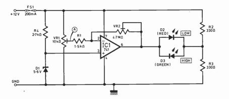
Fig. 1. Circuit diagram of Battery Condition Indicator. (For positive earth vehicles, simply connect the input supply wires the opposite way around, so that the line through FS1 connects to chassis instead)
