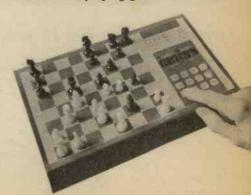
The player enters his move at a keyboard to the right of the chess-board, and the machine gives its reply on a four-digit seven-segment display. The moves are entered as the co-ordinates of the two squares involved (in what is unfortunately the opposite of standard algebraic notation): e.g. FROM 4b TO 4d. The "EN" key then enters the move and the machine replies in about two seconds.
