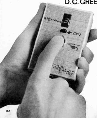
This novel and robust unit was designed to fill the slot requiring simple indication, and not expensive precision timing. Digital operation with numerical display was chosen however, because this eliminates argument over the results. It also precludes the possibility of a declining reading due to a discharging capacitor while the argument takes place, something which can happen with some analogue types.
