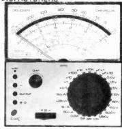
Accuracy: D.C. ranges, ± 2-0%, A.C. & Ω ranges ± 2-5%, 39 ranges: d.c. V, 0-150mV, 500mV, 1-5V, 5V, 15V, 50V, 150V, 500V, 1-5kV, d.c.l, 0-50µA, 500µA, 5mA, 50mA, 0-5A, 5A; a.c. V, 5V, 15V, 50V, 150V, 500V, 1-5kV; a.c.l, 5mA, 50mA, 0-5A, 5A; dB - 10 to + 65 in 6 ranges; Ω 0-05kΩ, 5kΩ, 50kΩ, 50kΩ, 5MΩ, 50MΩ, pF 50kpF, 500kpF,
