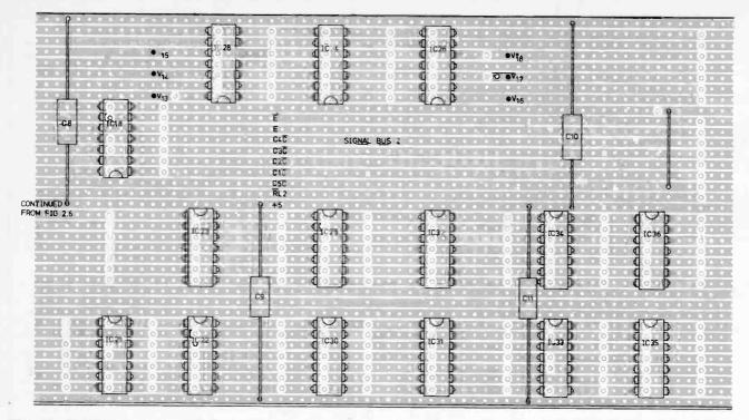
Fig. 3.5. Prototype components layout for the middle third of the main board (section B in photograph). To assemble this constructors should work from the circuit diagrams
