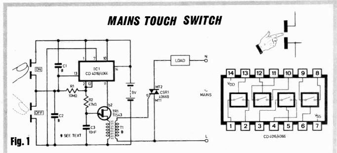
THE circuit diagram of Fig. 1 is for a touch switch offering the advantages of negligible current consumption, complete mains isolation, high noise immunity, great sensitivity and low cost.
