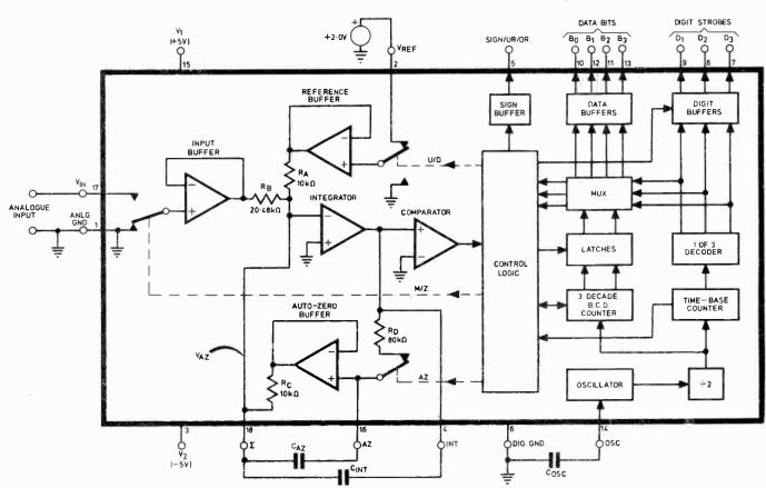
Fig. 1. Internal block diagram of the LD130 DVM chip
