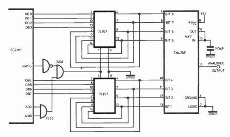
Fig. 1. . Circuit showing a latch formed from a pair of 74157 quad 2-input data selectors
