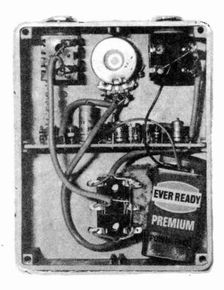
To prevent the unit sliding around on the floor it is a good idea to fix two small rubber feet to the rear of the case lid. This also tips the box forward at a convenient angle for foot operation. Finally glue a small piece of foam rubber inside the lid to hold the battery in place.
