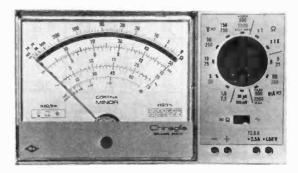
This 33-range instrument uses a Class 1.5 movement with  $20k\Omega/V$  d.c. and  $4k\Omega/V$  a.c. sensitivity. Accuracy is 2.5% d.c. and 3.5% a.c. Self-powered and pocket-sized, the Minor is guaranteed for 12 months and there is an optional 30kV probe available at £9.70.
