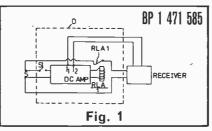
sisting of i.f. or r.f. signals from a receiver, and is connected to power source S through S1. The output of the amplifier supplies the coil of relay RLA1, the relay contact being closed when the coil is not energised. The receiver is thus normally connected to power source S via RLA1.
