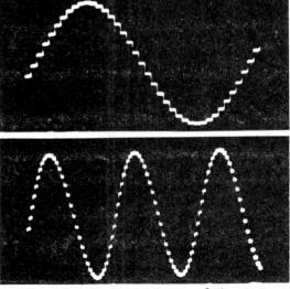
Fig. 3. Oscilloscope traces of sine wave produced from program in Fig. 2
