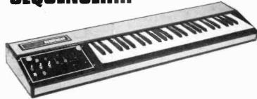
This unit will enable a synthesiser, e.g. PE MINISONIC, to automatically play a pre-programmed tune consisting of up to 32 pitches in a 128-note-long sequence from a single RAM. The note length and the rhythmic pattern can be made variable.
