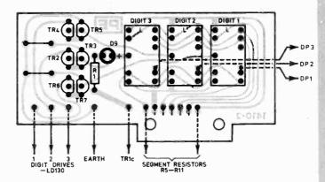
Fig. 7. Display p.c.b. This is mounted on the input socket
