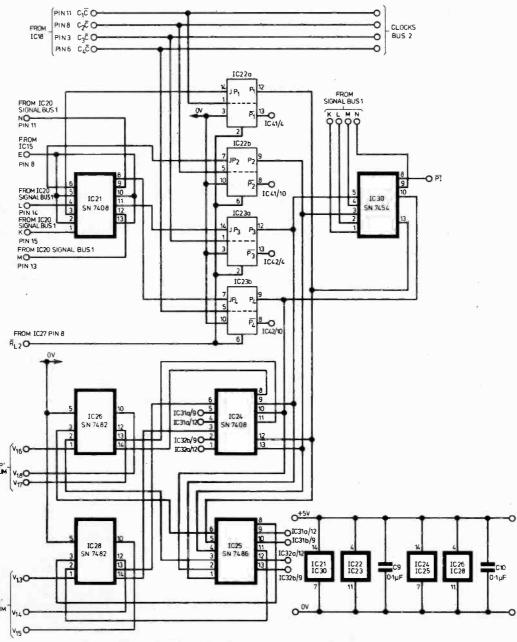
Fig. 3.4. The "P" flip flops and associated logic
