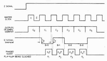
Fig. 3.3. Illustrating the clock phasing
