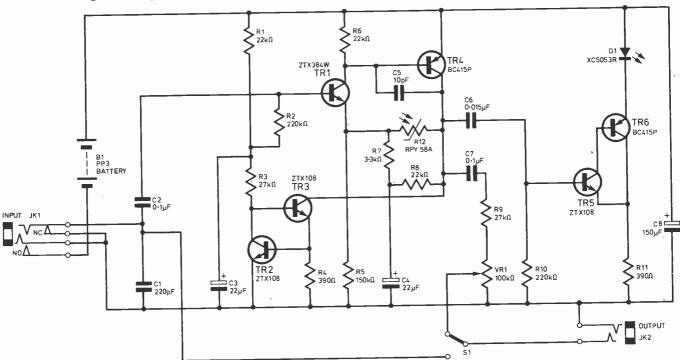
Fig. 5. Circuit diagram of sustain unit
