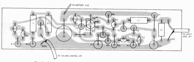
Fig. 7. Component layout and mounting details for D1 and R12 shown above
