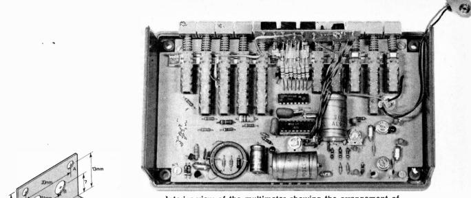
Interior view of the multimeter showing the arrangement of the range switches and segment driver resistors
