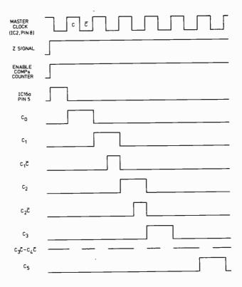
Fig. 3.2. Timing diagram for the comparisons counter
