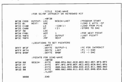
Fig. 2. Program for SC/MP to give a digital approximation to a sine wave
