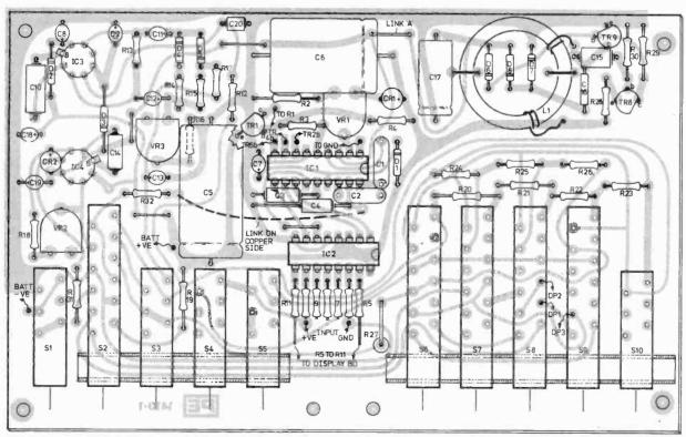
Fig. 8. Main p.c.b. Mounting spacers may be necessary, and may be soldered to the copper cladding
