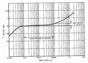
Fig. 3. Output response for different input levels
