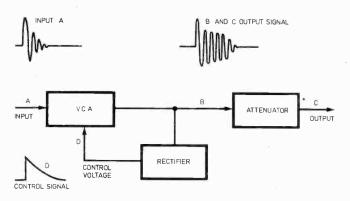
Fig. 2. Block layout for producing a non-distorting sustain unit using a voltage controlled amplifier
