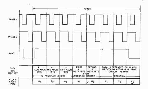
Fig. 2.1. System timing and data bus contents for the 4040
