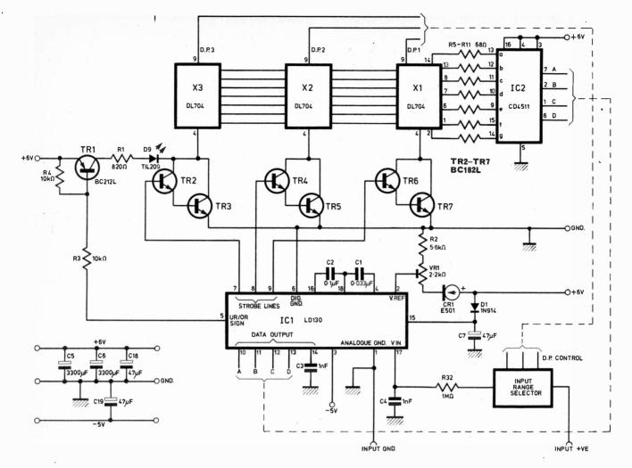
Fig. 2. Circuit diagram of the DMM
