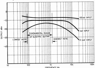
Fig. 4. Frequency response of sustain unit showing how bandwidth changes with input
