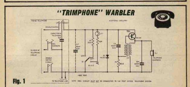
MANY of the surplus telephones available through the secondhand market are sold without bells. The circuit in Fig. 1 will produce a "warbling ring" rather like a Trimphone, and can directly replace a conventional telephone bell, therefore being suitable for both these phones, and for situations where a different ringing sound is required to differentiate between an internal or Post Office telephone system.
