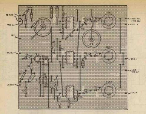
Fig. 2. Component and wiring details of main board. The 0V line is not connected to chassis
