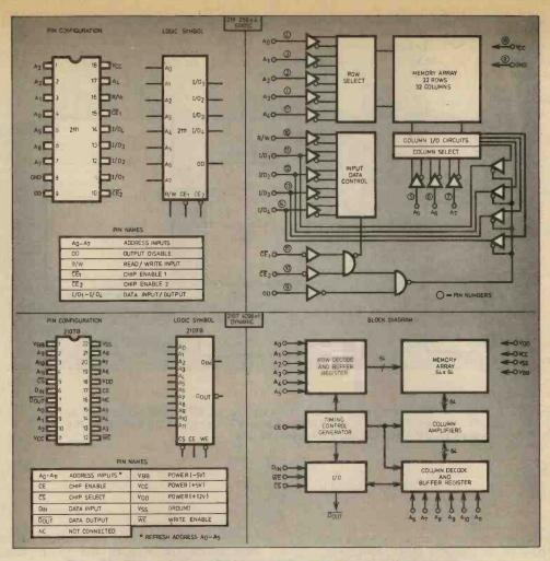
Fig. 4.3 Two useful NMOS RAMS suitable for MPU Systems. The 2111 is a  $256 \times 4$  static device with common data in/out data lines controlled by the O.D. (Output Disable) Pin. The 2107 is a  $4096 \times 1$  dynamic device with four times the capacity of the 2111
