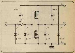
Fig. 2. Improved protection network used on new RCA cos/mos devices
