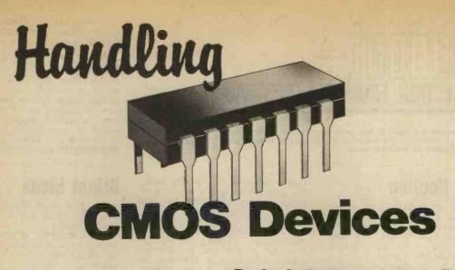
ALL metal-oxide semiconductor devices are susceptible to damage by electrostatic discharge of energy between any two pins. The gate input, for example, is equivalent to a small very low leakage capacitor which can be charged to a high voltage. The dielectric breakdown voltage is normally of the order of 80V, therefore, any discharge above this level could damage the gate oxide and result in a high leakage input.
