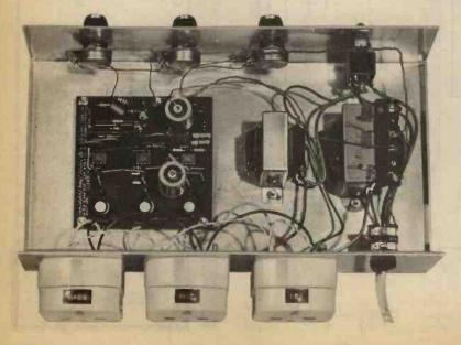
Showing the case assembly of the unit. Note the push fit heat sinks on the s.c.r.s
