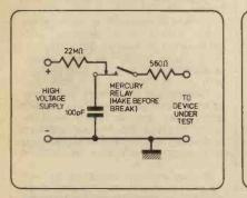
Fig. 3. Equivalent "body discharge" circuit used at RCA during all static test measurements
