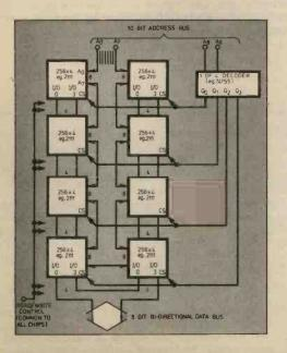
Fig. 4.2. Using the "Chip Select" inputs to build large memory arrays. This is a  $1024 \times 8$  bit memory with Intel 2111 256  $\times$  4 static RAMS
