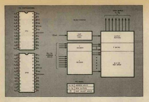
Fig. 4.4 The 2704 and 2708 are state of the art EPROMS organised as  $512 \times 8$  and  $1024 \times 8$  respectively. Erasure is achieved by exposing the chips to UV light via their transparent lids
