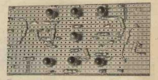
The seven l.e.d. assembly with its resistors is mounted on its own Veroboard. The board is fixed by pushing the l.e.d.s through mounting clips
