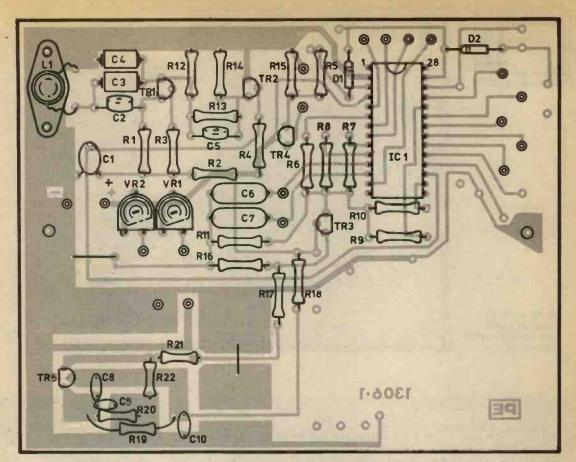
Fig. 11. Printed board component layout
