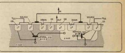
Fig. 4. Parasitic bipolar transistors in cmos circuits
