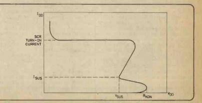
Fig. 6. Curve illustrating effect of secondary breakdown and s.c.r. latch-up
