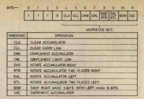
Fig. 2. An example of the IM6100 microcode format
