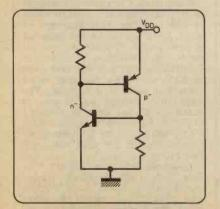
Fig. 5. Equivalent circuit for the s.c.r. structure present in CMOS circuits
