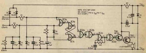
Fig. 1. Circuit diagram of the unit, negative earth version
