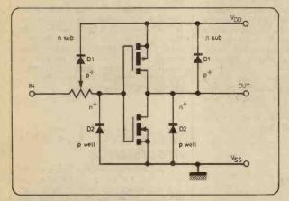
Fig. 1. Standard RCA protection network; used on all CD4000A and some CD4000B series devices
