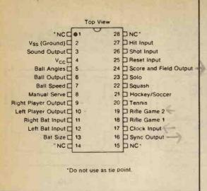
Fig. 7. AY-3-8500 pin configuration
