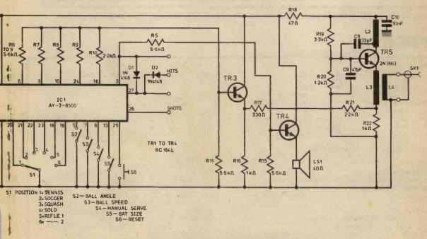
Fig. 9. Circuit diagram of the Sportcentre
