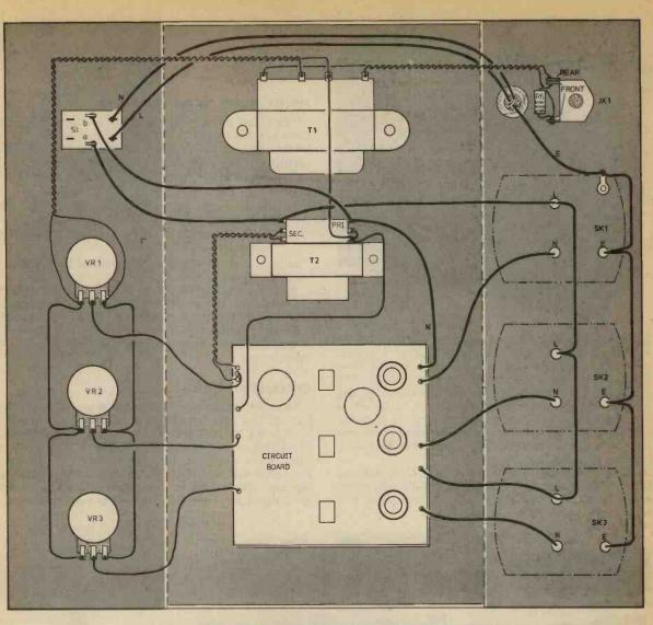
Fig. 3. Component interwiring to the board
