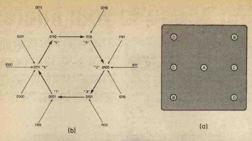
Fig. 2(a). Seven I.e.d,s are required to indicate the six states of the die. There are sixteen possible conditions presented by the four binary counters to the I.e.d.s. Each condition can be represented by the binary word DCBA. The words that relate to die 'number' configurations are shown in the central 'cycle' (Fig. 2b)
