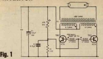
Potentiometer VR1 determines the output power. This circuit can accommodate npn or pnp transistors simply by changing the polarity of the supply and capacitor C1. I. P. Kemp, Cowley, Oxford.
