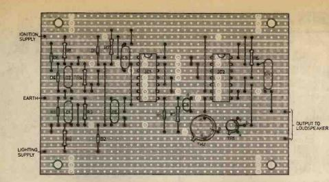
Fig. 2. Component layout on Veroboard, negative earth version
