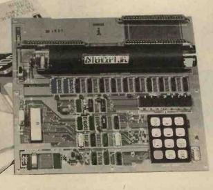
THE Intercept Junior Is a "stripped down" microprocessor development and tutorial system which features the unique Intersil IM6100 CMOS microprocessor chip in a versatile and expandable "no frills" design.
