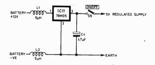
Fig. 4. Circuit diagram of the 5V regulator section. The chokes suppress transients in the leads
