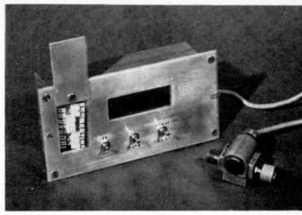
The completed unit showing the pulse sender unit and the cutouts for the displays and switches S2, 3a-d
