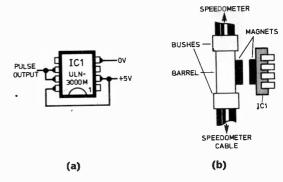
Fig. 1. Details of the pulse sender unit. (a) shows the pin connections to the ULN-3000M Hall-effect i.c. and (b) shows the method of mounting in the T-piece
