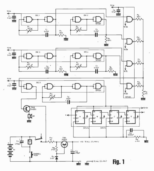
THE electronic doorbell to be described uses five separate oscillators, one for each note of the tune, and one for the clock generator which governs the speed at which a four-note tune is played. Each oscillator uses two NAND gates, each gate generating the NOT function. These are arranged as shown in Fig. 1.
