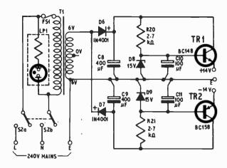
Fig. 3. Power supply circuit
