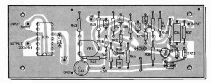
Fig. 14. Layout of the buffer and calibration circuits on the printed circuit board
