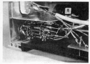
The input socket screen and attenuator resistors mounted on the selector switch
