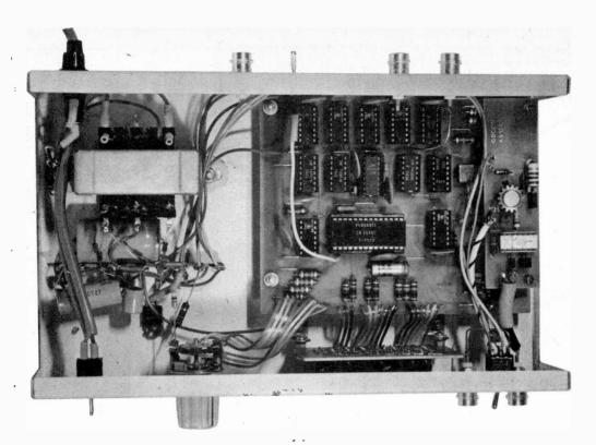
The completed frequency meter with the pre-scaler mounted in position on the right
