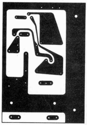
Fig. 5. Details of power supply p.c.b.
