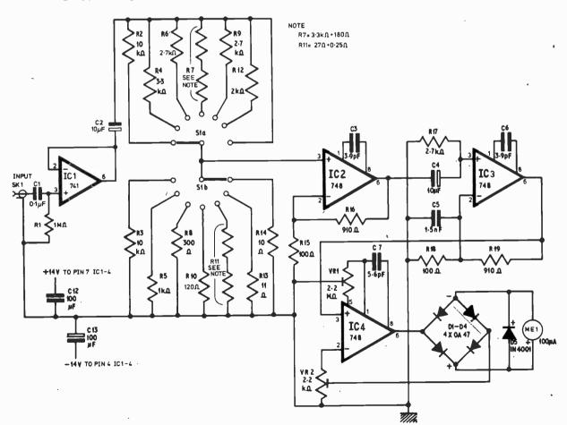
Fig. 2. Circuit diagram of the Audio Millivoltmeter
