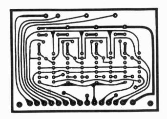
Fig. 1Q. Full size printed circuit master of the display board
