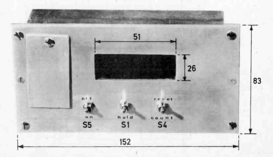
Fig. 5. Front panel details and overall measurements. The dual-in-line switches cutout measures 32  $\times$  45mm
