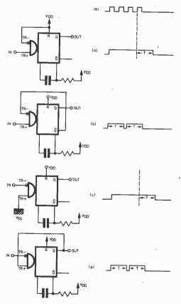
Fig. 6.2. The four possible modes of operation of the 4098/4528 monostable, and the four outputs obtained with the input shown
