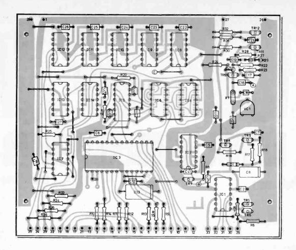
Fig. 7. Layout of the components on the main printed circuit board. Note that if the high impedance buffer is used then C1 and transistors TR5 and TR6 are not required. The three signal test points in Fig. 2 are marked as "A", "B" and "C". I.C. sockets should be used especially for IC3 as replacing a faulty i.c. is difficult
