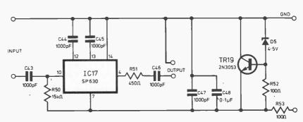
Fig. 17. Circuit diagram of the VHF Prescaler
