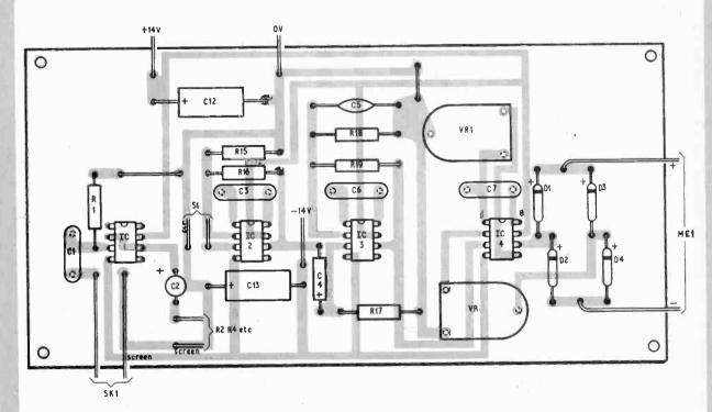
Fig. 4. Component layout and p.c.b. master for main board
