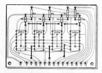
Fig. 9. Layout of the components on the display board. The 15 pads are wired to pads with the corresponding numbers on the main board
