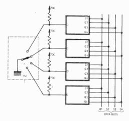
Fig. 6.8. Common bussing illustrated with hypothetical devices (such as the 4043) where only one set of outputs needs to be accessed at any time
