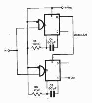
Fig. 6.3. Digital bandpass filter constructed from a single 4098/4528 package. If the input pulse interval lies between the periods of the monostables, the output follows the input. Otherwise the output is permanently held either high or low. With the values given only frequencies lying between 1kHz and 2kHz will be transmitted
