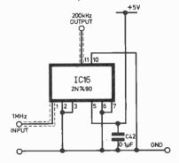
Fig. 13 (b). Circuit diagram of the divider to give the 200kHz calibration signal from the 1MHz available on the main board. Both circuits are mounted on the one board
