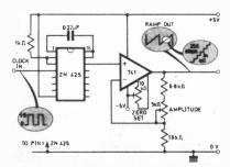
Fig. 1. Linear ramp generator
