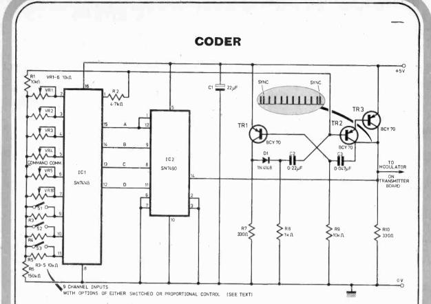
Fig. 2. Circuit diagram of the Coder
