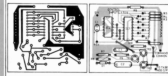
Fig. 3. Printed circuit master and component layout details for the Coder (full size)
