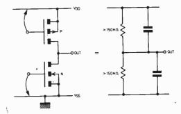
Fig. 6.5. Complementary pair with both devices biased "off" forms a disabled output which is floating with respect to the supply rails
