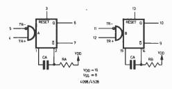
Fig. 6.1. Pin connections for the 4098 or 4528 dual retriggerable monostable.  $R_{\rm A}$  and  $R_{\rm B}$  can be between  $5 {\rm k}\Omega$  and  $10 {\rm M}\Omega$ .  $C_{\rm A}$  and  $C_{\rm B}$  can be any value, and the period is given approximately by T=RC seconds
