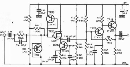
Fig. 13 (a). Circuit diagram of the high impedance buffer
