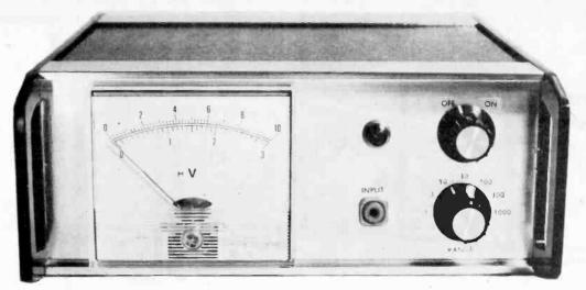
Front of the Audio Millivoltmeter showing the range switch and input socket
