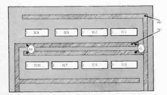
Fig. 6. Layout of the components on the dual-in-line board
