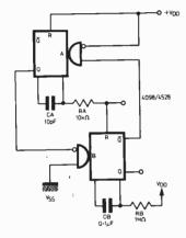
Fig. 6.4. Multivibrator using two monostables. With the values given the "on" and "off" times are about 0.1 secs and 0.1 μsecs respectively
