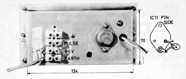
Rear view of the Milometer showing the three-way terminal block, regulator i.c. and measurements. Note that C4 is wired directly to the i.c. as shown on the right
