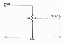
Fig. 20. A potentiometer across the input of the Digital Frequency Meter reduces the loading effects
