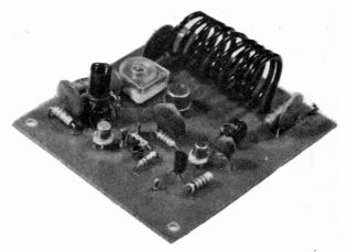
Transmitter Board. Note the crystal is not shown in position
