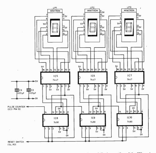
Fig. 3. Circuit diagram of the display counter, decoder and display section of the Milometer
