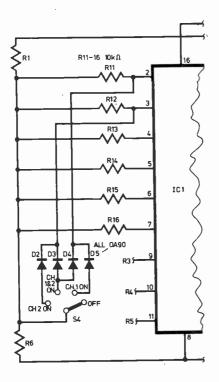
Fig. 4. Method of diode gating to give simultaneous control of channels in addition to individual control
