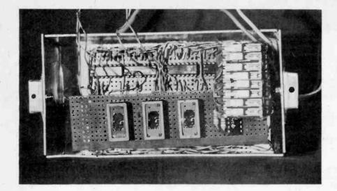
Interior view of the Milometer showing the dual-inline switches and general layout of display board
