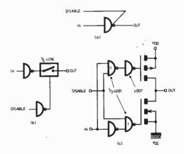
Fig. 6.6. (a) Symbol for an inverter with a three-state output. (b) Three-state output using a bilateral switch. The extra inverter is to make the disable input active when "high". (c) Three-state output using the connections to the gates of the individual MOSFETs, made available in the 4007
