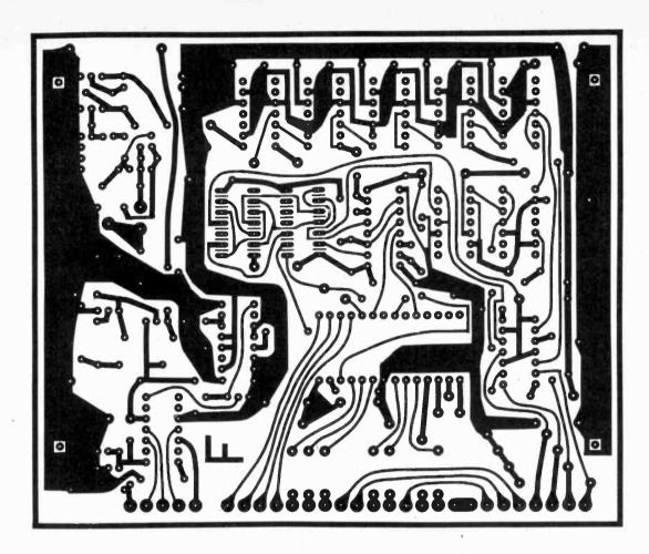
Fig. 8. Full size printed circuit master of the main board as viewed from the copper side
