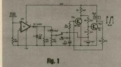
D ESIGNED to operate a bedside lamp (using the remaining contacts RLA2), the circuit shown in Fig. 1 uses an interesting form of bistable, which unlike conventional types, does not need a steep rising edge to trigger it. Despite its limitations (it will not operate at more than 0.8Hz), it does away with the need for a Schmitt trigger.
