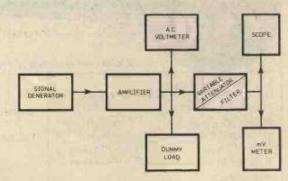
Fig. 1. Arrangement used by the author to measure t.h.d. The filter removes the fundamental enabling the distortion products (including noise) to be measured
