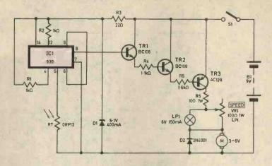
first NAND gate is at "1" and the other input automatically becomes "1". An output of "0" is produced and this is fed into the second NAND gate producing an output of "1" which is fed into the base of TR1. This transistor switches TR2 to the logic level and then TR3 starts to conduct, producing a current which drives the motor and lamp LP1. Due to greater current consumption of the motor the more the bulb light
