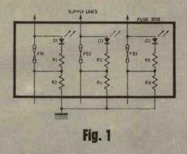
**F** uses have a nasty habit of blowing at very inconvenient times, such as when its dark, cold or wet. This simple arrangement can provide an easy-to-see monitor as to the state of the fuses and thus can save a lot of bother.
