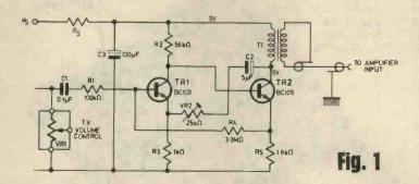
After amplification. the signal is presented to the external amplifier through T1, the primary of which is the collector load of TR2. Transformer T1 must be a mains
