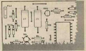
Fig. 18. The positions for the additional components required on PCB2 (Fig. 5) are shown here. Note that the rear right-hand pad on the underside was not used in the car clock but is now connected to the outside right pad on the display p.c.b. PCB4. The START I.e.d. becomes the ALARM ENABLE I.e.d. R61 is in series with S11. (Alarm circuit is given in Fig. 3)
