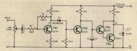
Fig. 3. Circuit diagram of the mono version of the peak level indicator
