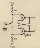
Fig. 3.7. Switch debouncer using an R-S latch. The resistors may be any large value. Alternatively NOR gates may be used, with the resistors going to  $V_{\rm SS}$  and the switch to  $V_{\rm DD}$
