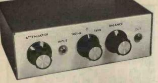
at the position which gives the lowest indication on an oscilloscope or millivolt meter connected to the output of the filter. VR3 should be set at its midway setting during this operation.
