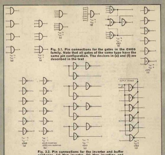
Fig. 3.2. Pin connections for the inverter and buffer packages. (a) Hex inverter. (b) Hex inverting and non-inverting buffers or level converters. (c) Quad true/complement buffer. (d) Strobed hex inverter buffer. Pin 4 is the three-state output disable, and pin 12 is the output inhibit
