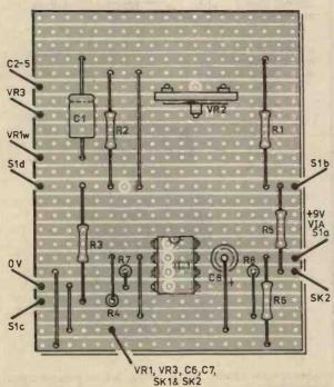
Fig. 4. Veroboard details and component layout
