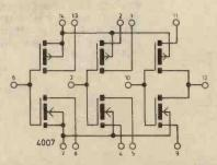
Fig. 3.3. Connection diagram for the 4007 dual complementary pair and inverter. The diode protection networks are not shown
