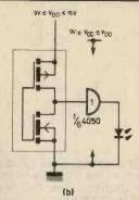
Fig. 3.4. Driving circuits. The block represents a standard CMOS output. Resistor R, where necessary, limits the current through the l.e.d. (a) Simple transistor driver. (b) Use of 4050 as a driver and level-converter;  $V_{CC}$  is chosen to give the correct current through the l.e.d. (c) Driver using 4049 with supplies of above 7 volts. (d) To provide sufficient current for the l.e.d. at very low voltages both a buffer and a transistor may be required
