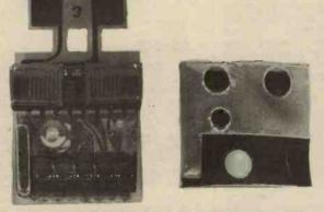
The assembled watch module and copper surround. It is essential that all components are closely seated on the p.c.b. and all lead ends cropped short or the copper screen will not fit. It is expected that the screen will be omitted from future kits with circuit modification.
