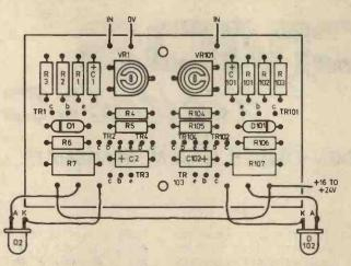
Fig. 4(a). Layout of the components of the printed circuit board. For a mono version the board can be split down the middle and only half used
