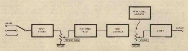
Fig. 1. Block diagram of a typical audio preamplifier showing the suggested connection point for peak level indicator
