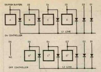
Fig. 17. Example of connecting BCD switches to Controller for on/off switching. A box indicates as BCD switch with series diodes to lines LA to LD
