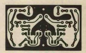
Fig. 4(b). Full size printed circuit master of the peak level indicator
