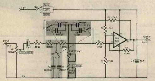
Fig. 3. Full circuit diagram of the filter
