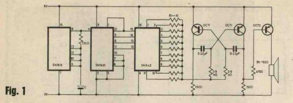
T HE circuit in Fig. 1 is similar to the Autotone published in P.E. about a year and a half ago. The ring counter has been replaced by a triple i.c. system. An SN7413, R1 and C1 forms an oscillator which then drives a 7490 decade counter. This then feeds a 7442 decoder which sequentially public resistors R1-10 to earth. The
