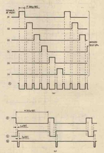
Fig. 14(a). Signals at points marked on Latch circuit (b) Signals at IC5/6 and (c) enlarged view of these at (8), (9), (10)
