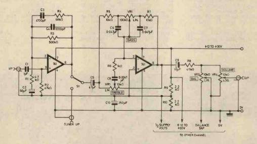
M ost i.c. pre-amp circuits specify the use of specialised, and sometimes hard to obtain, integrated circuits. There is no reason, however, why the ubiquitous (and cheap!) 741 should not be employed in this application. Fig. 1 shows a circuit using these which does not require the normal dual power supply and will in fact operate satisfactorily on any single unregulated supply in the range 12 to 30V.
