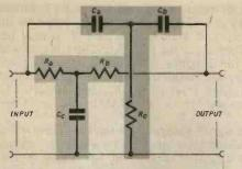
Fig 2. The basic "Twin-Tee" notch filter
