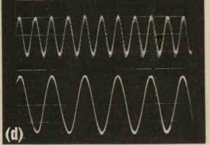
Fig. 5. Typical oscilloscope traces obtained using the filter: (a) balance control set roughly correct; (b) balance control adjusted to align tops of waveforms; (c) signal generator frequency then adjusted to align bottoms of waveforms; (d) distortion (predominantly second harmonic) and residual noise with fundamental notched out. The sinewave input is at 1kHz and the measured level of distortion is 1%
