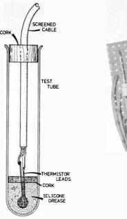
Fig. 2. Construction of the sensor using a small test tube and some silicone grease
