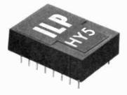
The HYS is a complete mono hybrid preamplifier, ideally suited for both mono and stereo applications. Internally the device consists of two high quality amplifiers—the first contains frequency equalisation and gain correction, while the second caters for tone control and balance.
