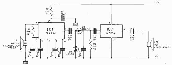
Fig. 3. Circuit diagram of the basic ultrasonic receiver
