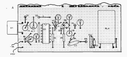
Fig. 6. Component layout and Veroboard cutting details for the receiver of Fig. 4. Note the mounting of the transducer and the extra board space which may be used for power supply or other items
