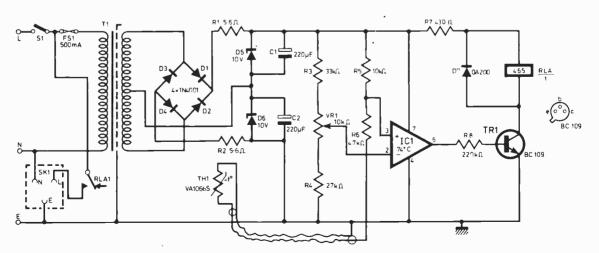
Fig. 1. Complete circuit diagram of the Electronic Thermostat
