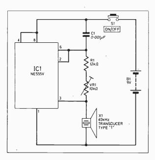
Fig. 2. The transmitter circuit
