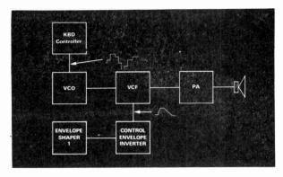
Fig. 5.2. Diagram showing the patching arrangement to use the voltage controlled filter as a Waa-Waa
