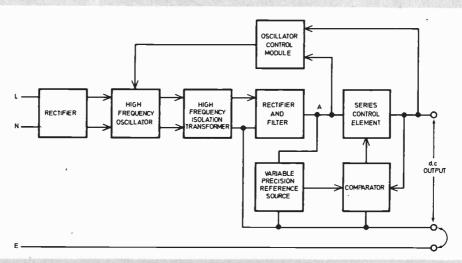
Fig. 5. Power unit incorporating both linear and switching principles
