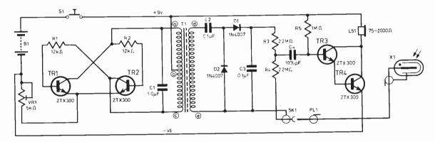
Fig. 2. Circuit diagram of the power supply, GM tube and amplifier
