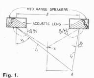
The plates are made from wood or plastic, are arranged vertically, and are of varying length. When the listener stands at position X the plates have virtually no influence or effect on the sound waves from the mid-range speakers. But as the listener moves away from the position X towards one side, the nearest speaker's plates both diminish the level of sound to that ear and delay it in dependence on how close and thus how far off the axis of the plates he is standing.
