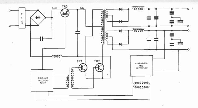
Fig. 2. Conventional inverter circuit diagram
