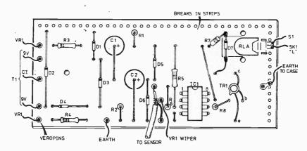
Fig. 3. Layout of components on the Veroboard. The diode D7 is connected directly across the coil contacts of the relay
