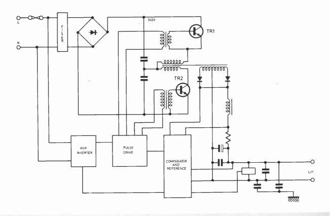
Fig. 3. Variable output inverters
