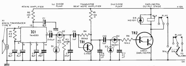
Fig. 4. An alarm receiver circuit including a latching relay at the output
