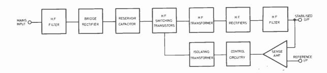
Fig. 1. Block diagram of switching regulator
