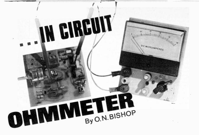
HIS instrument can be used for measuring the resistance of a component without the need to disconnect it from its circuit. This facility can save a lot of time in circuit checking, particularly when working with miniature components on circuit boards. It may also be used in the normal manner for checking unconnected components.
