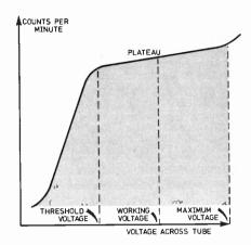
Fig. 1. The characteristic curve of a GM tube
