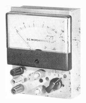
from base to collector, but not in reverse or from collector to emitter. A pnp transistor will conduct only from emitter or collector to base. When connected for conduction, the meter will indicate some resistance less than f.s.d. When otherwise connected, a greater resistance (usually greater than f.s.d.) will be shown.
