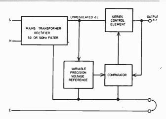
Fig. 4. Linear regulator block diagram
