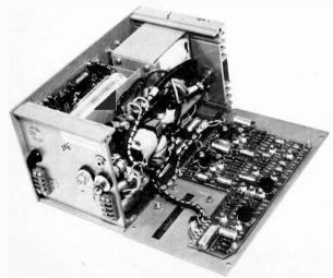
Also the circuit can give very large swings of output voltage and input voltage without unlocking. The main disadvantages are that since it operates near the audio range it can, under light load conditions, break into the audio range. Furthermore, as the ripple frequency is variable, it is more difficult to filter out.
