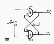
Fig. 2. Eliminating switch bounce using half an SN7400N
