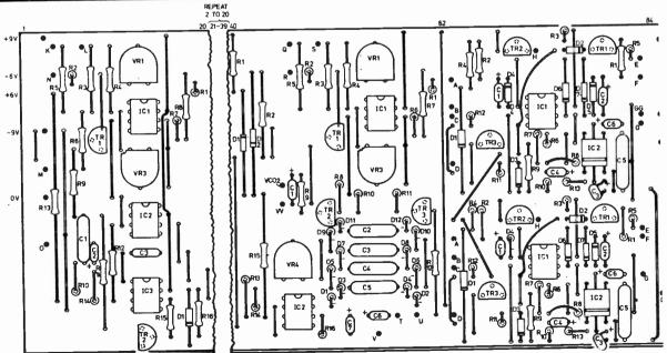
Fig. 2.8. Layout of the components on the Veroboard. Note that two identical VCO's are required side by side on the panel, only one is shown. Both Envelope Shapers are shown in full. Letters next to Veropins are for wiring to the front panel and correspond with those on the circuit diagrams
