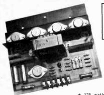
All output power ratings ±0.5dB; Output impedance 8-15.ohms; THD at full power 2% typically 1%. Input sensitivity 60mV into 10kΩ: Fre-quency response 20Hz-20kHz quency response 20Hz-20kHz ± 2dB; Hum and noise better than
