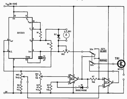
Fig. 4. A variation of the diode thermometer designed to give both control and indication functions
