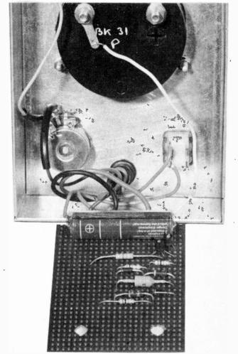
View inside the prototype Dwell Meter showing the simple interwiring between the meter, board and external vehicle circuit
