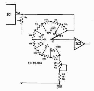
Fig. 6. A modification of Fig. 1 which gives an expanded scale covering 10°C but switchable to start at any of a number of selected temperatures
