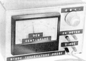
Obviously there are many applications including normal workshop testing as when a transistor is running hot. The indicator can show if it is too hot or still within its range. The blind controller can be used to maintain an item of equipment at a given pre-set temperature using a heating element.
