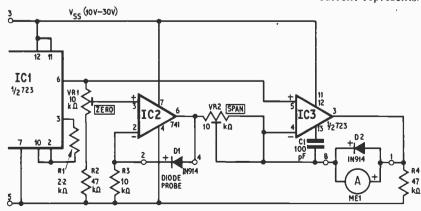
Fig. 1. Circuit diagram of the heart of the indicating diode thermometer showing the use of integrated circuits to provide sophisticated circuit functions in a very simple manner
