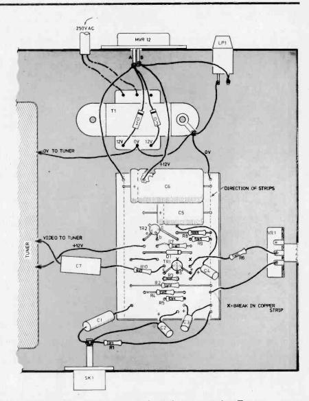
Fig. 4.4. Component layout of sync separator, video inverter and power supply. Tuner unit is adjacent
