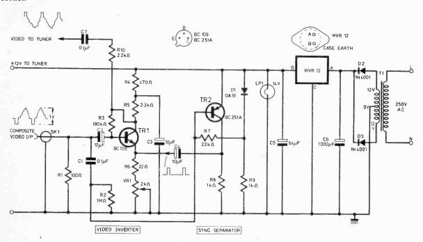
Fig. 4.1. Circuit diagram of sync separator and video inverter
