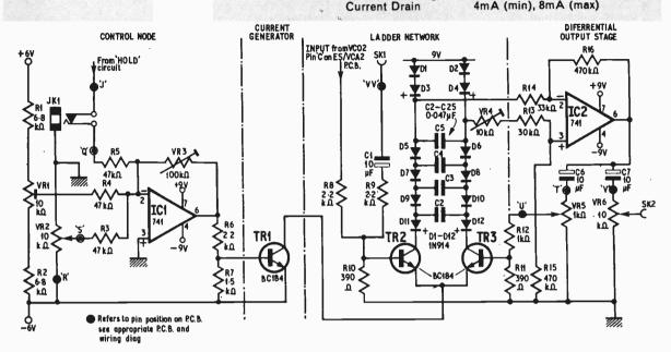
Fig. 2.4. Complete circuit diagram of the Voltage Controlled Low-pass Filter
