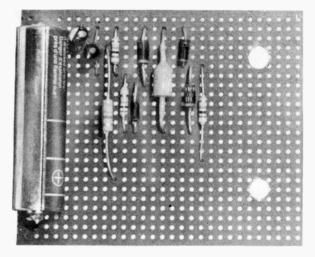
Component layout on the Veroboard used in the prototype. Note the use of the alkaline cell power source
