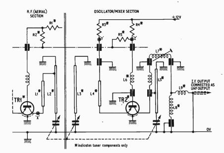
Fig. 4.2. Showing modifications and connections to typical u.h.f. tuner. All straight line inductances are lecher bars
