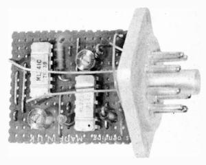
An assembled circuit board mounted on its octal plug carrier and with the cover removed
