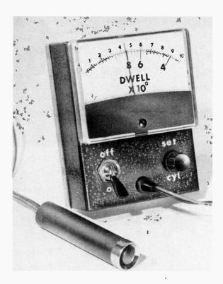
The Dwell Meter together with the starter switch push unit. Of course, they are not connected electrically, one going to the starter solenoid whilst the other goes to the points
