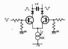
Fig. 2.5. Simplified circuit diagram of the lower section of the VCF showing how the a.c. signal is superimposed on the ladder current
