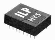
The HY5 is a complete mono hybrid preamplifler, ideally suited for both mono and stereo applications. Internally the device consists of two high quality amplifiers—the first contains frequency equalisation and gain correction, while the second caters for tone control and barcott.
