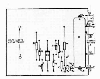
Fig. 3. Component layout and Veroboard cut details for the dwell meter
