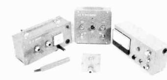
The devices vary in characteristic. Type 308 sensor has a very long warm up time of between 5 and 10 minutes and is, therefore, better suited for use where only occasional turning off or on is required. However, the device is very sensitive to carbon monoxide and smoke.
