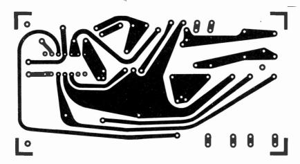
Fig. 2. Printed circuit master for the power supply
