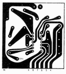
Fig. 8.5. Master p.c.b. copper layout for the decoder board
